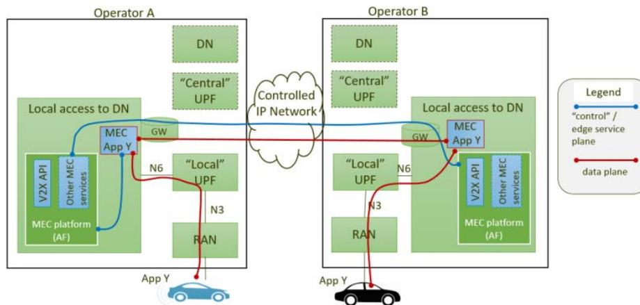
**Figure 5.1.1-2: Illustration of a MEC federation reference scenario where both MNOs have MEC platforms and a MEC application Y ("MEC App Y") is instantiated (Multiple OEM vehicle use case) (source: 5GAA document XW2\_200048, May 2020) [i.5]**
