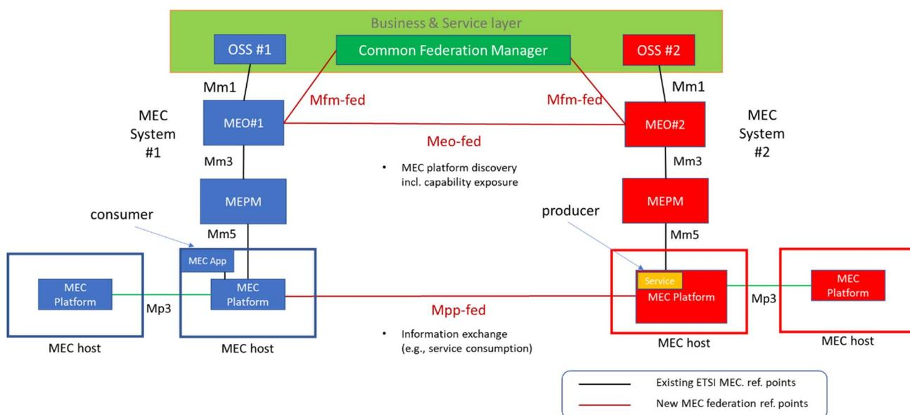
**Figure 6.5.2-5: All proposed MEC federation reference points assuming a single Federation Manager, the scope of which is the whole MEC federation**
