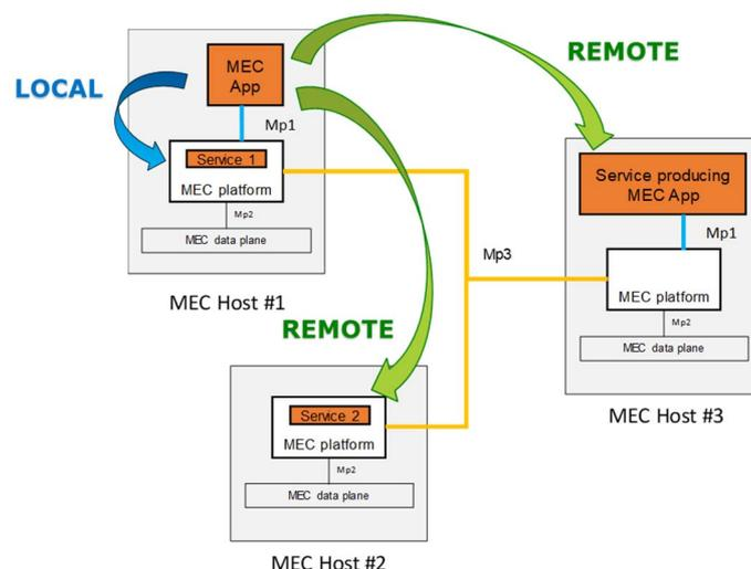
**Figure 6.5.1-1: Edge service consumption options within a single MEC system**
