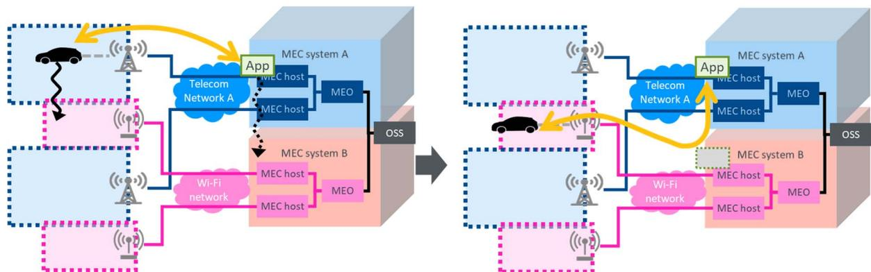
Figure 5.4.1-4: Abstract level of behaviour in case of MEC service remote consumption
