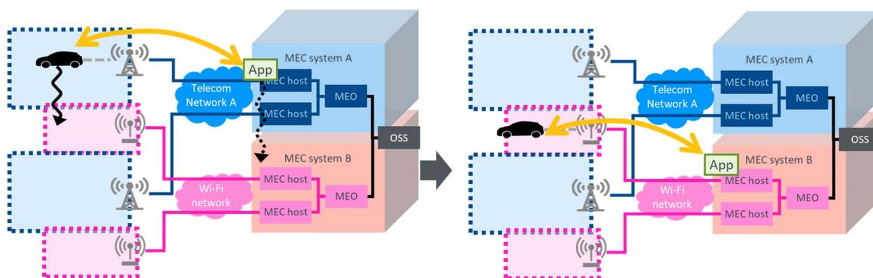
Figure 5.4.1-1: Abstract level of behaviour in case of two MEC systems in one MNO environment
