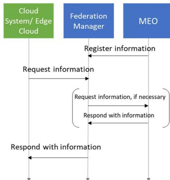
**Figure 6.7.2-1: Exposure of MEC service information to a Cloud System/Edge Cloud via Federation Manager**
