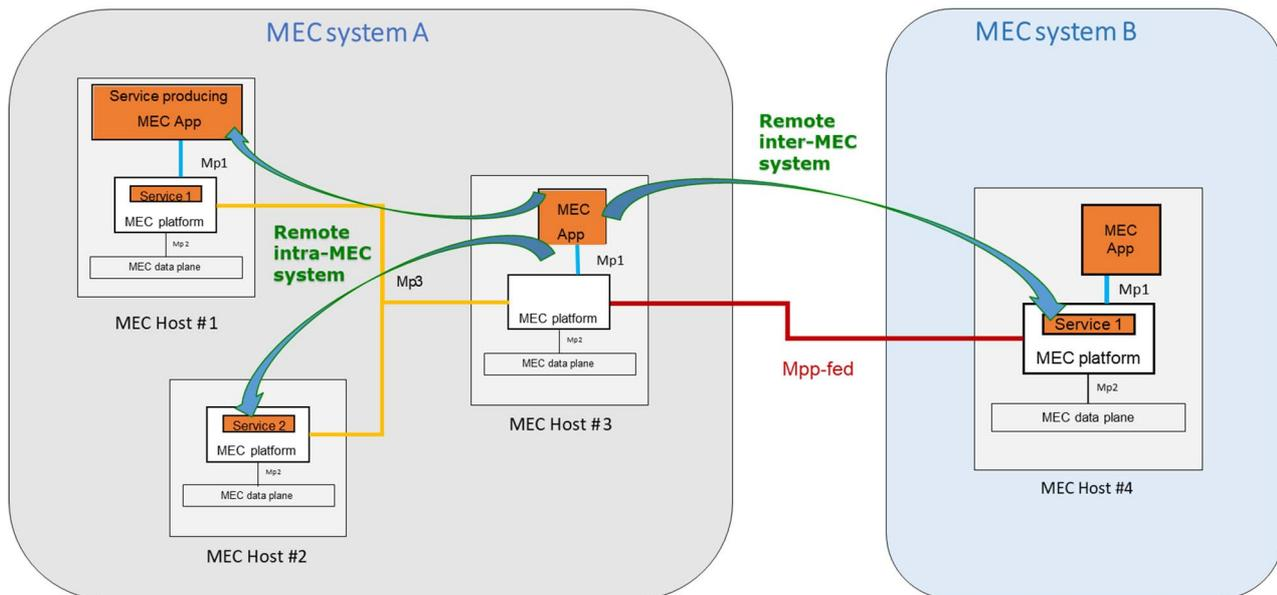
**Figure 6.5.2-1: MEC federation scenario enabling edge service consumption across MEC systems**
