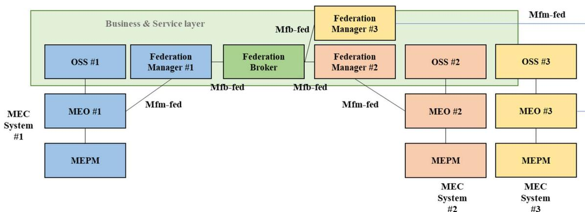
NOTE: In this implementation variant, a single Federation Broker for the whole MEC federation is considered.
