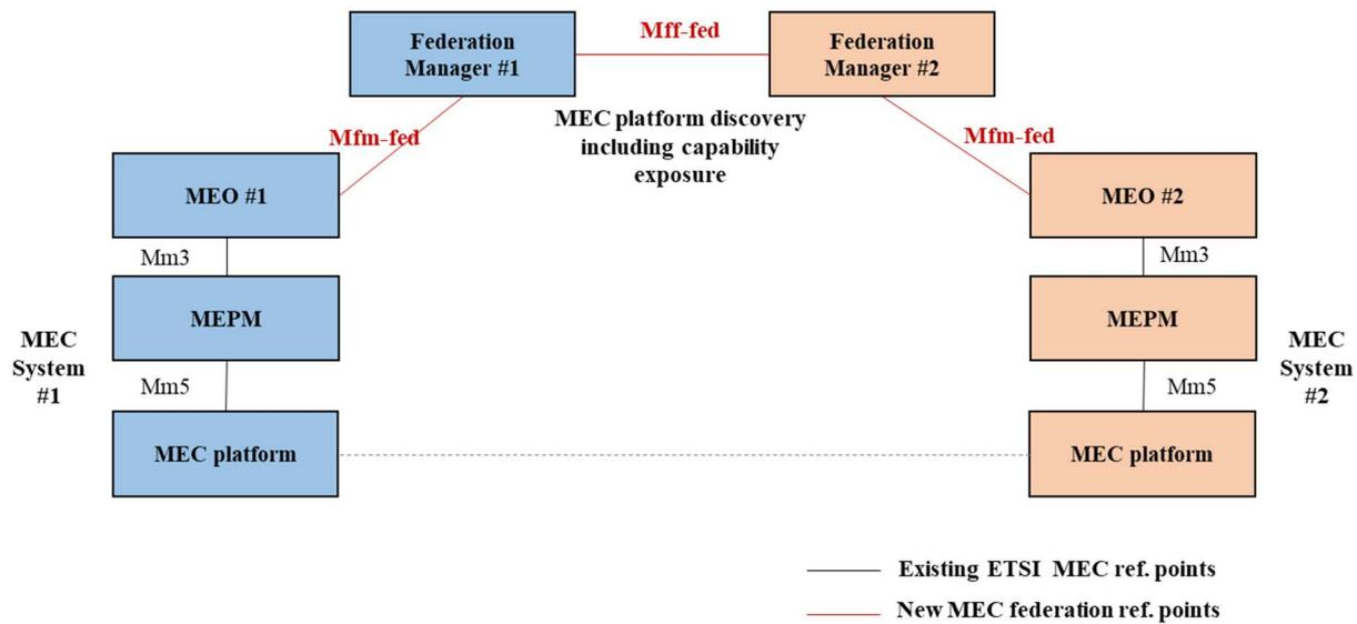
**Figure 6.4.3-1: Inter-MEC platform discovery by using the Federation Manager modules**
