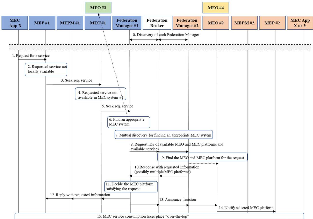
**Figure 6.5.3-1: Sequence diagram explaining the involved signalling via MEC federation management reference points to establish inter-MEC system communication for the needs of service consumption**
