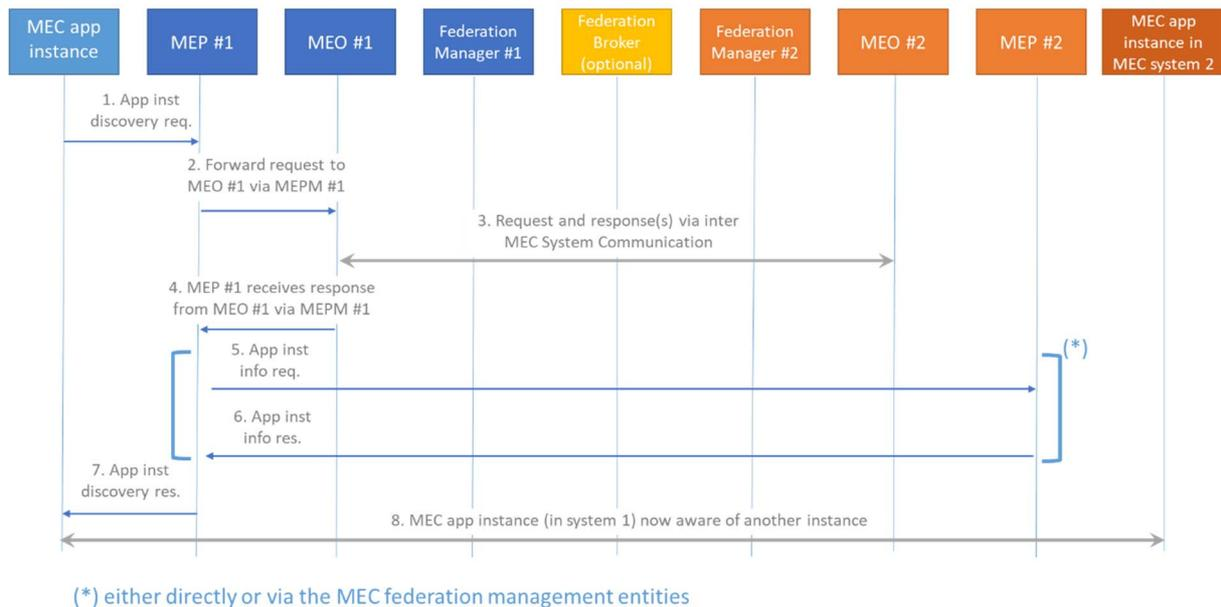
**Figure 6.8.2-1: Sequence diagram explaining MEC application instance discovery**
