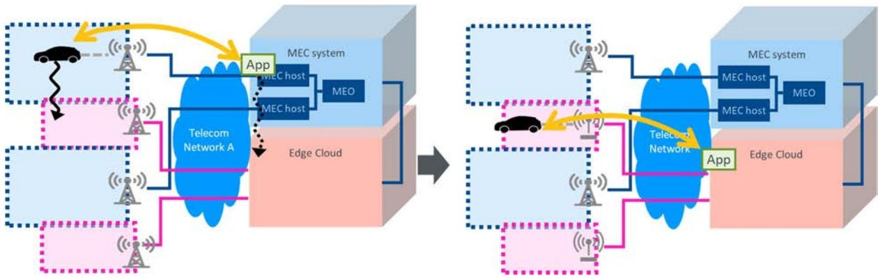
Figure 5.4.1-2: Abstract level of behaviour in case of MEC system and Edge Cloud in one MNO environment
