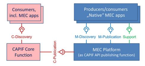
Figure 4.3.2-1: Loosely-coupled deployment of CAPIF and MEC
