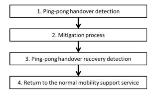
Figure 5.2.2-1: High level information flow to mitigate ping-pong handover effects
