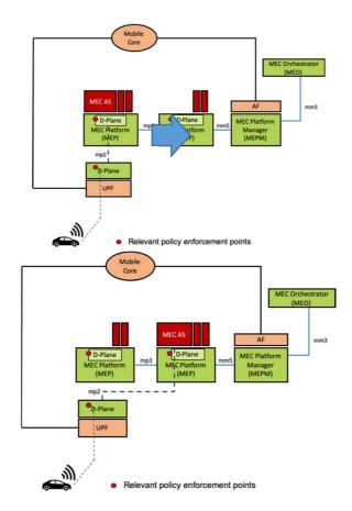
Figure 5.1.3.3-1: Traffic steering between UPF and MEC AS
