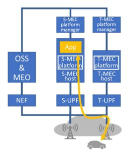
Figure 5.1.2.2-1: Function blocks in intra-operator case
