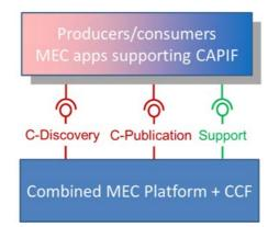
Figure 4.3.3-1: Fully-integrated hybrid deployment of CAPIF and MEC
