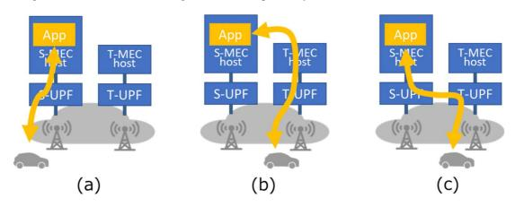
Figure 5.1.1.2-2: Mobility support, where the target MEC host cannot be used
