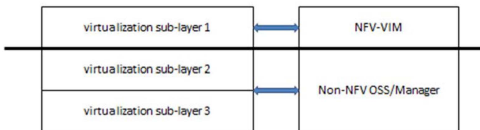
Figure 2: Example sub-layering of nested virtualization technologies [i.7]
