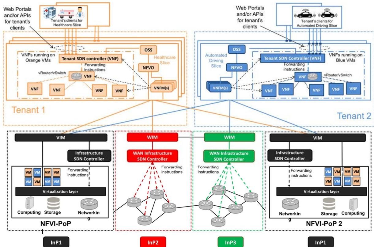
**Figure 4.5-1: Network slicing deployment applying NFV concepts to achieve isolation (Figure 4.3-1 in ETSI GR NFV-EVE 012 [i.16])**
