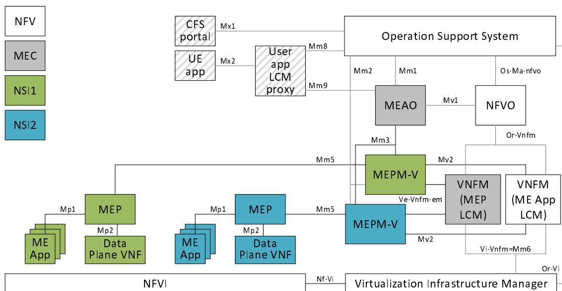
Figure 5.5.1-1: Example of MEC in NFV with dedicated instances of MEC components in distinct NSIs
