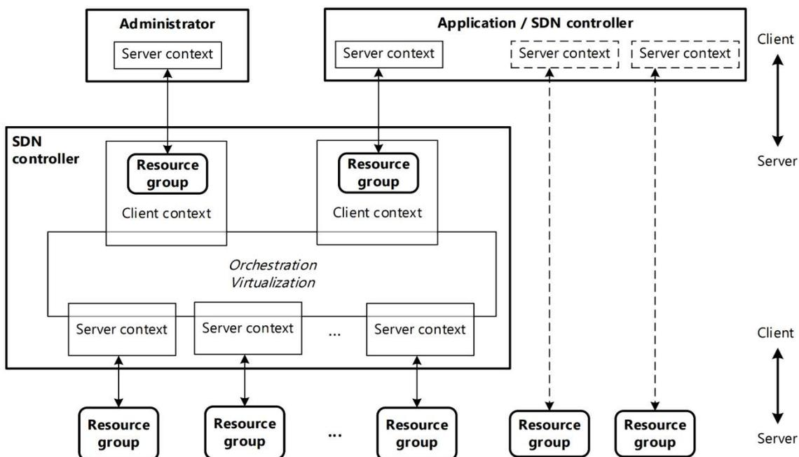
**Figure 4.3-1: Core concepts of the SDN architecture**
