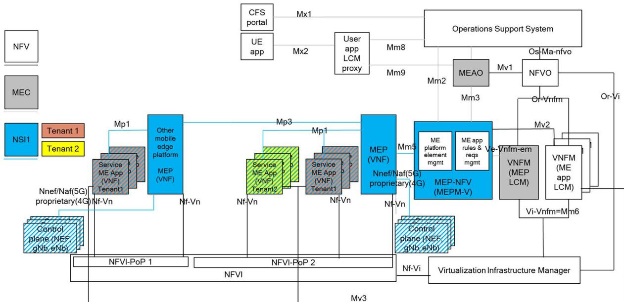
**Figure 5.6.1-1: Example of multiple MEC applications belonging to different tenants deployed in a single NSI**
