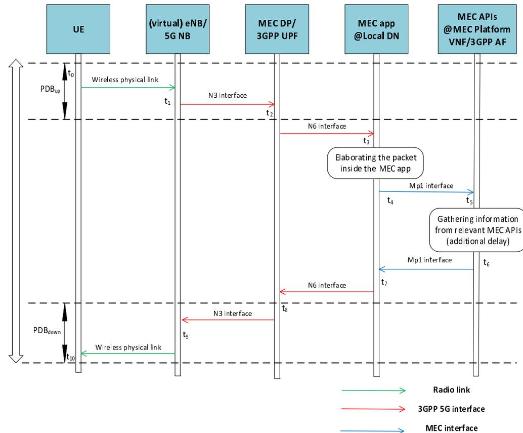
**Figure 5.7.1-1: Message sequence chart illustrating the various latency components during the direct communication between a client app (at the UE) and a MEC application (at the edge), which consumes in its turn some MEC services running on the MEP**
