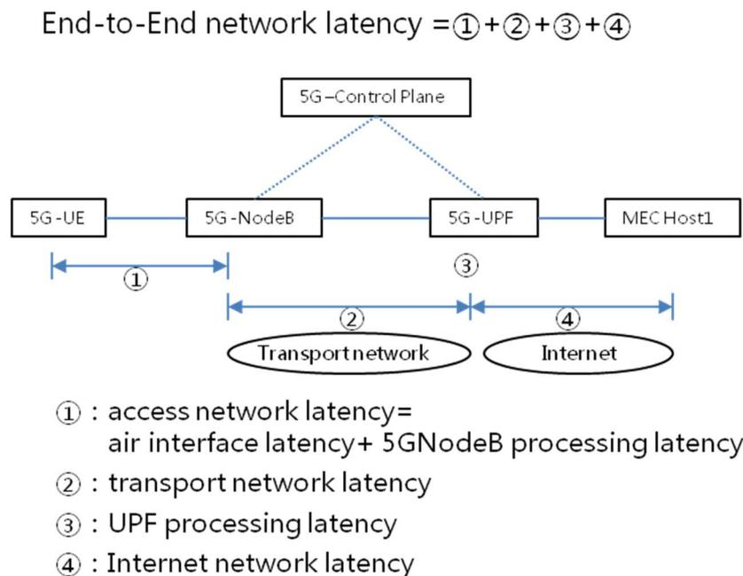
**Figure 5.4.1-1: End-to-end latency of a Network Slice Instance with MEC**
