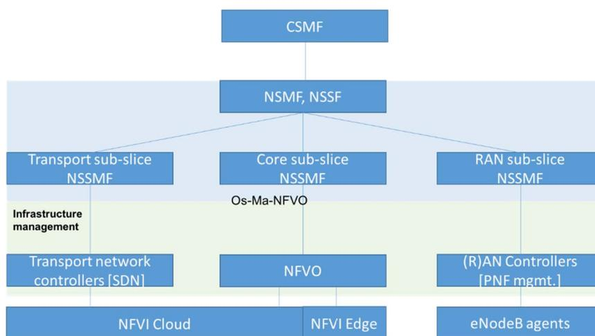
Figure 5.3.1-1: Network Slice architecture including MEC
