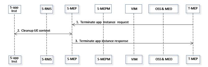
Figure 5.4.2-1: A message flow for terminating application instance of shared service triggered by T-MEP
