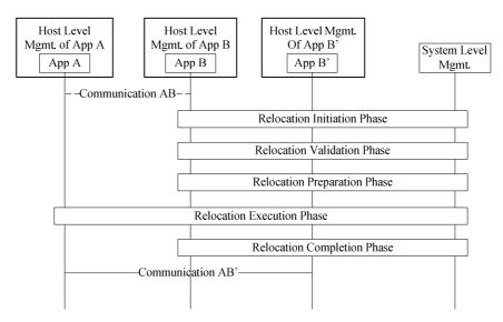
Figure 5.5.3-1: High-level information flow for relocation procedure
