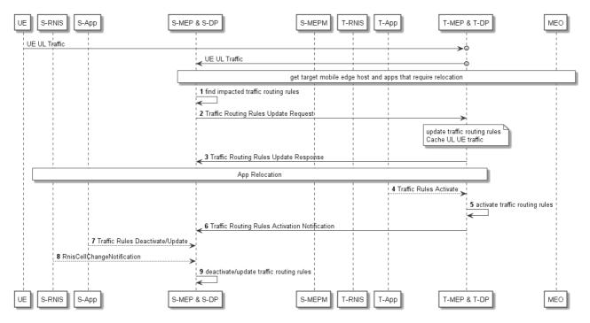
Figure 6.2.6.3-1: Information flow for updating traffic routing rules triggered by UE UL Traffic
