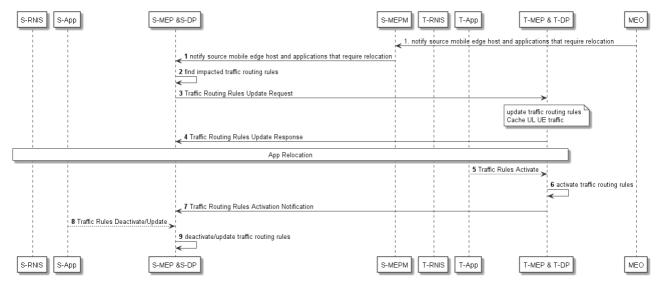
Figure 6.2.6.4-1: Information flow for updating traffic routing rules triggered by MEO
