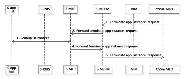
Figure 5.4.2-2: A message flow for terminating a shared service of application instance triggered by MEO
