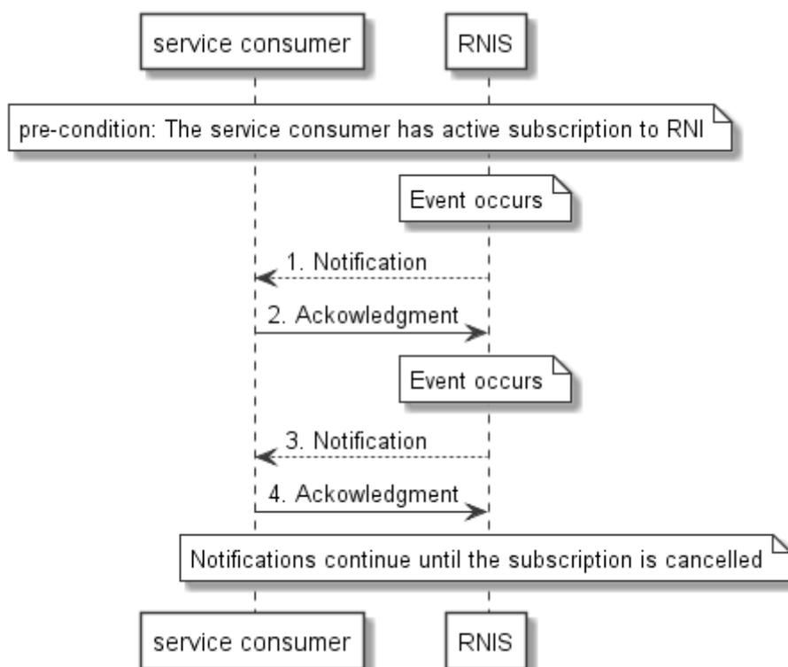
Figure 8.5.5-6: Flow of subscribing to the RNI event notifications tests
