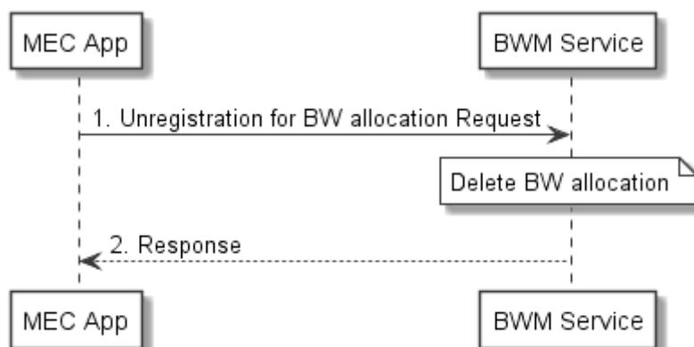
Figure 8.8.2-1: Flow of MEC Application unregistering BW allocation from BWMS
