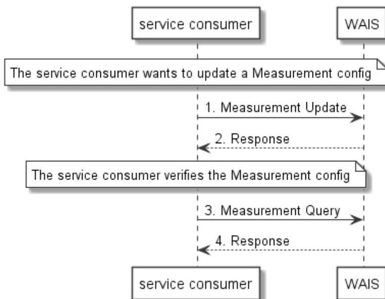
Figure 8.6.4-2: Flow of service consumer updating a WLAN measurement configuration
