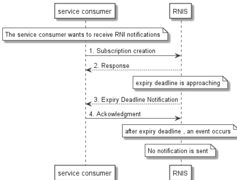
Figure 8.5.5-4: Flow of Receiving notification on expiry of RNI event subscription tests
