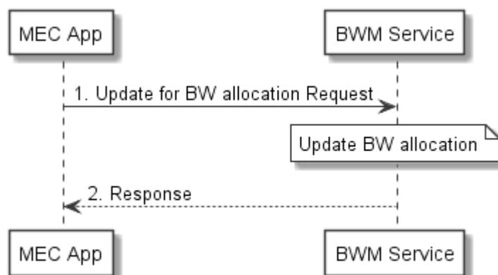
Figure 8.8.3-1: Flow of MEC application updating its requested bandwidth requirements on BWMS
