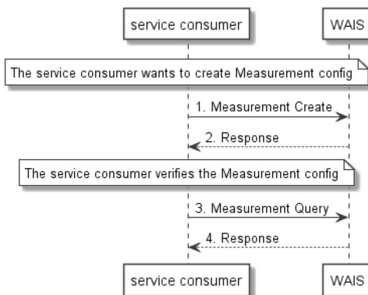
Figure 8.6.4-1: Flow of service consumer creating a WLAN measurement configuration
