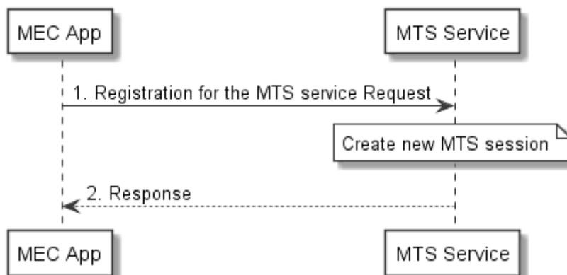
Figure 8.8.7-1: Flow of MEC Application registration to the MTS service
