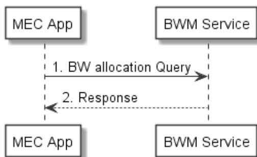
Figure 8.8.5-1: Flow of MEC Application getting its configured bandwidth allocation from BWMS
