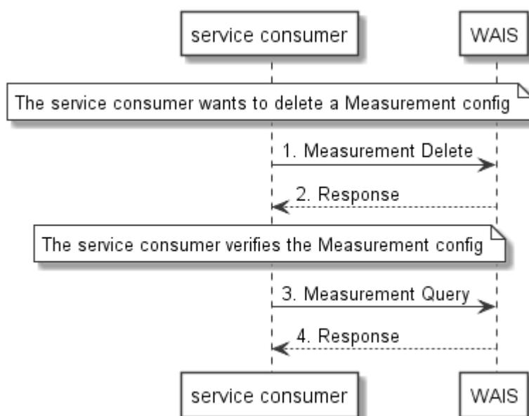
Figure 8.6.4-3: Flow of deletion of a Measurement Configuration
