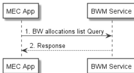
Figure 8.8.4-1: Flow of MEC Application getting bandwidth allocation list from BWMS
