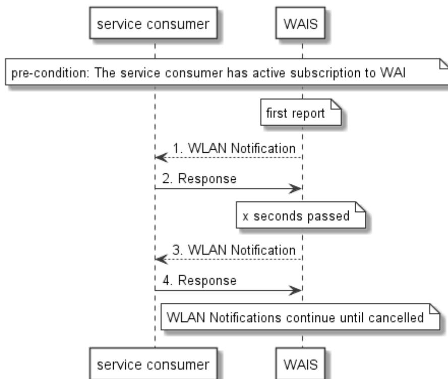
Figure 8.6.3-7: Flow of subscribing to the WLAN event notifications tests, once every x seconds
