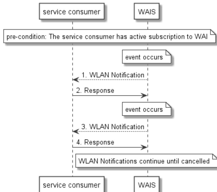
Figure 8.6.3-6: Flow of subscribing to the WLAN event notifications tests
