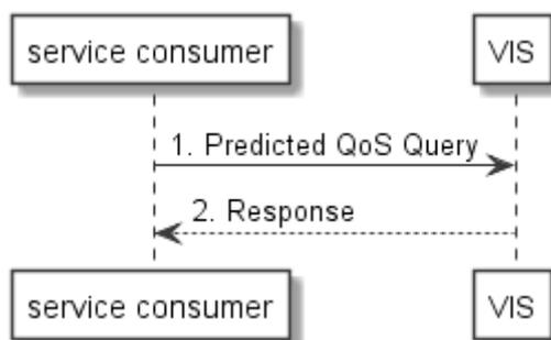
Figure 8.7.4-1: Flow of a V2X application requesting the predicted QoS of a UE with potential routes
