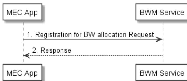
Figure 8.8.1-1: Flow of MEC Application registration to BWMS
