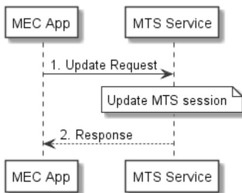
Figure 8.8.9-1: Flow of MEC application updating its requested requirements on the MTS service
