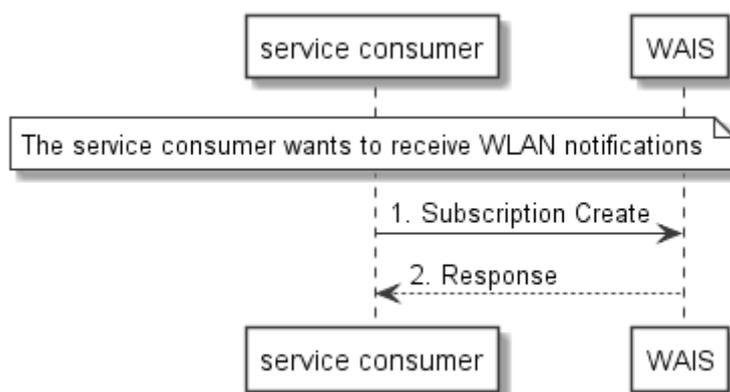
Figure 8.6.3-1: Flow of subscribing to the WLAN event notifications tests
