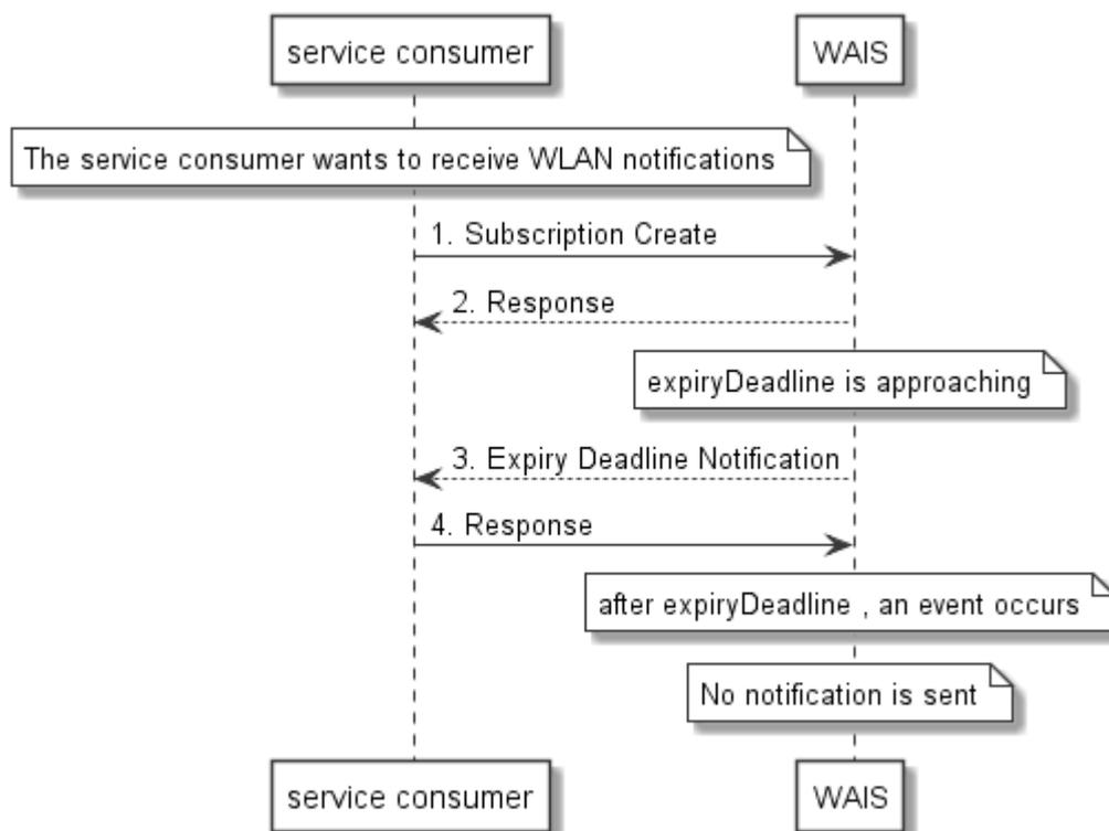
Figure 8.6.3-4: Flow of Receiving notification on expiry of WLAN event subscription tests
