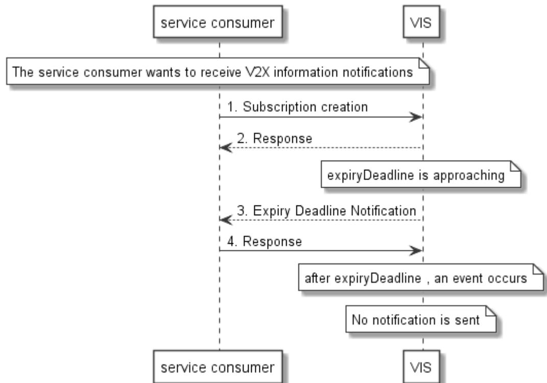
Figure 8.7.5-4: Flow of VIS sending a notification on expiry of the subscription
