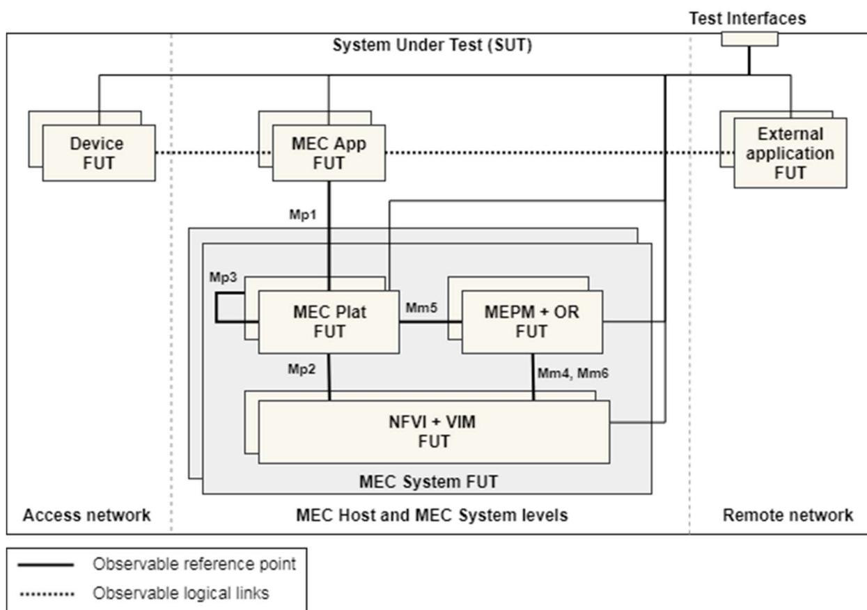
**Figure 4.4.3-1: EXAMPLE: A specific SUT architecture for a specific interoperability test may contain Device FUT, MEC App FUT and MEC System FUT**
