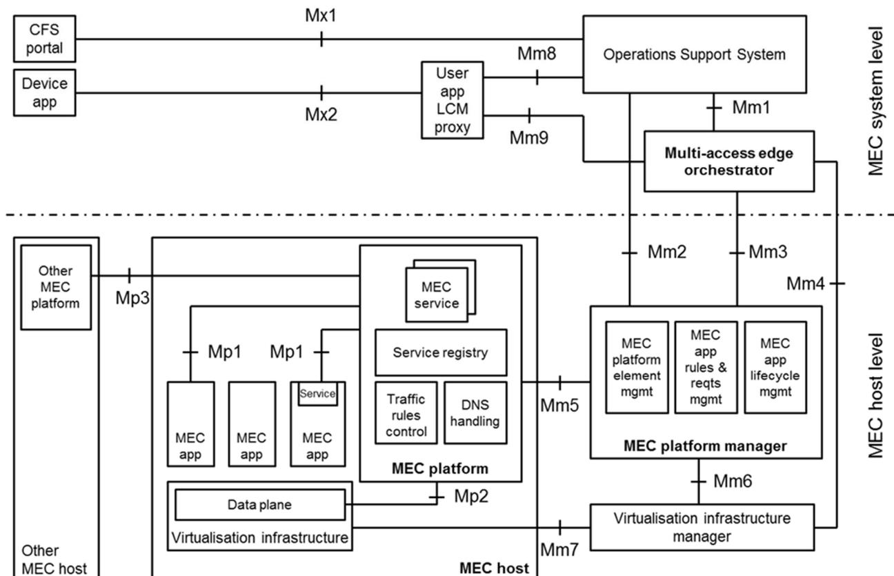
Figure 4.3.2.1.1-1: Multi-access edge system reference architecture
