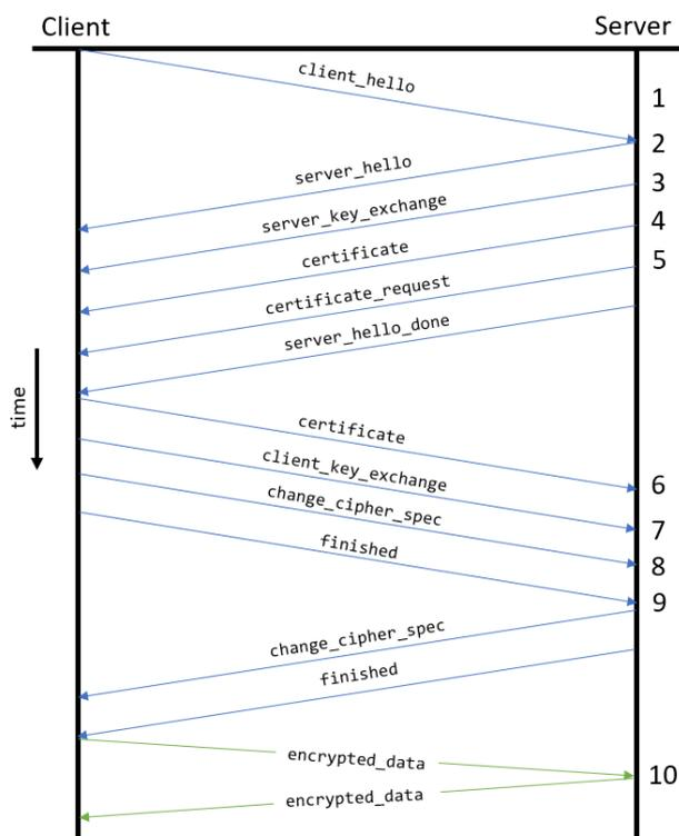
Figure 2: SSL/TLS Handshake Protocol
