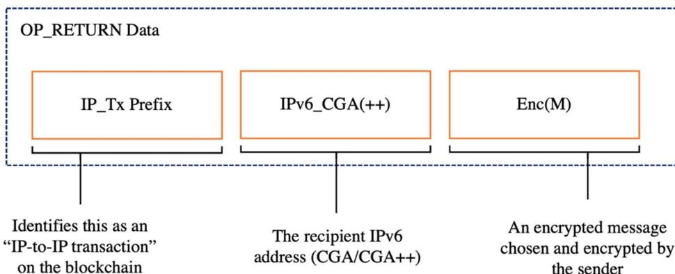
**Figure 9: The on-chain data components of an example on-chain messaging scheme**
