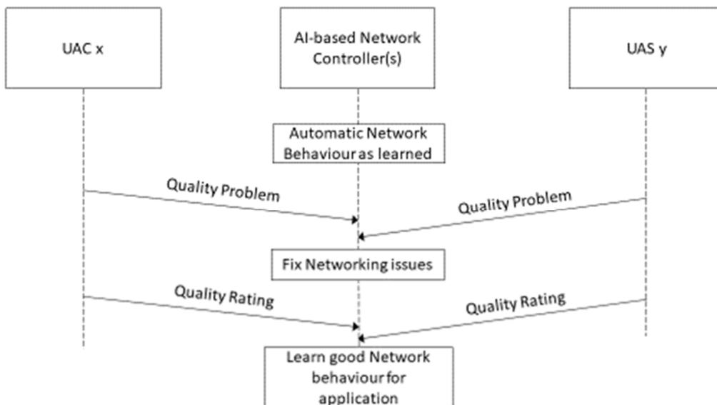
NOTE: This is an example using reactive network controller mechanism based on AI.
