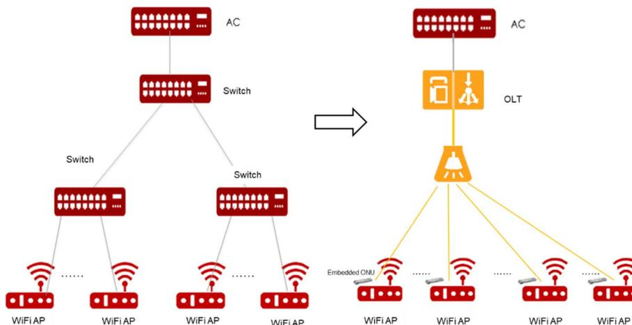
Figure 33: Extend PON to AP Ethernet Uplink
