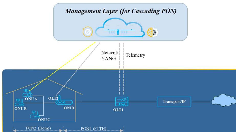
**Figure 43: Example of enhanced traffic monitoring and network control for cascading PON**
