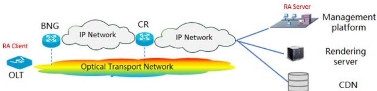
Figure 48: Remote Attestation Network Architecture
