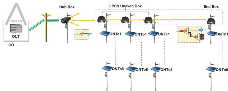
**Figure 26: PON based connection for smart light poles**
