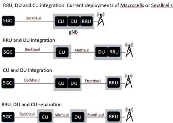
**Figure 31: Different options for gNB modules integration/separation**
