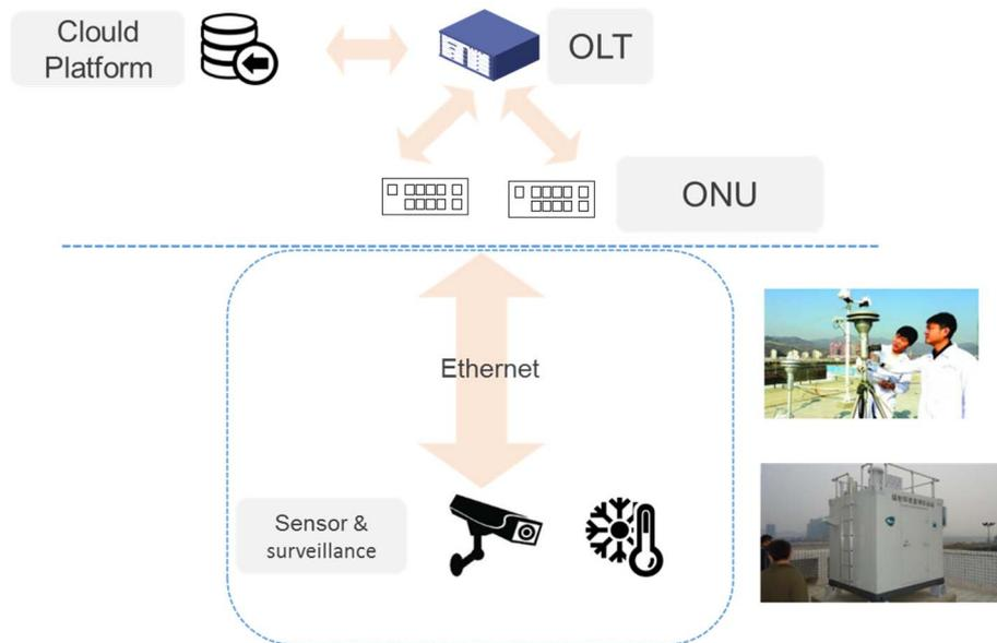
**Figure 25: PON for sensor & surveillance network overview**
