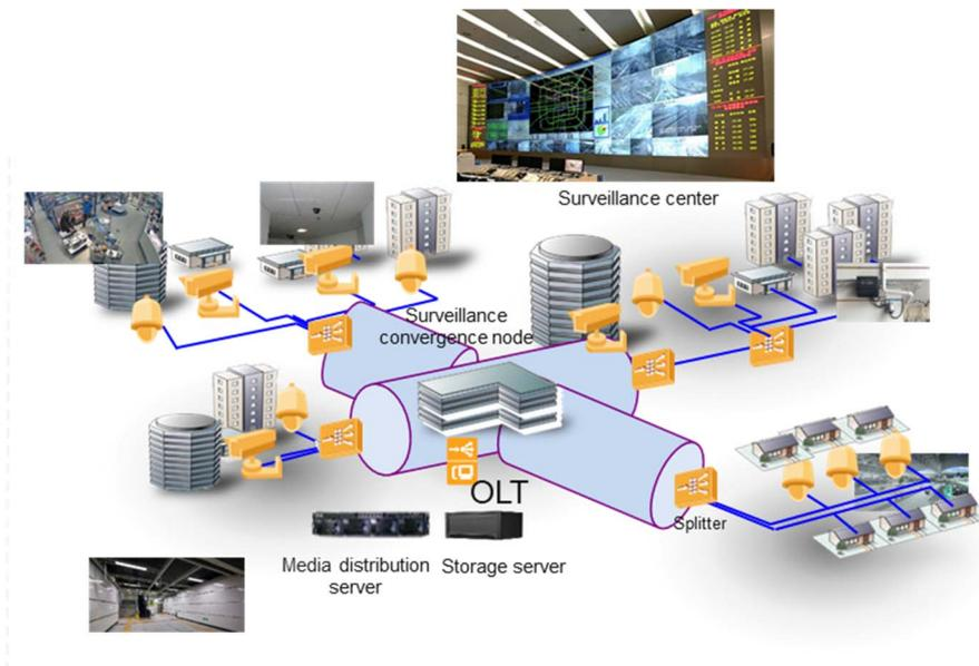
**Figure 34: Extend PON to Video surveillance backhaul**
