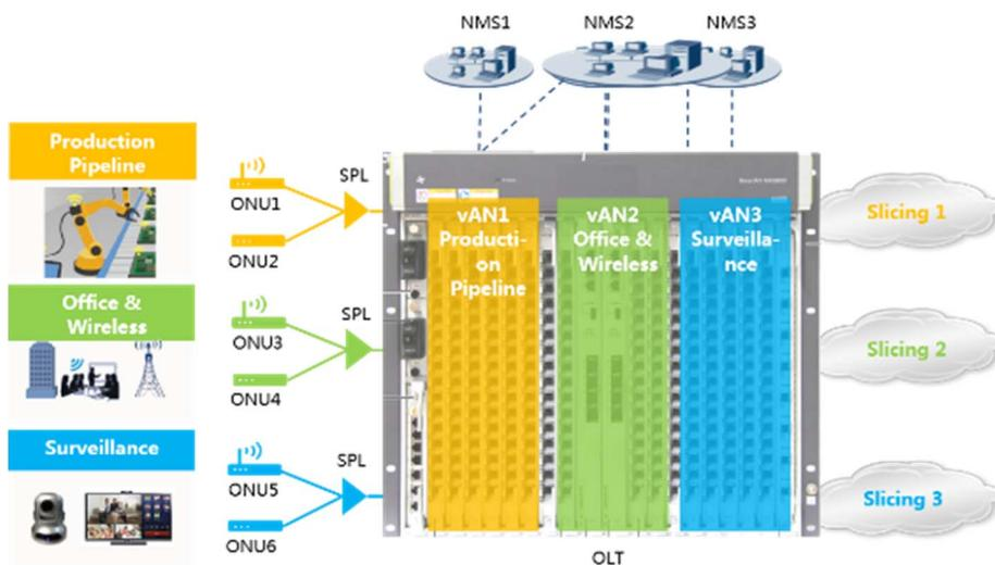
**Figure 22: Schematic diagram of PON slice**
