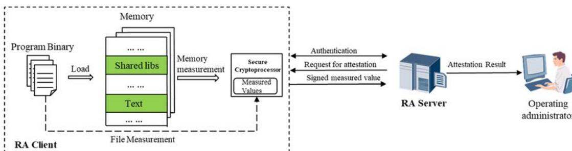
Figure 50: DIM With Remote Attestation
