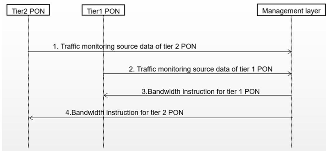
**Figure 44: Operational flow of bandwidth dynamic adjustment in Intelligent Access Network**
