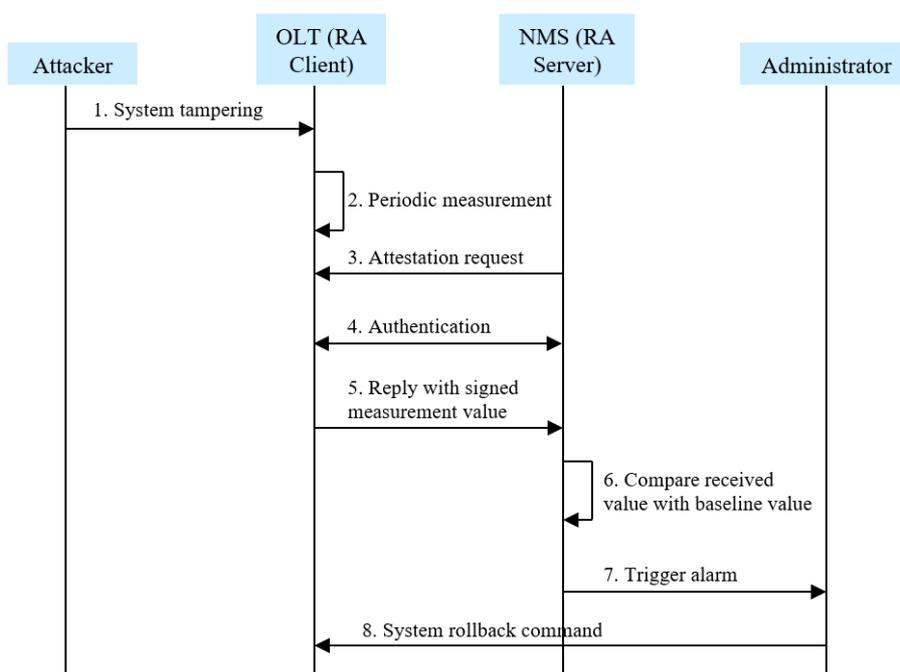
**Figure 51: Operational flow of remote attestation**
