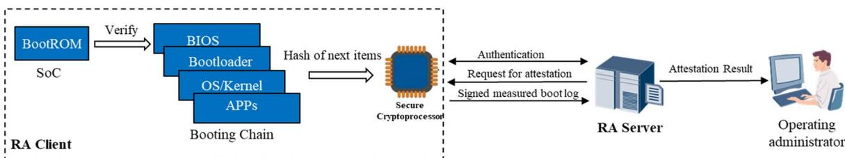
Figure 49: Measured Boot with Remote Attestation
