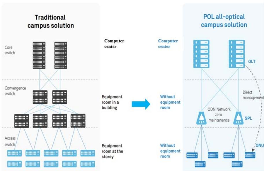
Figure 15: The POL all-optical solution compared with traditional campus solution
