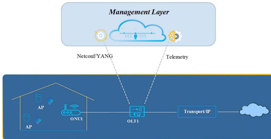
**Figure 42: Example of enhanced traffic monitoring and network control for intelligent access network**
