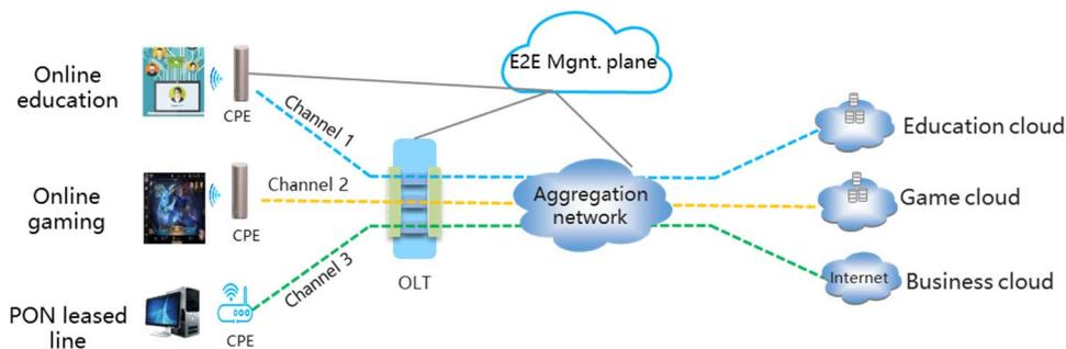
**Figure 35: Multiple applications carrying on the network**
