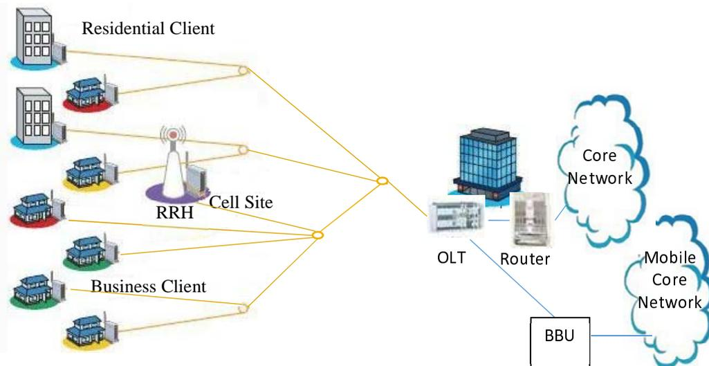
**Figure 27: Overview of the multiple access aggregation over PON**
