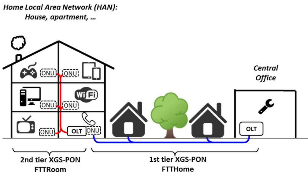
Figure 14: Cascaded PONs with new on-premises devices
