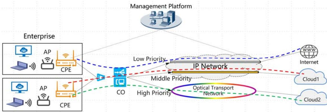
**Figure 10: SME private line service identification and distribution of application traffic**
