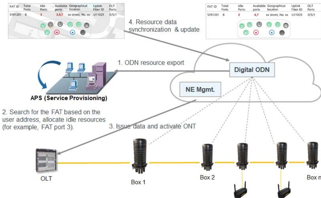
**Figure 53: Digitalized ODN enables automatic service provisioning and accurate resource management**
