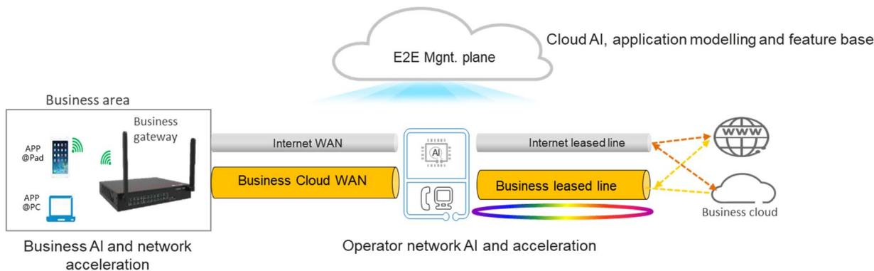
**Figure 40: Network architecture of the PON leased line**
