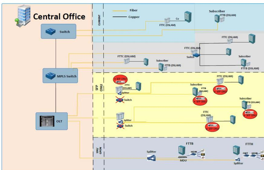
Figure 32: Extend PON to DSLAM Ethernet Uplink
