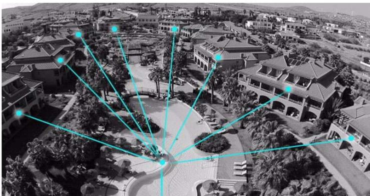
**Figure 20: Overall PON architecture in the resort**
