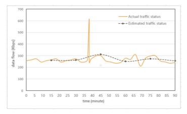
Figure 41: Example diagram of micro traffic burst
