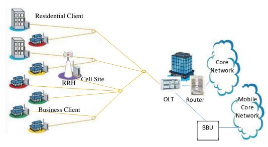
Figure 27: Overview of the multiple access aggregation over PON
