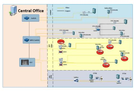
Figure 32: Extend PON to DSLAM Ethernet Uplink
