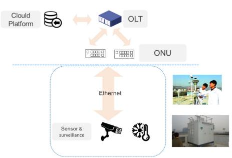
Figure 25: PON for sensor & surveillance network overview
