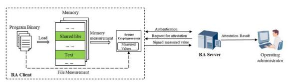
Figure 50: DIM With Remote Attestation
