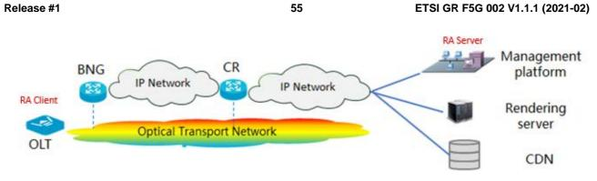
Figure 48: Remote Attestation Network Architecture
