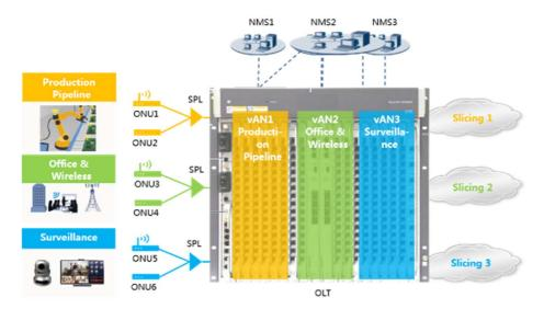
Figure 22: Schematic diagram of PON slice
