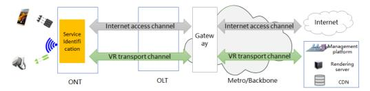
Figure 4: Cloud VR transport in independent channel
