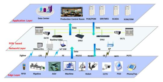
Figure 21: PON based industrial network solution overview
