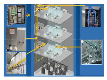
Figure 24: PON for office network, the internal networking in the office park with internet/intranet, telephone, fax services
