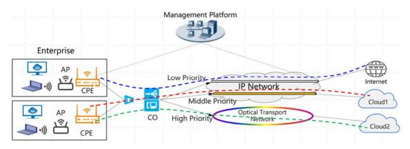
Figure 10: SME private line service identification and distribution of application traffic
