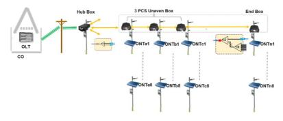
Figure 26: PON based connection for smart light poles
