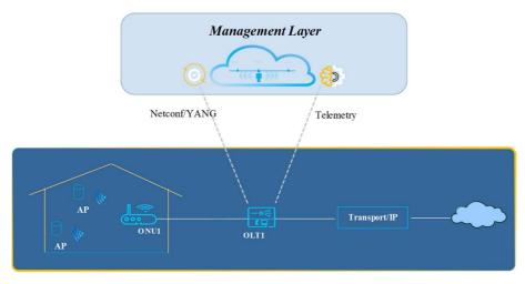
Figure 42: Example of enhanced traffic monitoring and network control for intelligent access network
