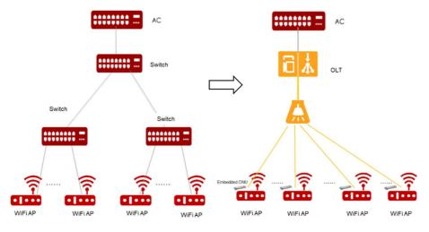
Figure 33: Extend PON to AP Ethernet Uplink
