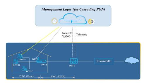
Figure 43: Example of enhanced traffic monitoring and network control for cascading PON
