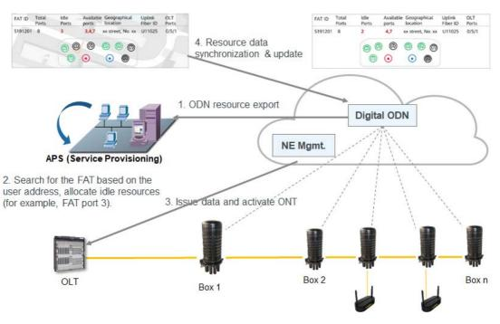
Figure 53: Digitalized ODN enables automatic service provisioning and accurate resource management
