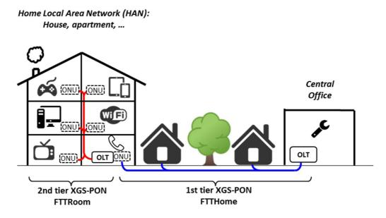
Figure 14: Cascaded PONs with new on-premises devices
