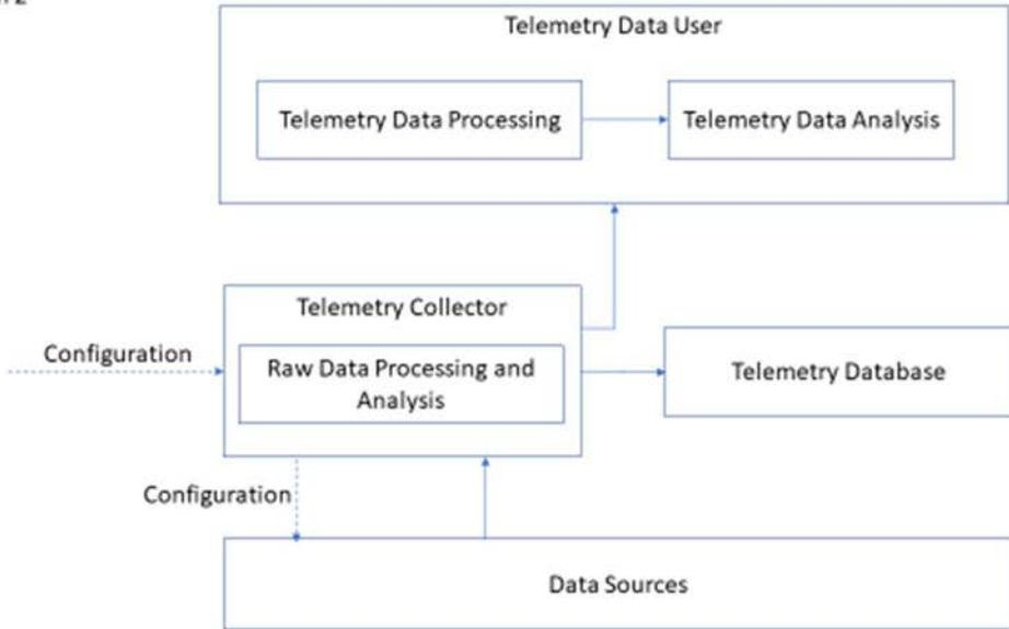
**Figure 5-3b: Components of Network Telemetry framework, Push Option**
