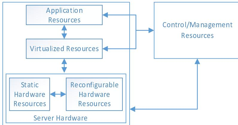
**Figure 5-4: Various infrastructure resources that generate telemetry data**
