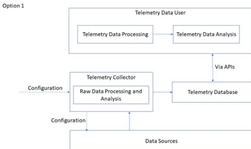
**Figure 5-3a: Components of Network Telemetry framework, API option**
