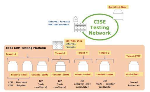
Figure 8: A conceptual scheme of the ETSI CDM testing platform
