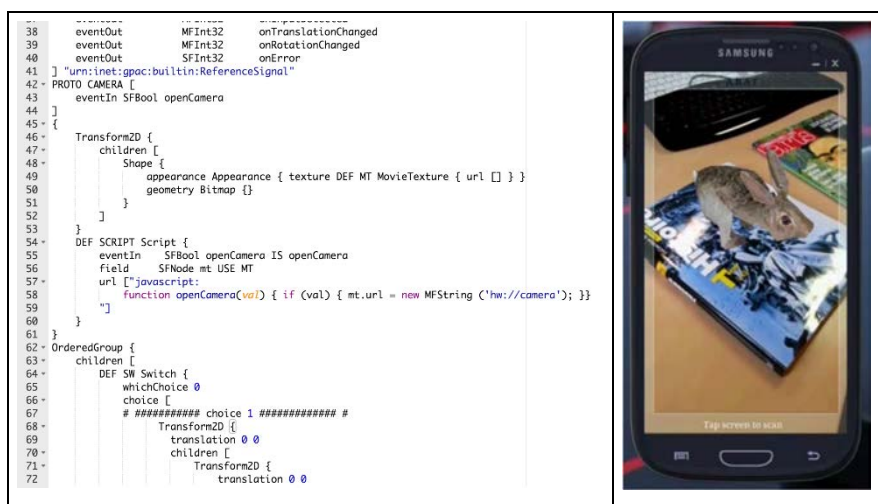
Figure 3: A fragment from the ARAF file for APM use-cases illustrated on right side of the figure
