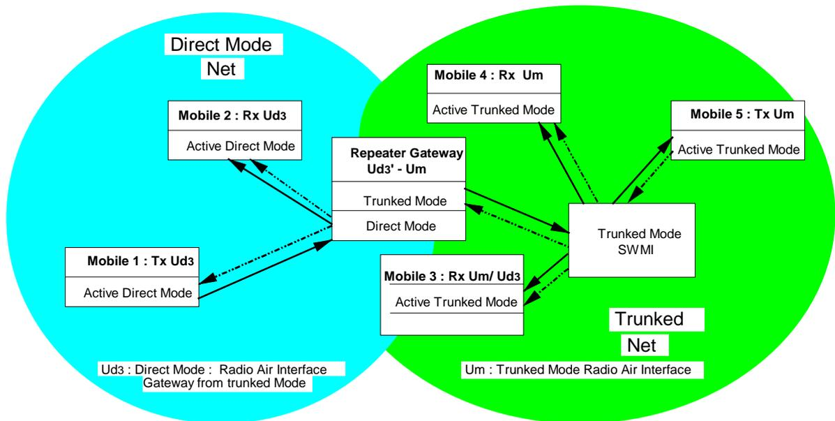
**Figure 11: Functional network configuration showing Direct Mode Repeater/Gateway air interface**
