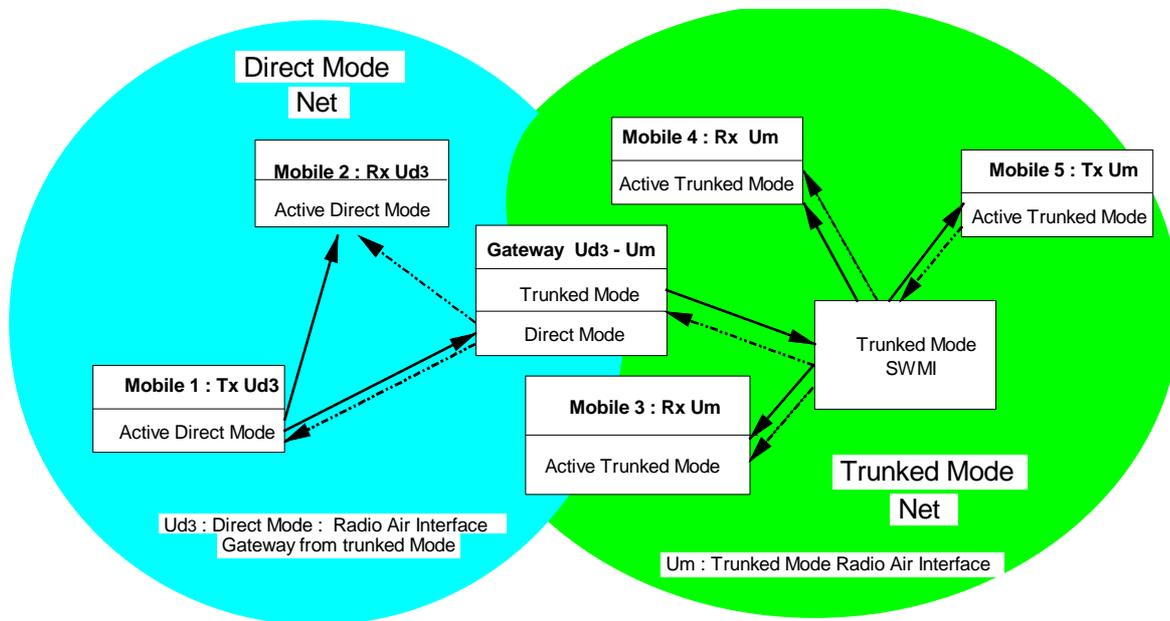
**Figure 10: Functional network configuration showing Direct Mode Gateway air Interface**
