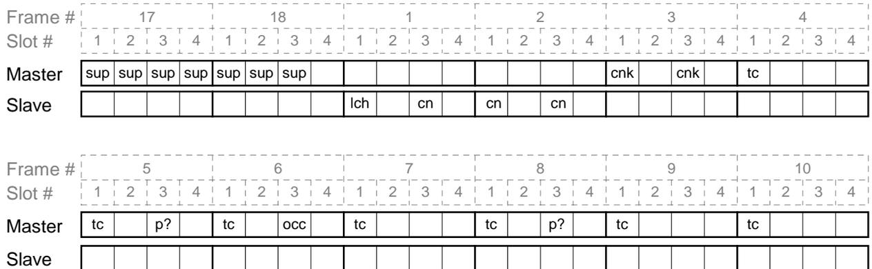
**Figure 15: Call sequence for set-up with presence check**
