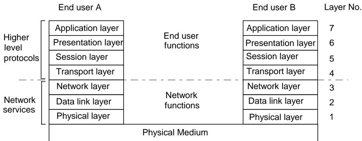
**Figure 12: OSI reference model for communication architectures**
