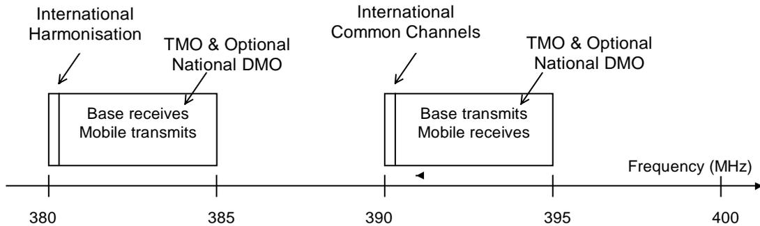
**Figure 1: Proposal for spectrum lay-out in the 380 MHz to 400 MHz frequency range**
