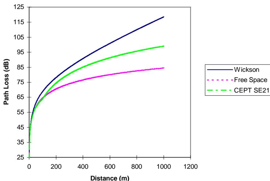
**Figure C.3: Calculated path loss for the three propagation models  $h_1 = 10$  m,  $h_2 = 30$  m**
