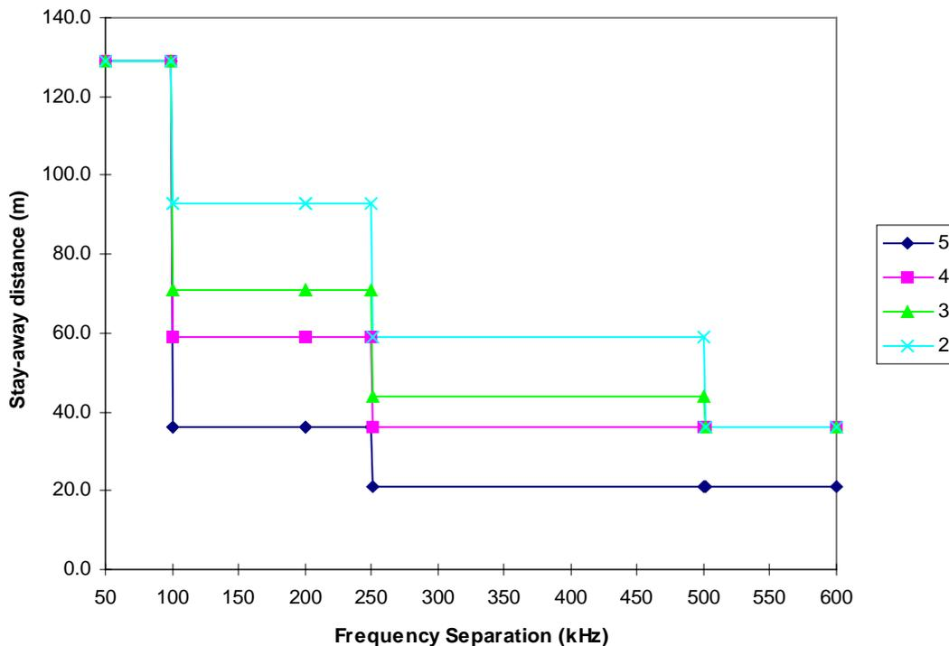
**Figure 26: Stay away distance to ensure effects of blocking Tx or wideband Tx interferer are at negligible level for different interfering Tx power classes.**
