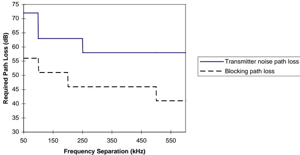
Figure 24: Path loss to reduce blocking Tx or wideband Tx interferer to negligible level
