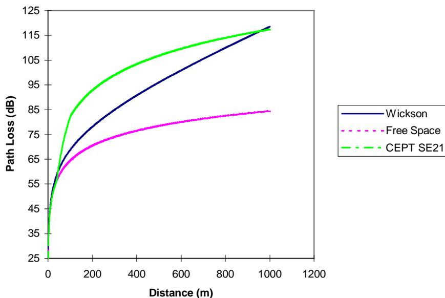
**Figure C.2: Calculated path loss for the three propagation models  $h_1 = 1,5$  m,  $h_2 = 30$  m**
