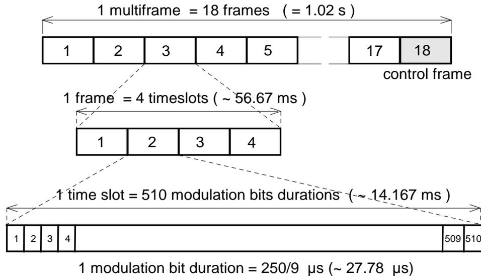
Figure E.1: DM framing structure
