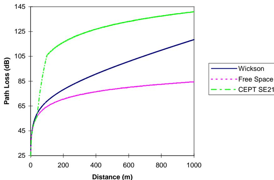
**Figure C.1: Calculated path loss for the three propagation models  $h_1=1.5\text{m}$ ,  $h_2=2\text{m}$**
