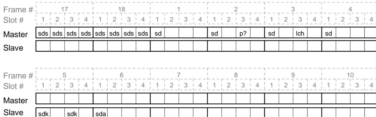
Figure F.2: Call sequence for SDS - for acknowledgement with data
