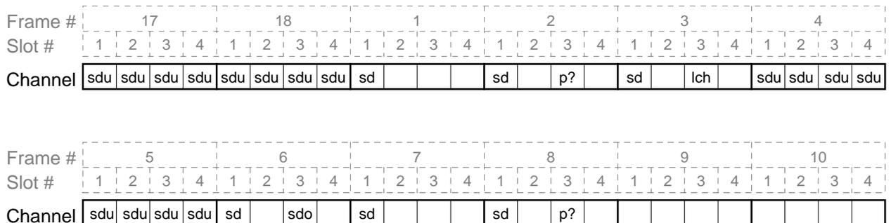
Figure F.1: Call sequence for SDS - for unacknowledged data
