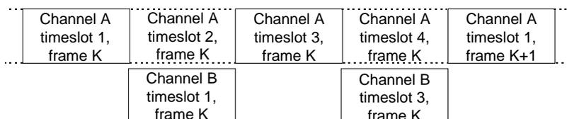
Figure 19: Illustration of DM channel A and B timeslots
