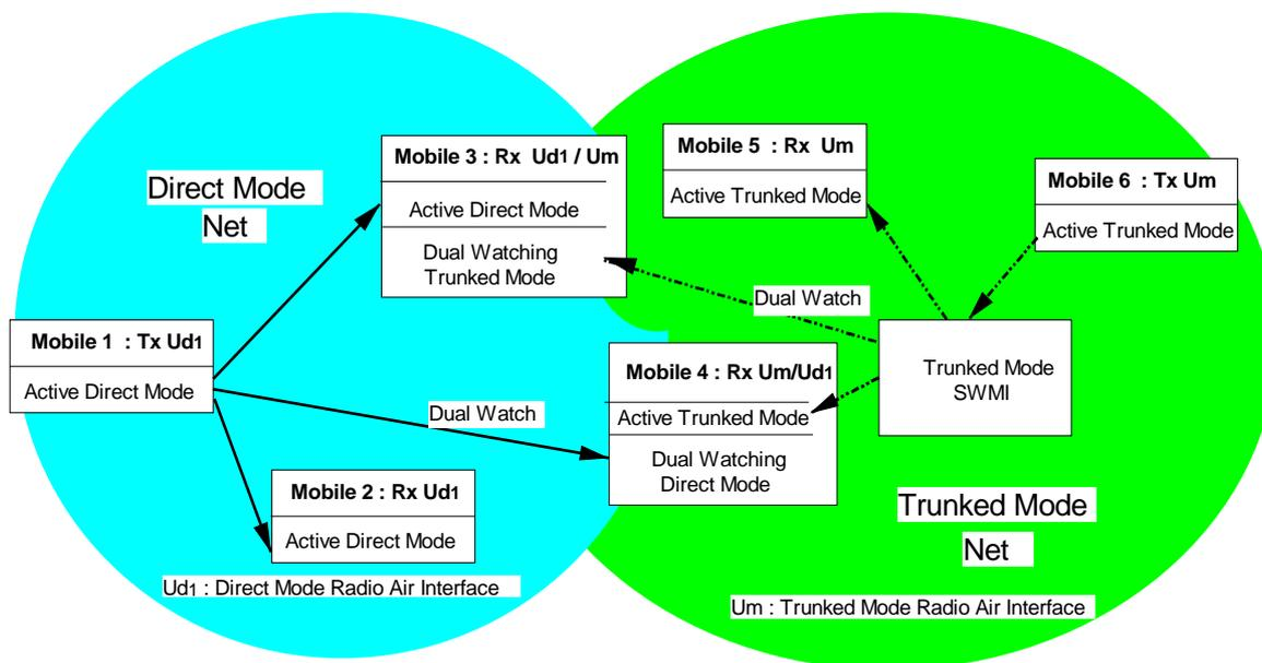
**Figure 8: Functional network configuration showing Direct Mode MS-MS air interface.**
