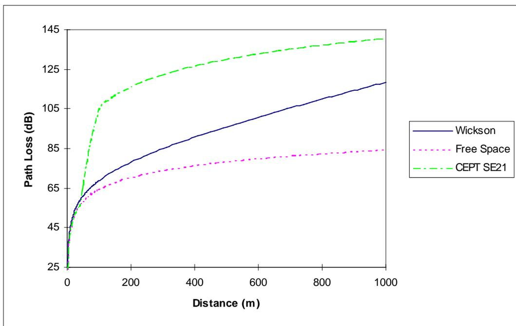
Figure 23: Characteristics of the short range propagation models
