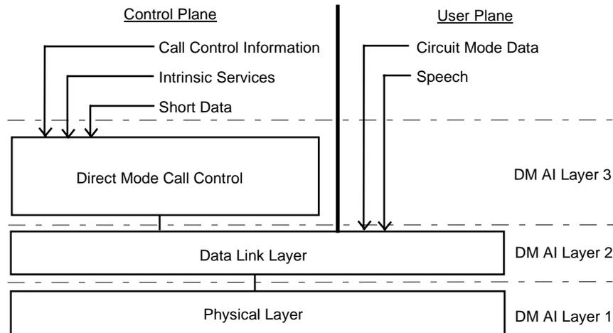
**Figure 13: Protocol stack for direct MS-MS operation**
