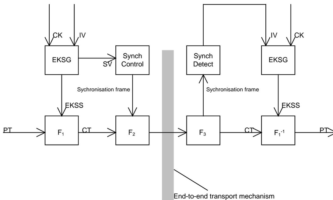
Figure B.2: Functional diagram of voice encryption and decryption mechanisms
