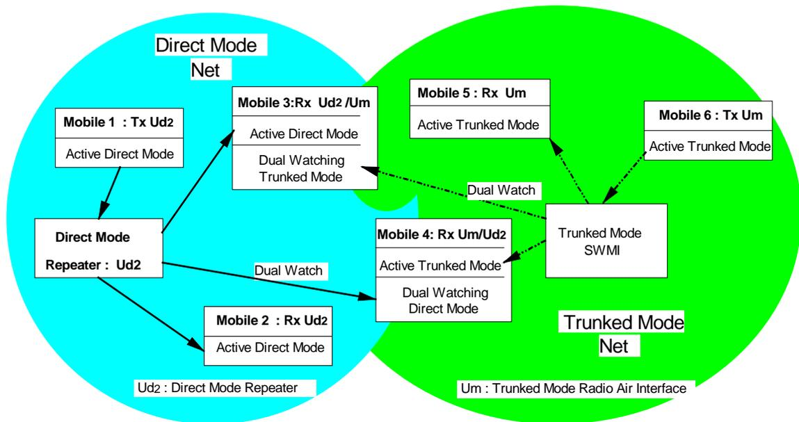
**Figure 9: Functional network configuration showing Direct Mode Repeater air interface.**
