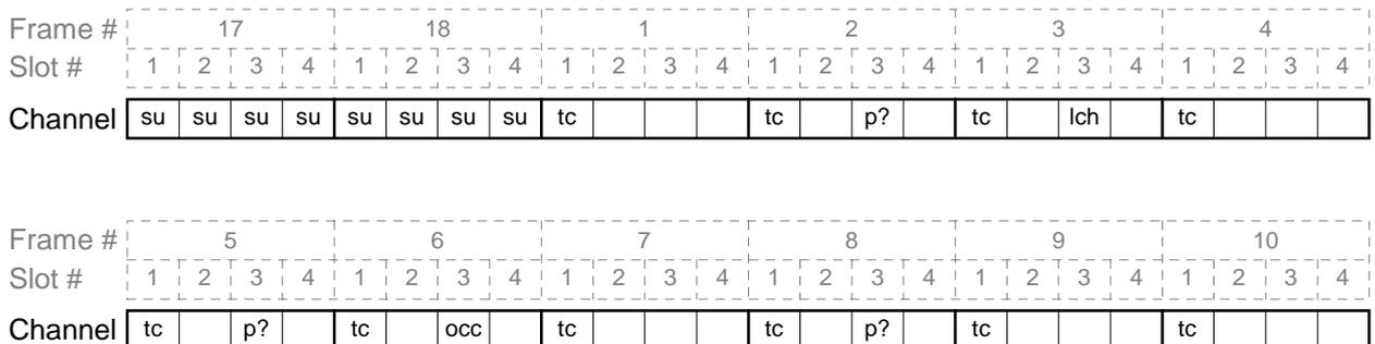
**Figure 14: Call sequence for set-up without presence check**
