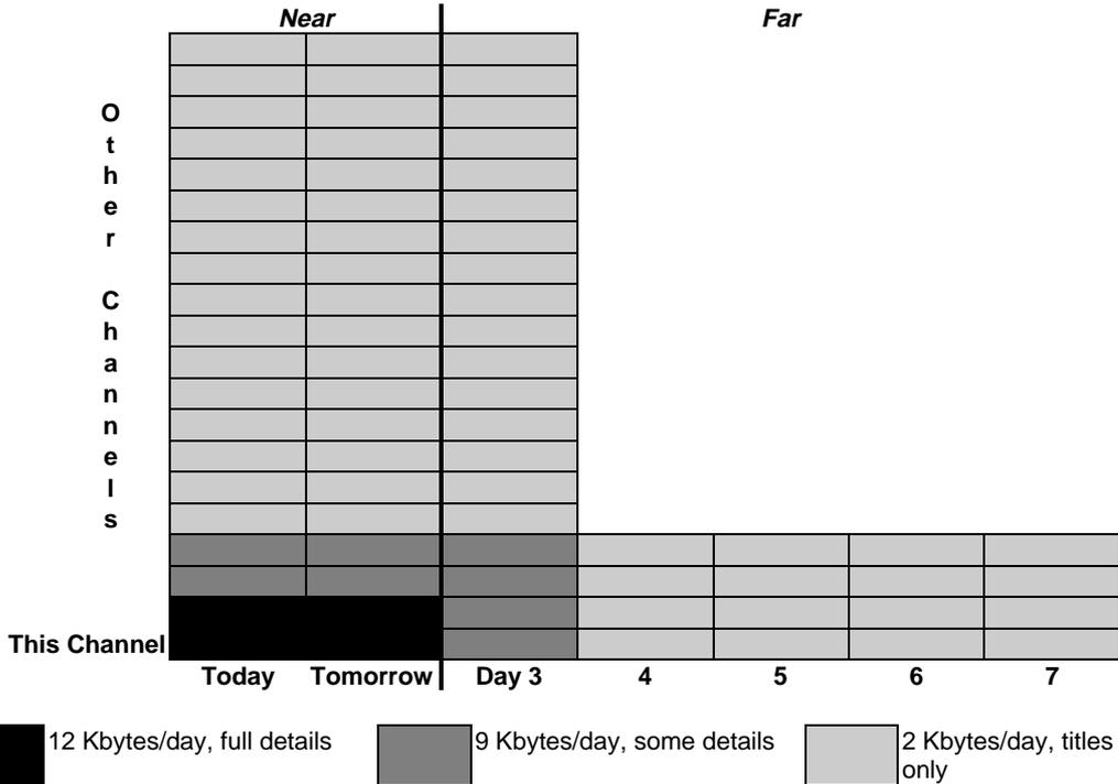
The menu and navigation components are estimated at 20 Kbytes. A 5 minute rate is chosen for the *Near Information* from other channels, and a 20 minute rate for all *Far Information*.
