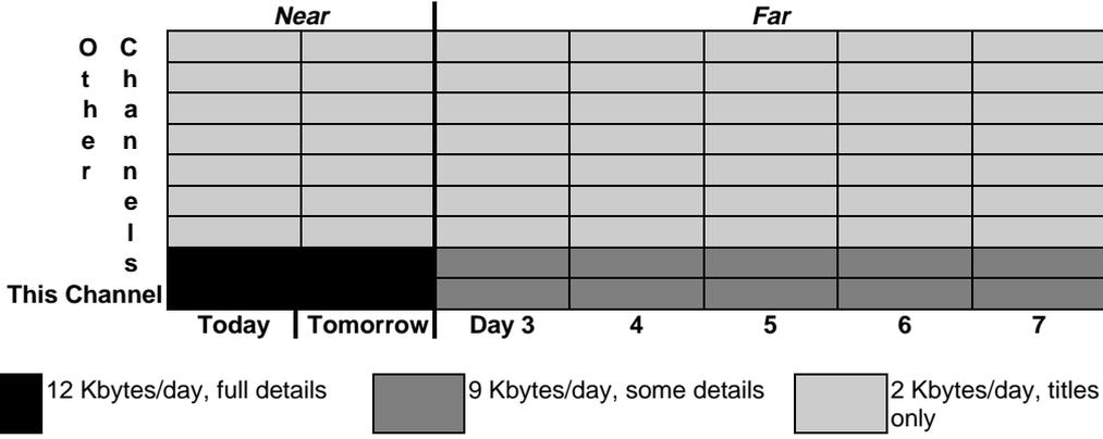
The menu and navigation components are estimated at 25 Kbytes. A 3 minute rate is chosen for the *Near Information* from other channels, and a 20 minute rate for all *Far Information*.
