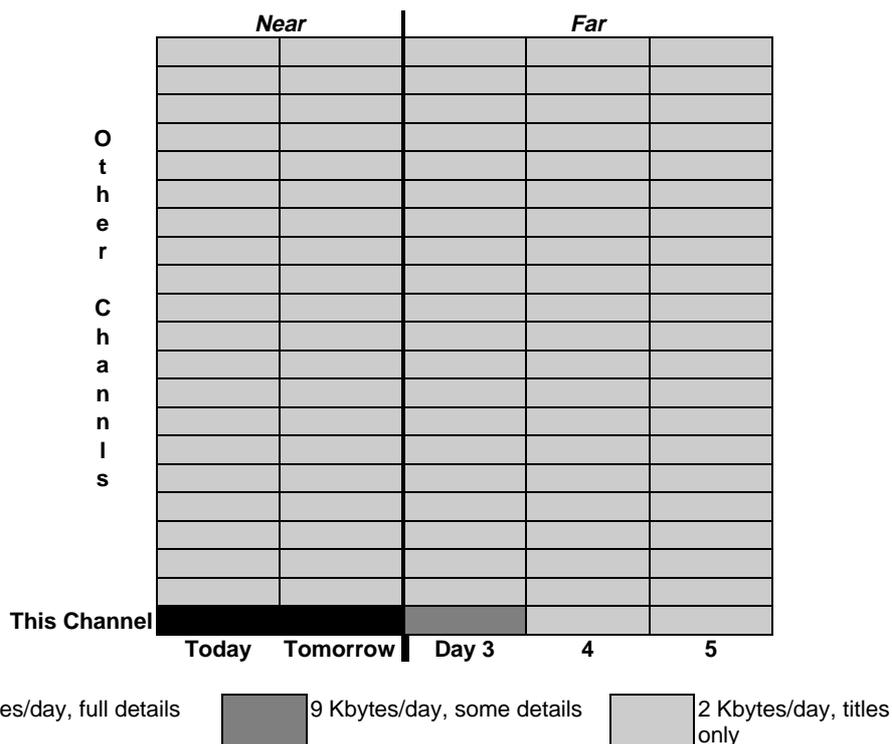
The menu and navigation components are estimated at 15 Kbytes. A 5 minute rate is chosen for the remaining *Near Information*, and a 20 minute rate for all *Far Information*.
