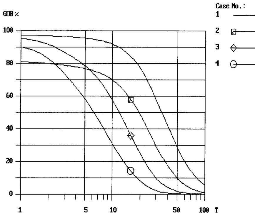
Case 1: STMR = 15 dB; TELR = 30 dB. Case 2: STMR = 25 dB; TELR = 30 dB. Case 3: STMR = 15 dB; TELR = 20 dB. Case 4: STMR = 25 dB; TELR = 20 dB
