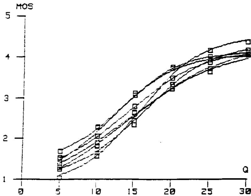
Figure E.1: MOS as function of quantizing distortion Q in a MNRU; seven different subjective tests
