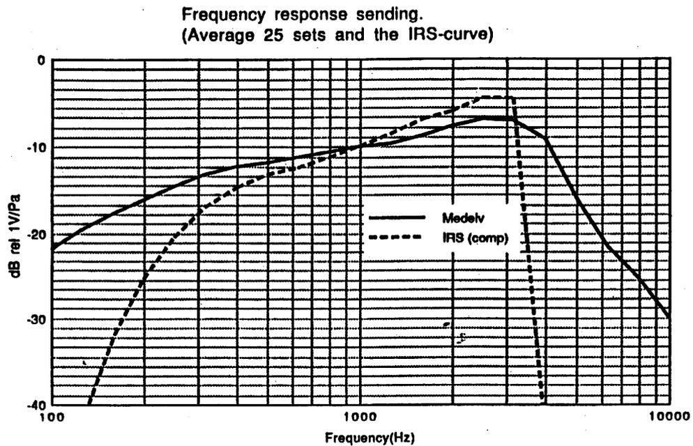
Figure 8: Frequency response sending, IRS and mean value of 25 approved Swedish handsets
