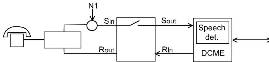
Figure D.4: Speech detector/Echo control device interactions
