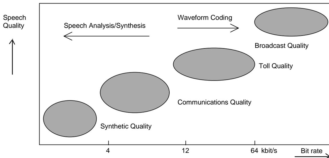
**Figure 35: Quality of speech coding transmission rates**
