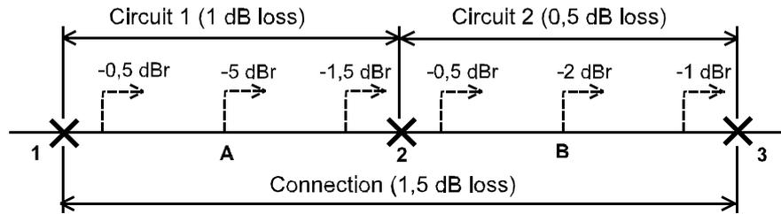
**Figure C.3: Example of relative levels and losses in a connection consisting of two (ITU-T) circuits, where there is, for stability reasons, a "level jump" of 1 dB in exchange 2**
