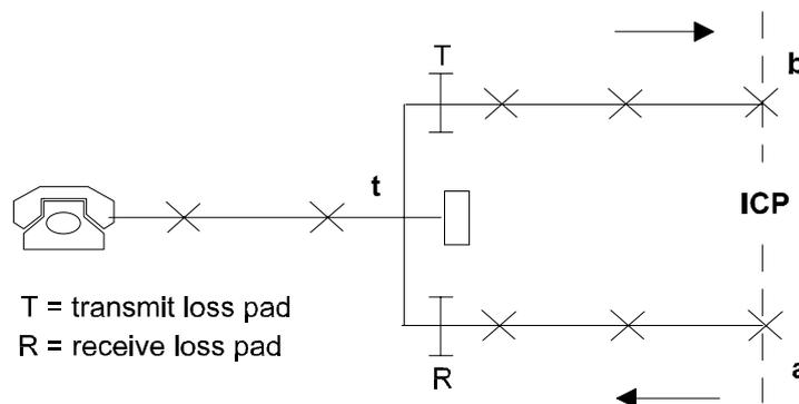
Figure 24: Loss of the path a-t-b of a national system
