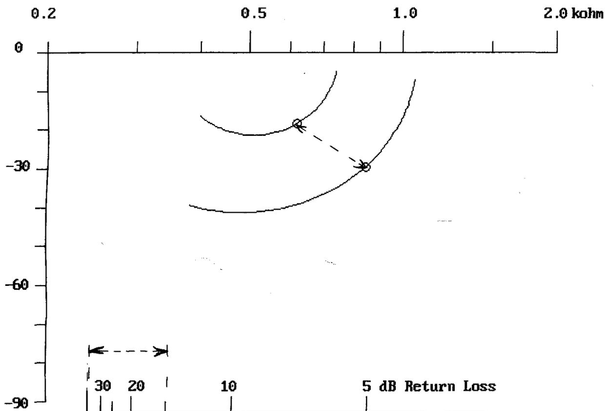
NOTE: X-axis = Absolute value in kΩ; Y-axis argument in degrees of impedance.
