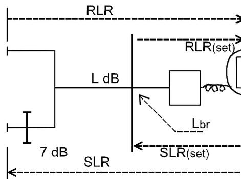
NOTE:  $L$  = loss of the subscriber line.  $L_{br} = L_{st}$  = weighted average of the return loss between the equ. sidetone balance impedance  $Z_b$  and the input impedance  $Z$  of the line.
