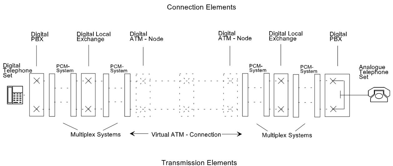
**Figure 2: Configuration for a fully digital connection including ATM sections with a terminating hybrid**
