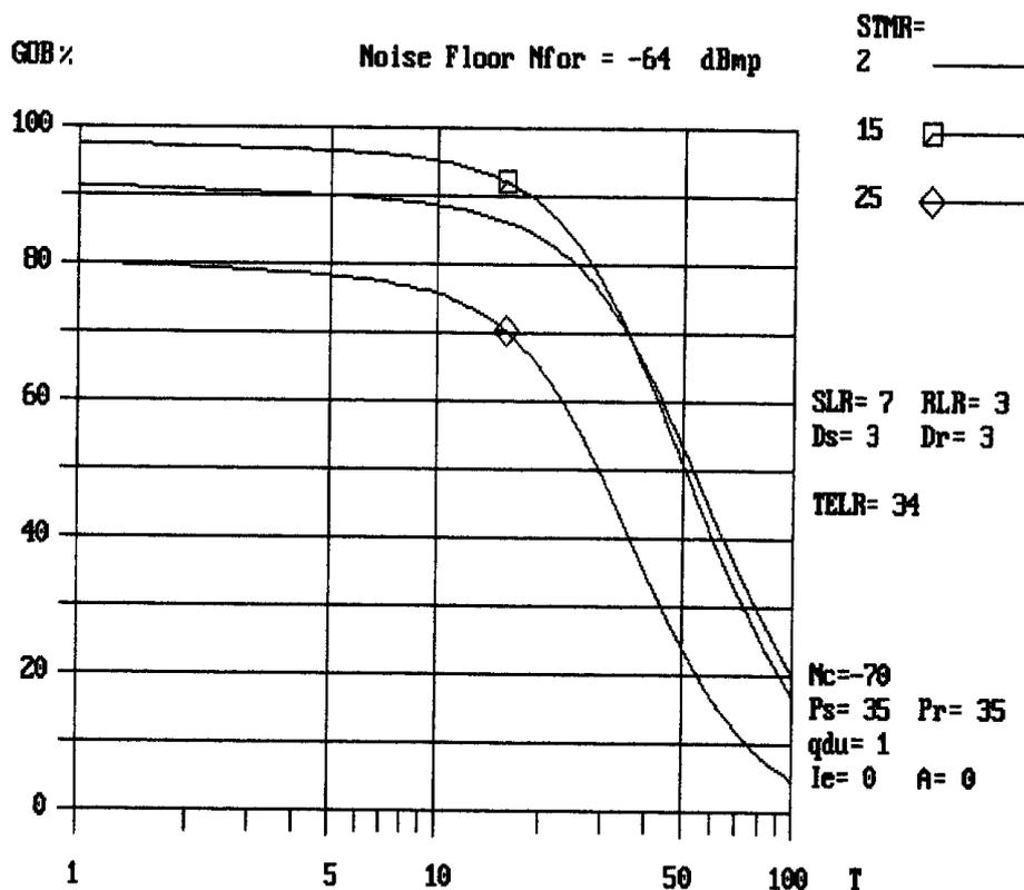
Figure F.6: GOB as function of mean one-way-delay for  $TELR = 34$  dB; STMR as parameter
