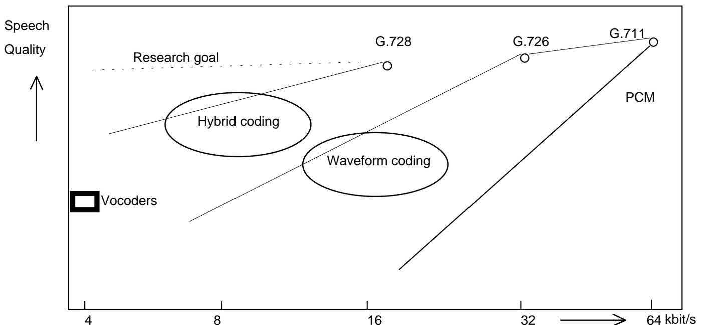
Figure 36: Quality of telephone speech as a function of the bit-rate
