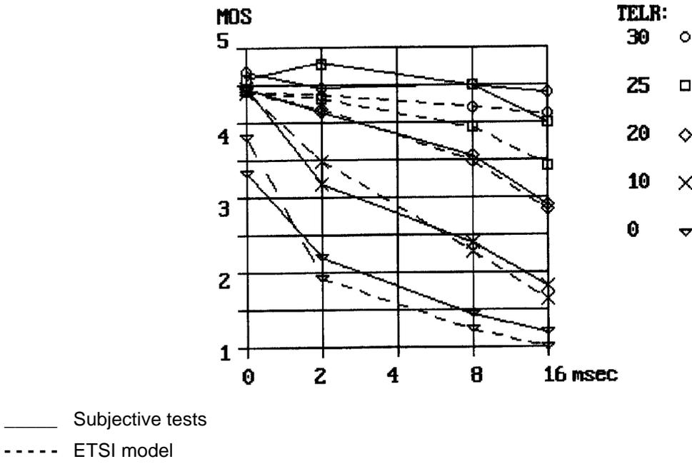
Figure 62: Subjective MOS - values, reference [4], and predicted values, ETSI model, for short-delay talker echoes. (T = mean one-way delay)
