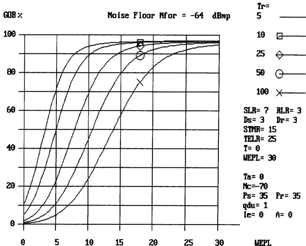
Figure F.5: GOB as function of listener echo WEPL dB; round-trip delay  $T_r$  ms as variable
