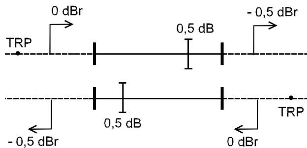
NOTE: TRP = the Transmission Reference Point, i.e. the circuit 0 dBr reference point.
