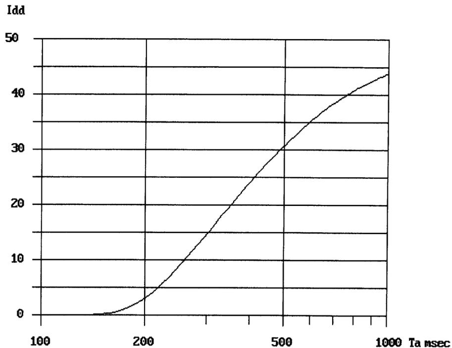
Figure 52: Impairment factor Idd as function of the absolute one-way transmission time Ta
