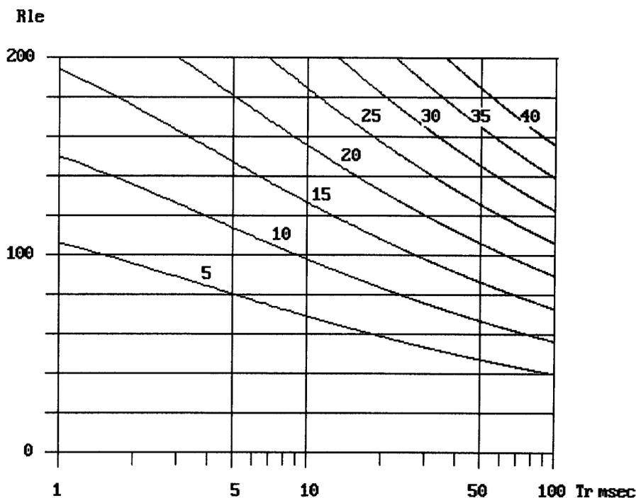
Figure 50: Parameter *Rle* as function of round-trip delay *Tr*; curve parameter = WEPL
