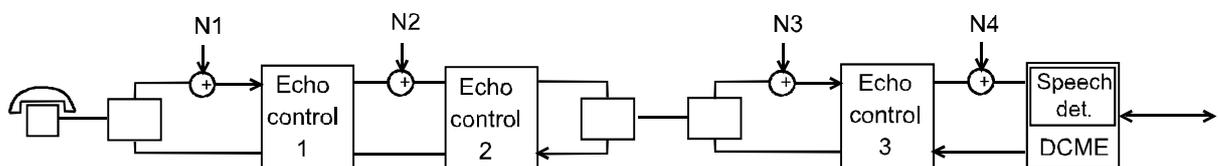
Figure D.5: Multiple echo control device configuration
