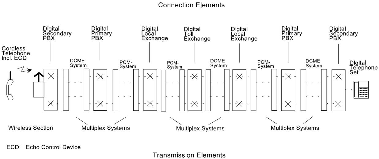
Figure 4: Configuration for a cordless telephone connected via DCME equipment
