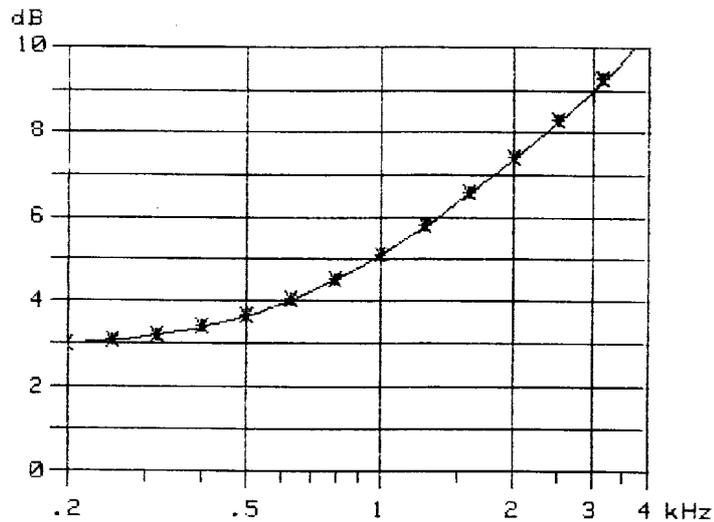
**Figure 13: Typical attenuation of an unloaded cable (3 km; 0,4 mm copper; 50 nF/km)
