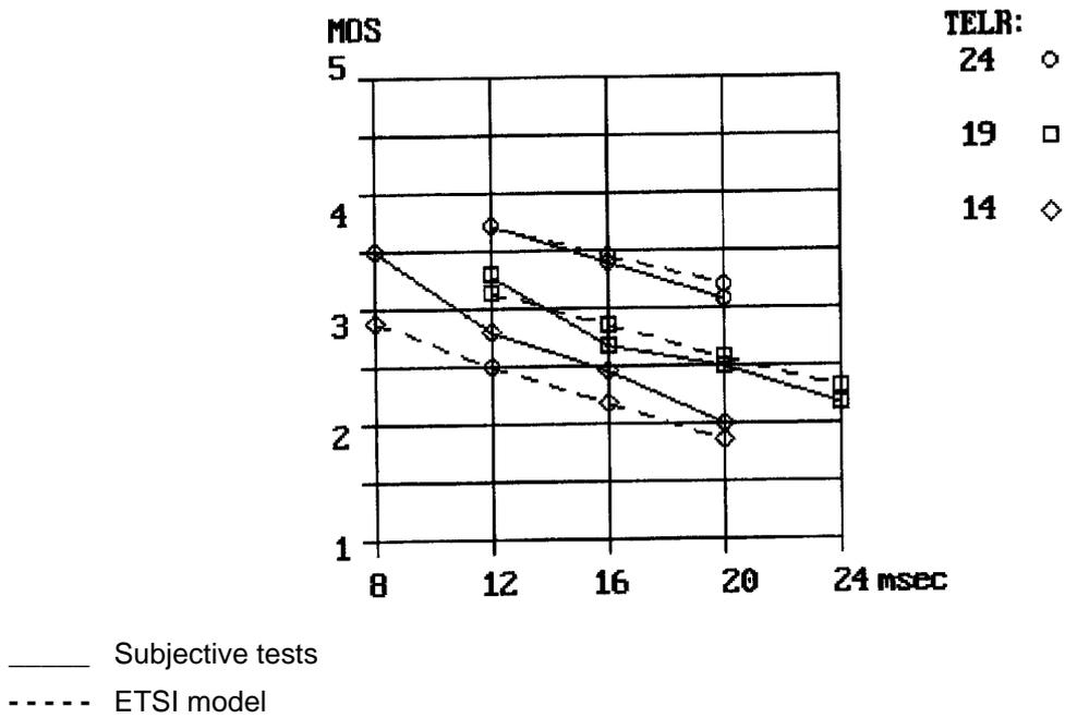
Figure 63: Subjective MOS - values, reference [57], and predicted values, ETSI model, for short-delay talker echoes. (T = mean one-way delay)
