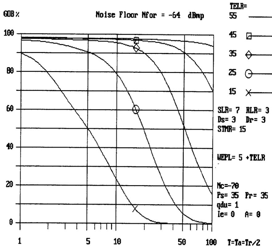
Figure F.8: The influence of talker echo. GOB as function of mean one-way delay T ms; TELR as variable
