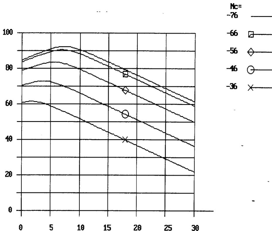
Figure 57: The  $R$ -factor as function of OLR and  $N_c$  at  $RLR = 0$  dB; the ETSI model ( $N_c$  in dBmp)
