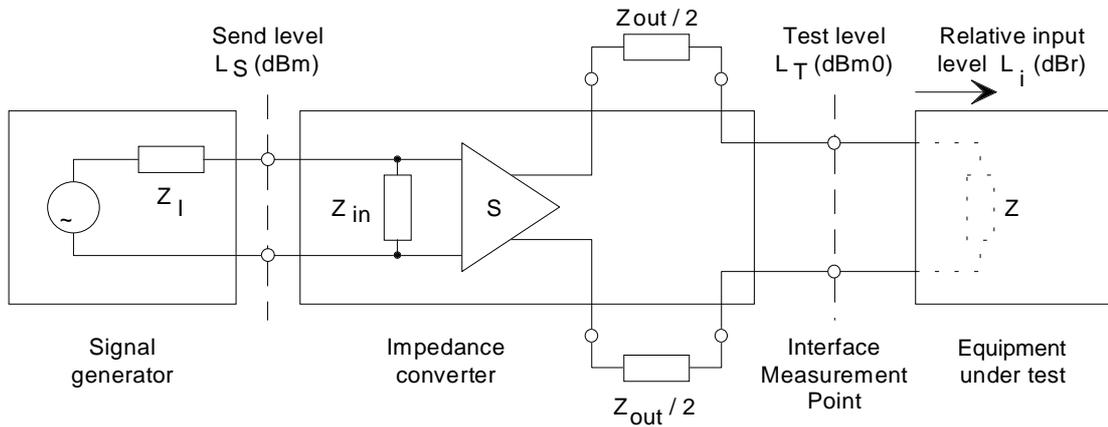
Figure C.4: Impedance converter in the sending path
