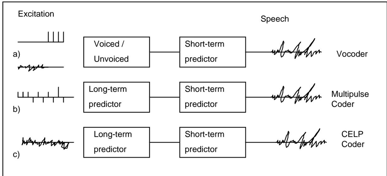
**Figure 37: Models of speech excitations in vocoders (a) and hybrid coders (b, c)**
