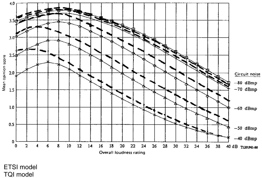
Figure 58: Comparison between the ETSI and the TQI models; MOS as function of OLR and Nc at RLR = 0 dB
