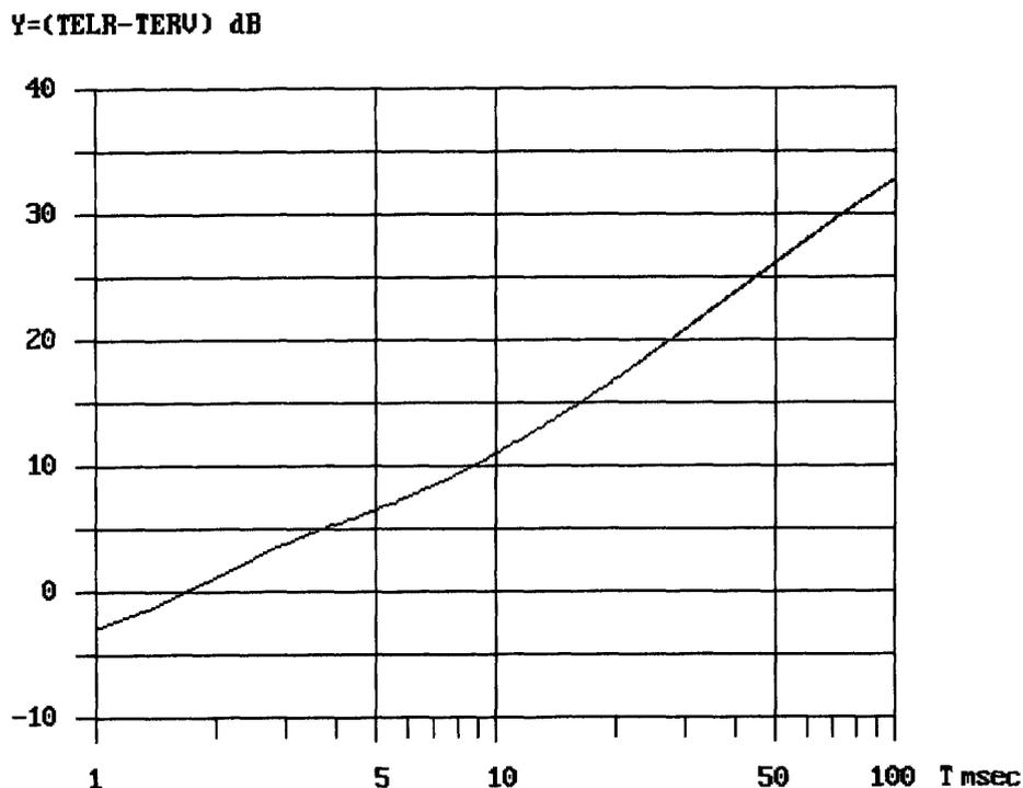
Figure 47: TERV = TELR - Y; T = mean one-way transmission time
