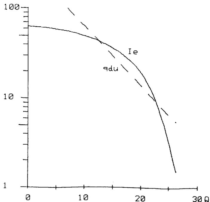
Figure G.3: Equipment impairment factor  $I_e$  and quantizing distortion  $q_{du}$  as functions of the MNRU quantizing distortion  $Q$
