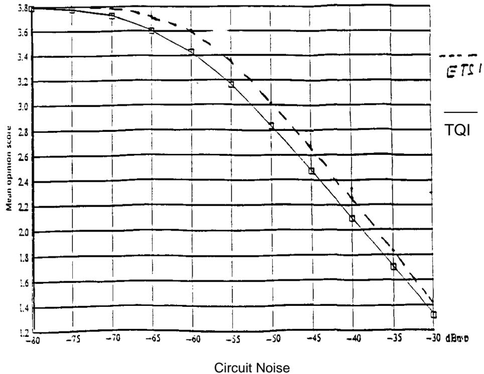
Figure 59: Comparison between the ETSI and the TQI models. MOS(Nc), OLR = 10 dB; RLR = 0 dB
