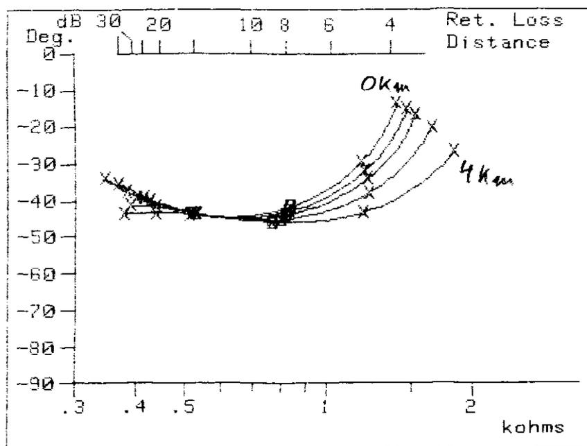
Figure A.3: Input impedance of cable terminated by impedance a). Length 0, 0,5, 1, 2 and 4 km. 0,5 mm Cu, 50 nF/km. Frequency markings at 0,2, 0,5, 1, 2, 3, 4 kHz
