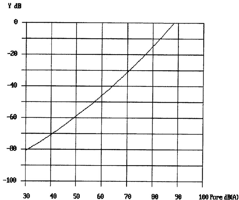
Figure 43: Equivalent circuit noise  $N_{or}$  dBm0p caused by the effective room noise at side R.
