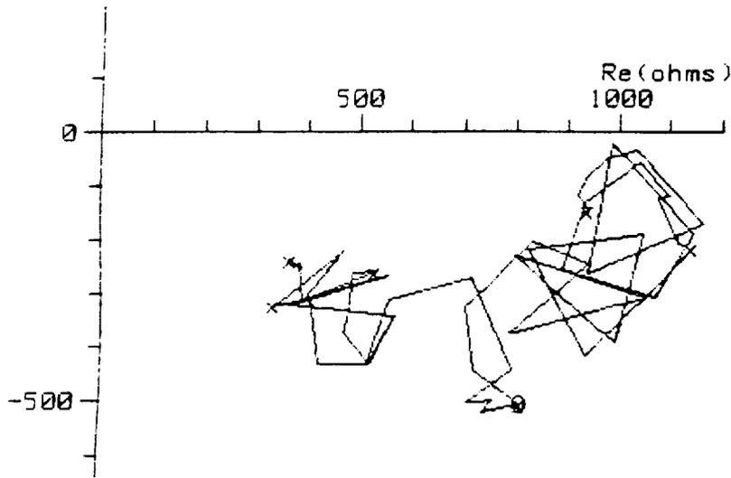
NOTE: The diagram in figure A.8 is based on impedance calculations at 54 frequencies, spaced 1/12 octave apart, in the range 200 Hz to 4 000 Hz. For simplicity, the impedance points in the diagram have been connected by straight lines. In reality, due to the rapid change of phase with frequency in the exchange 4-wire loop, the impedance curve between two points will consist of arcs-segments of circles.
