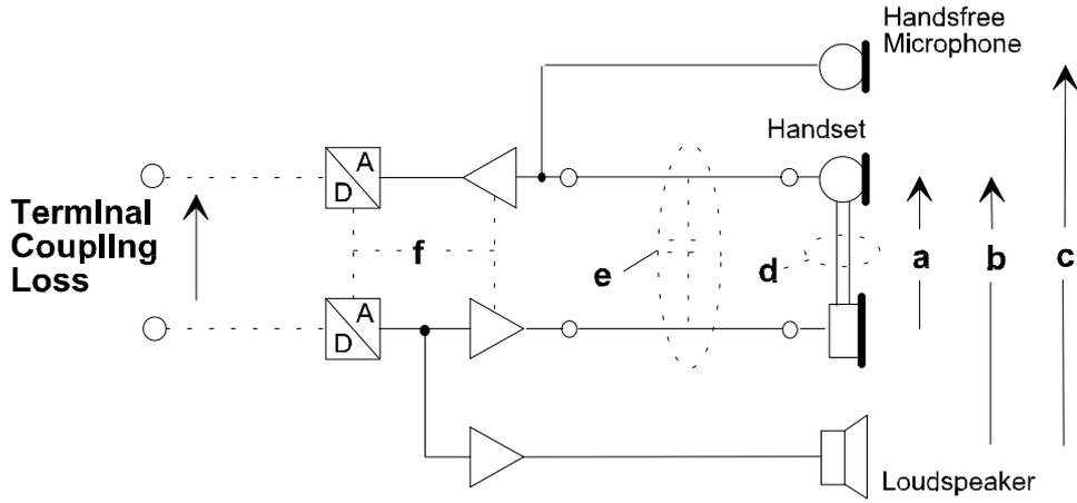
**Figure 21: Coupling in a digital telephone set**
