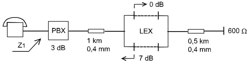
Figure A.6: Example of a digital PBX connected two-wire to a digital local exchange (LEX)
