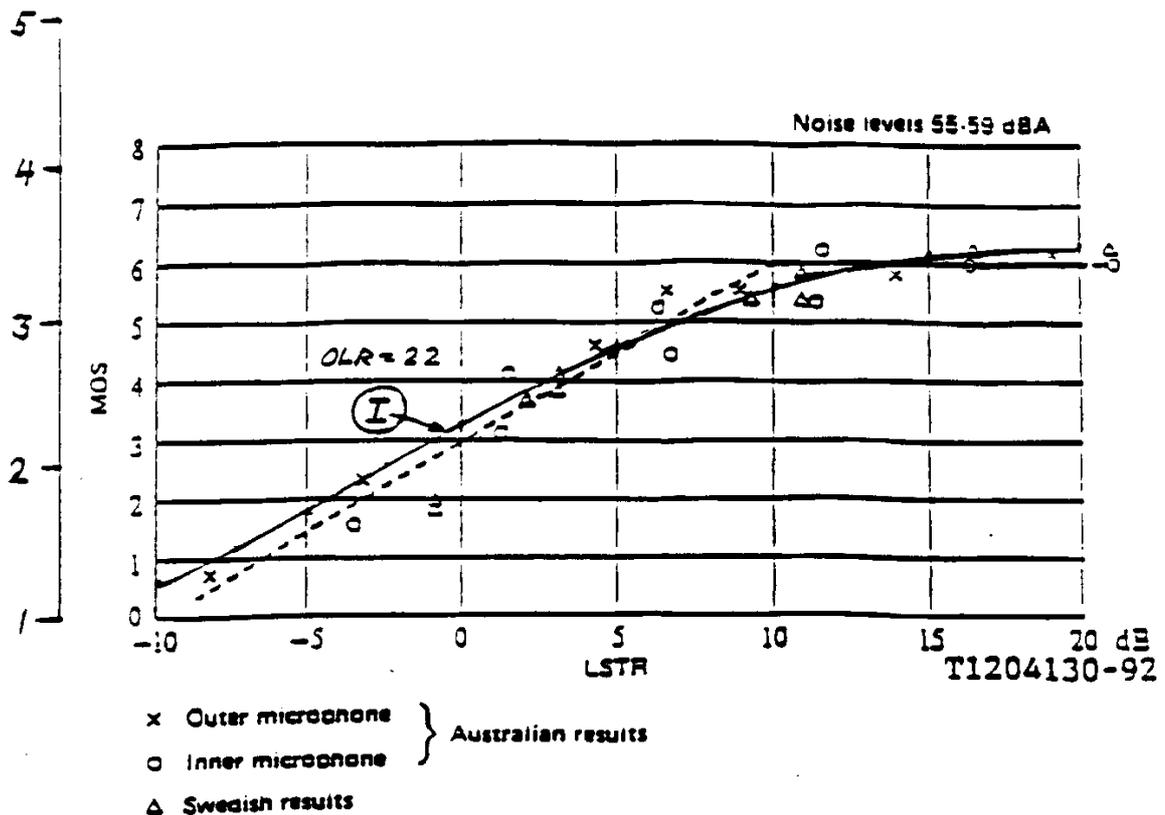
Figure 61: MOS for listening tests as function of LSTR for a quiet connection.
