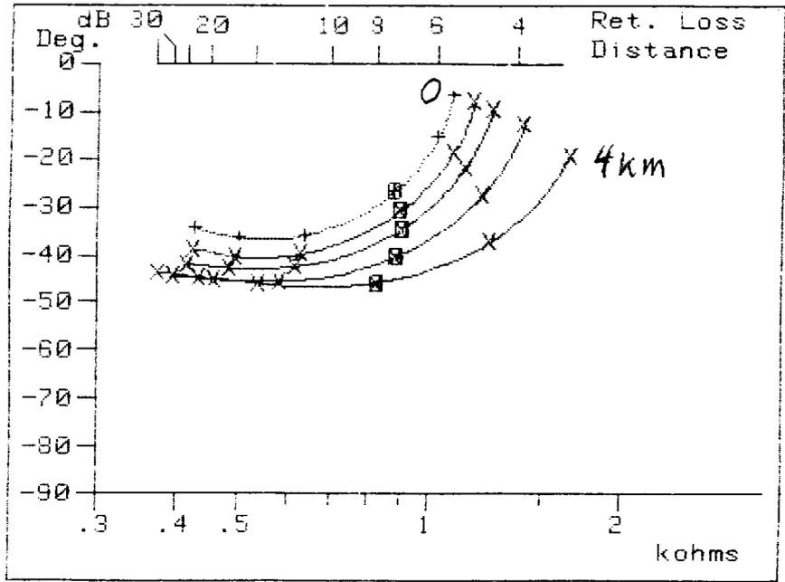
Figure A.4: Input impedance of cable terminated by impedance b). Length 0, 0.5, 1, 2 and 4 km. 0,5 mm Cu, 50 nF/km. Frequency markings at 0,2, 0,5, 1, 2, 3, 4 kHz
