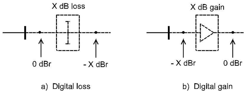
**Figure C.1: Conventions, in the context of equipment specification and testing, for relative level of a digital bit stream when digital signal processing is applied**
