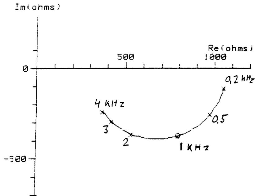
Figure A.7: Input impedance  $Z_1$  seen by the telephone in figure A.6; perfect balancing at the exchange port of the PBX
