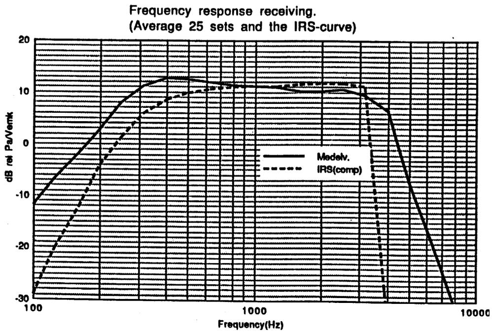
Figure 9: Frequency response receiving, IRS and mean of 25 approved Swedish sets
