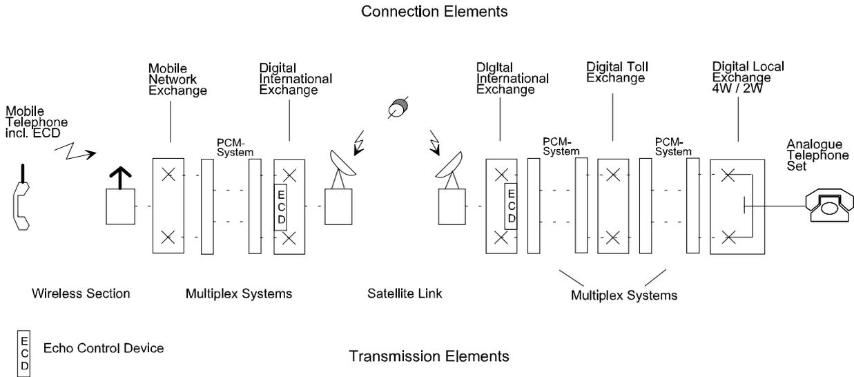
Figure 3: Configuration for a mobile telephone connected via satellite link
