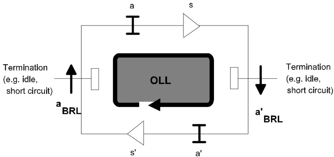
**Figure 23: Stability of a 4-wire loop**
