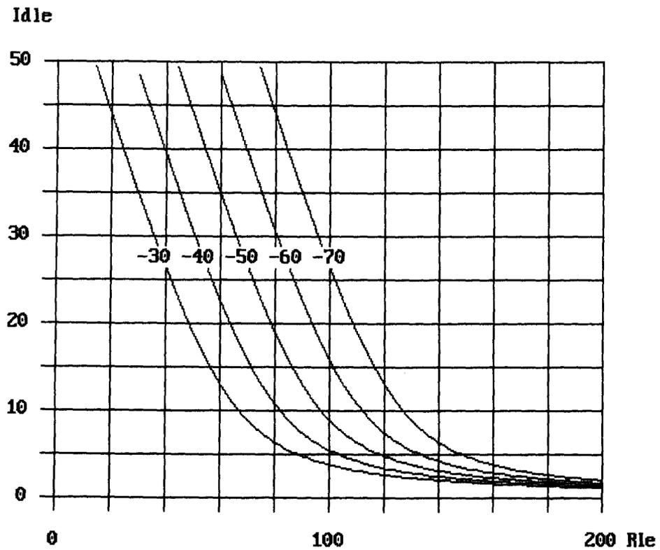
Figure 51: Impairment factor Idle as function of parameter Rle; curve parameter = (SLR + No) dBmp
