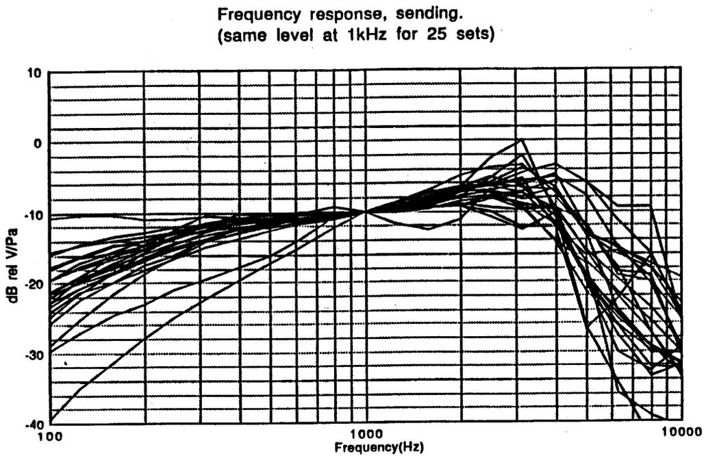
Figure 10: Frequency response, sending. The level is adjusted to -10 dB relative to 1 V/Pa at 1 000 Hz for all 25 set
