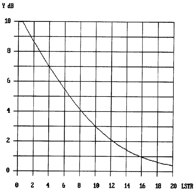
Figure 42: Enhancement of room noise  $P_{or}$  to  $P_{ore}$  due to LSTR at side R.  $P_{ore} = P_{or} + Y$  dB(A)
