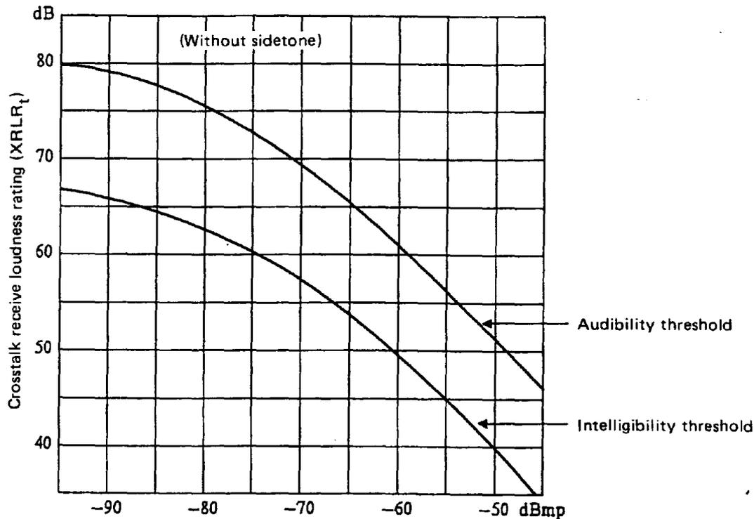
Figure 32: Threshold values of crosstalk receive loudness rating XRLR (referred to a 0 dBr point)
