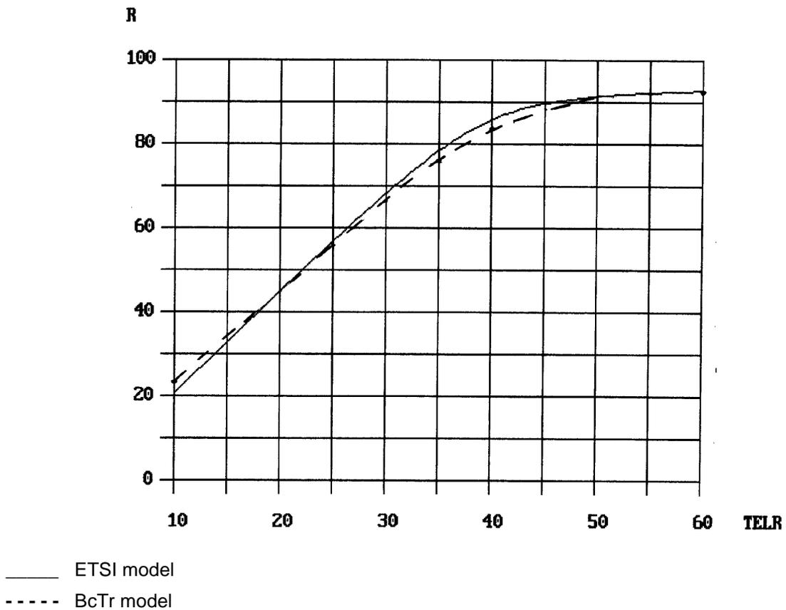
Figure 64: Rating factor *R* as function of TELR. OLR = 10 dB (SLR = 7 dB, RLR = 3 dB), T = 25 ms, Nc = -70 dBm0p
