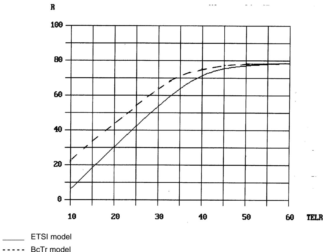
Figure 65: Rating factor R as function of TELR. OLR = 20 dB (SLR = 17 dB, RLR = 3 dB),
