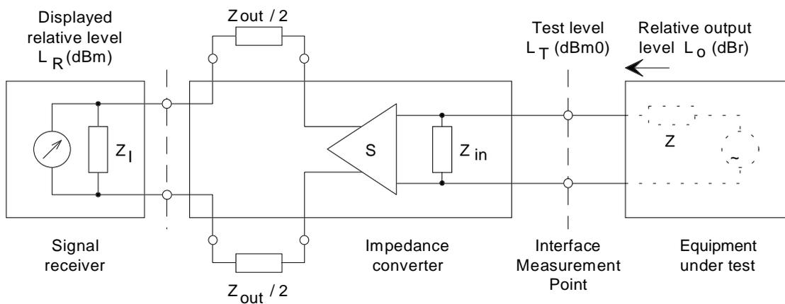
Figure C.5: Impedance converter in the receive path
