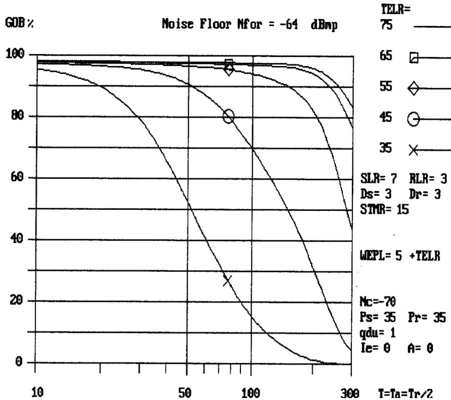
T = mean one-way delay for talker echo; Ta = one-way absolute delay from side S to side R; Tr = round-trip delay for listener echo, all measured in ms; TELR as variable.
