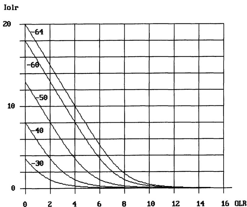
Figure 44: Impairment factor *Iolr* as function of *OLR*. Parameter for the curves is  $N_t = N_o - RLR$  dBmp;  $N_o$  = circuit noise (in dBm0p) at the 0 dBr point
