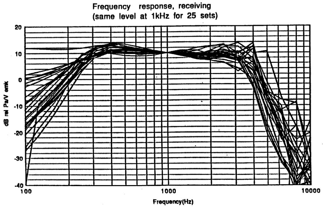
Figure 11: Frequency response, receiving. The level is adjusted to -10 dB relative to 1 Pa/V e.m.f. at 1 000 Hz for all 25 sets
