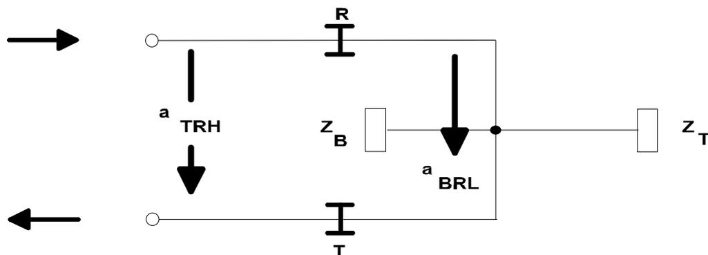
Figure 20: Balance return loss and transhybrid loss
