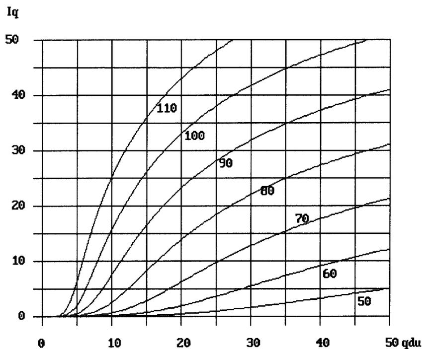
Figure 46: Impairment factor  $I_q$  as function of  $q_{du}$ . Curve parameter =  $(SLR + N_o)$  dBmp
