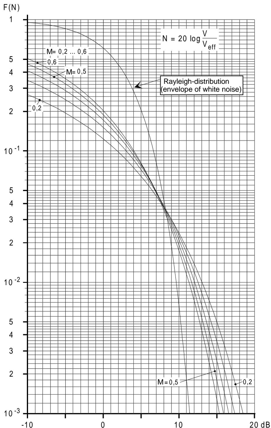
**Figure 30: Cumulative statistical distribution of speech signals and of white noise envelope**
