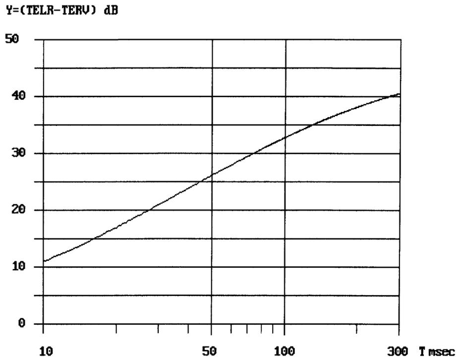
Figure 48:  $TER_V = TEL_R - Y$ ;  $T$  = mean one-way transmission time
