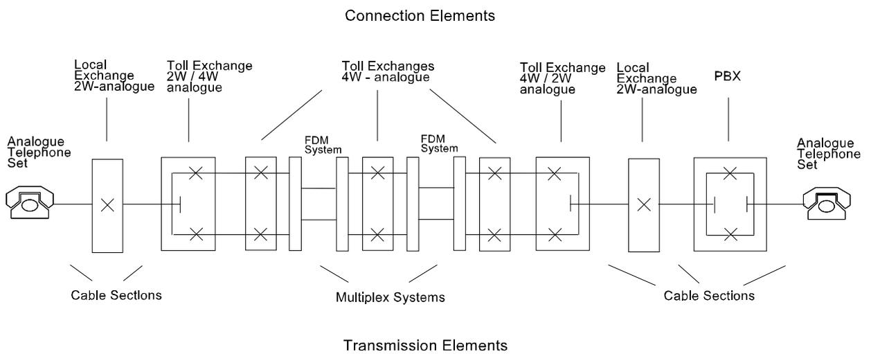
**Figure 1: Typical configuration for a fully analogue connection**
