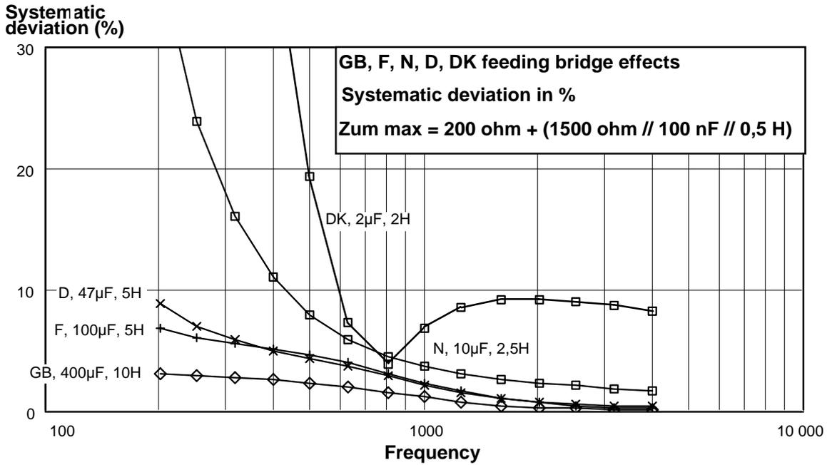
Figure D.4: GB, F, N, D, DK feeding bridge effect on the impedance ( $Z_{um\ max}$ ) measurement and related systematic deviation
