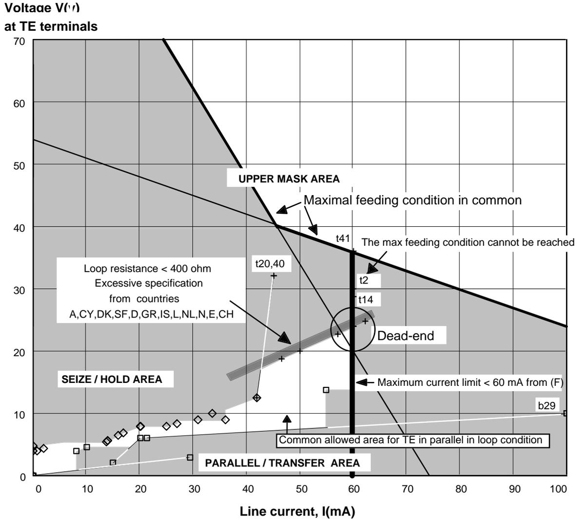
**Figure A.13: Common allowed area available in the intersection of the 19 country masks (case of TE in parallel in loop condition)**
