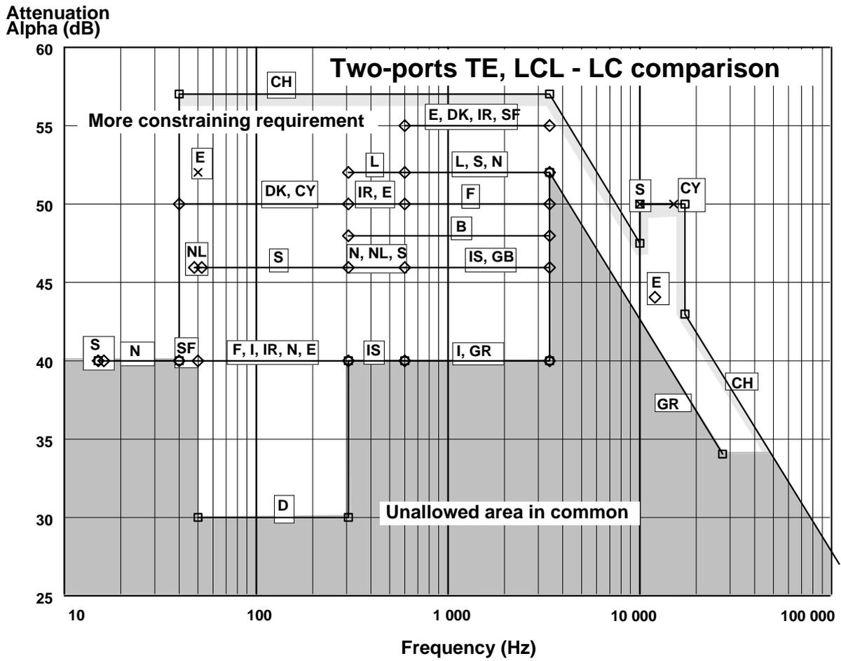
Figure C.4: Comparison of the attenuation value for all countries for the degree of unbalance about earth, case of LCL in loop condition (LC) for one port TE
