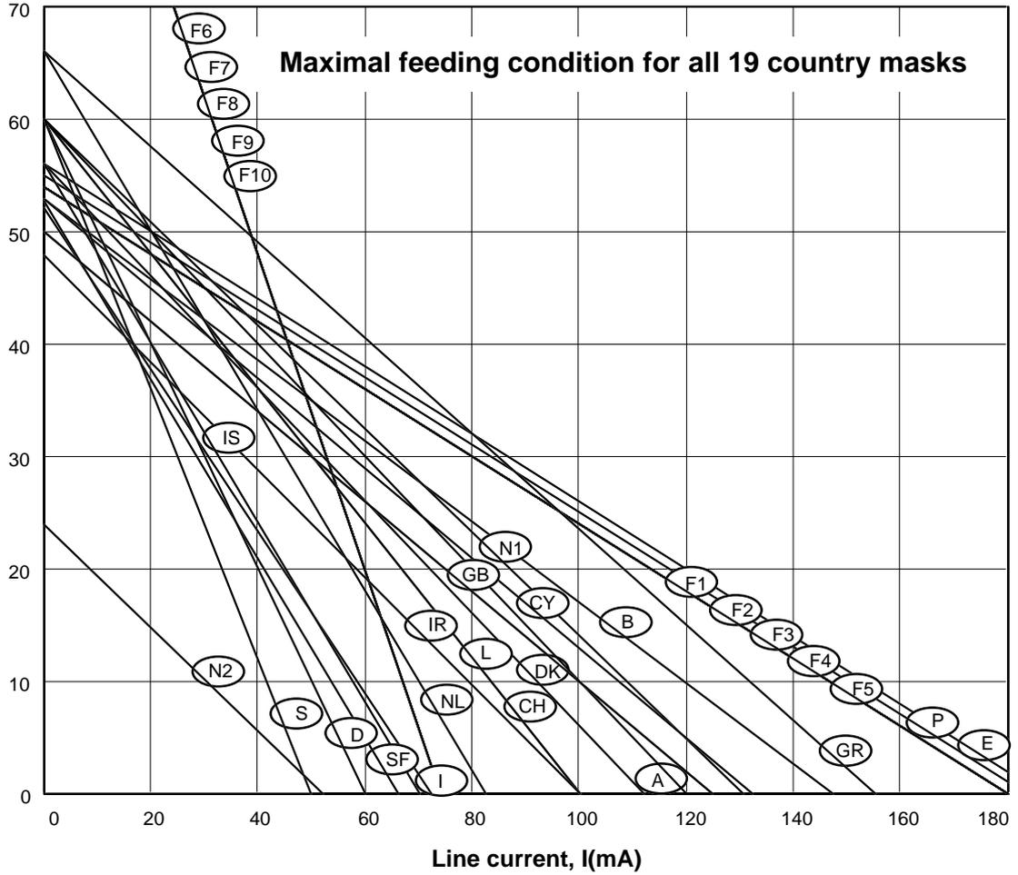
Figure A.11: Maximal feeding condition limits of the 19 country masks
