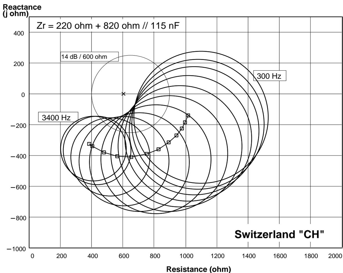
Values of the reference impedance and return loss limits for Switzerland "CH":
