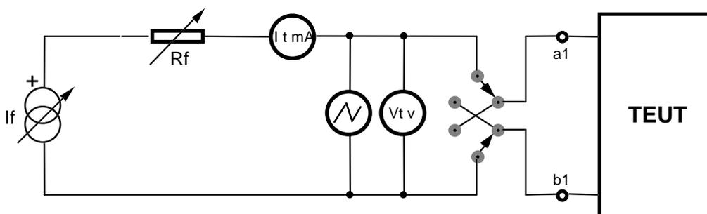
Figure D.13: DC current and loop resistance, Test 2, Constant current feeding for stability test
