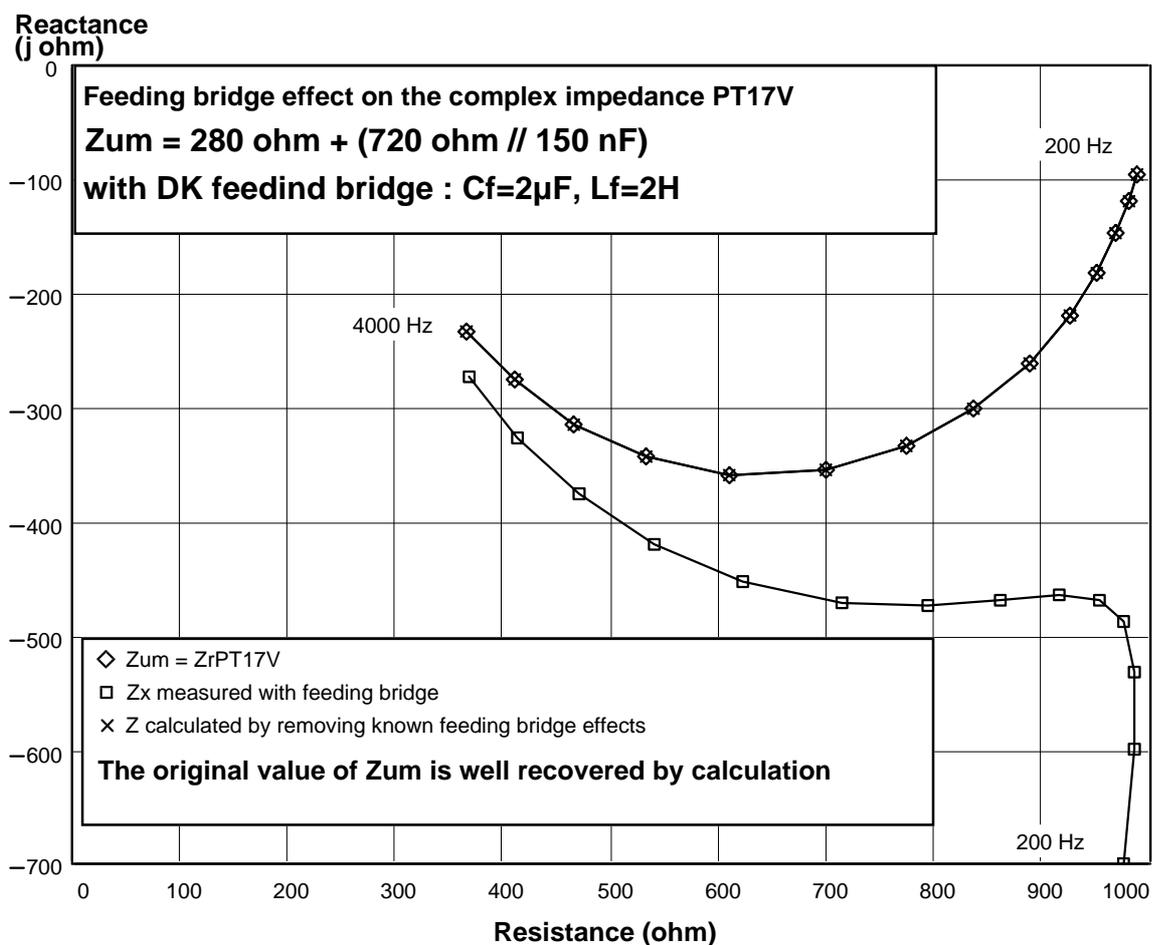
Figure D.8: Reduction of the systematic deviation due to the feeding bridge by calculation
