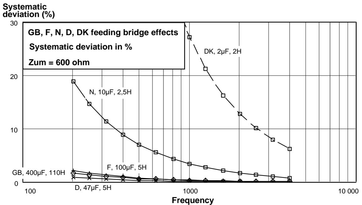
Figure D.3: GB, F, N, D, DK feeding bridge effect on the impedance (600 ohm) measurement and related systematic deviation
