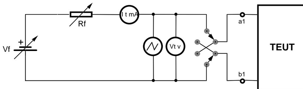
Figure D.12: DC current and loop resistance, Test 1, Test 3, Test 4 for respectively, DC characteristic plotting, constant voltage feeding stability, loop starting closure voltage
