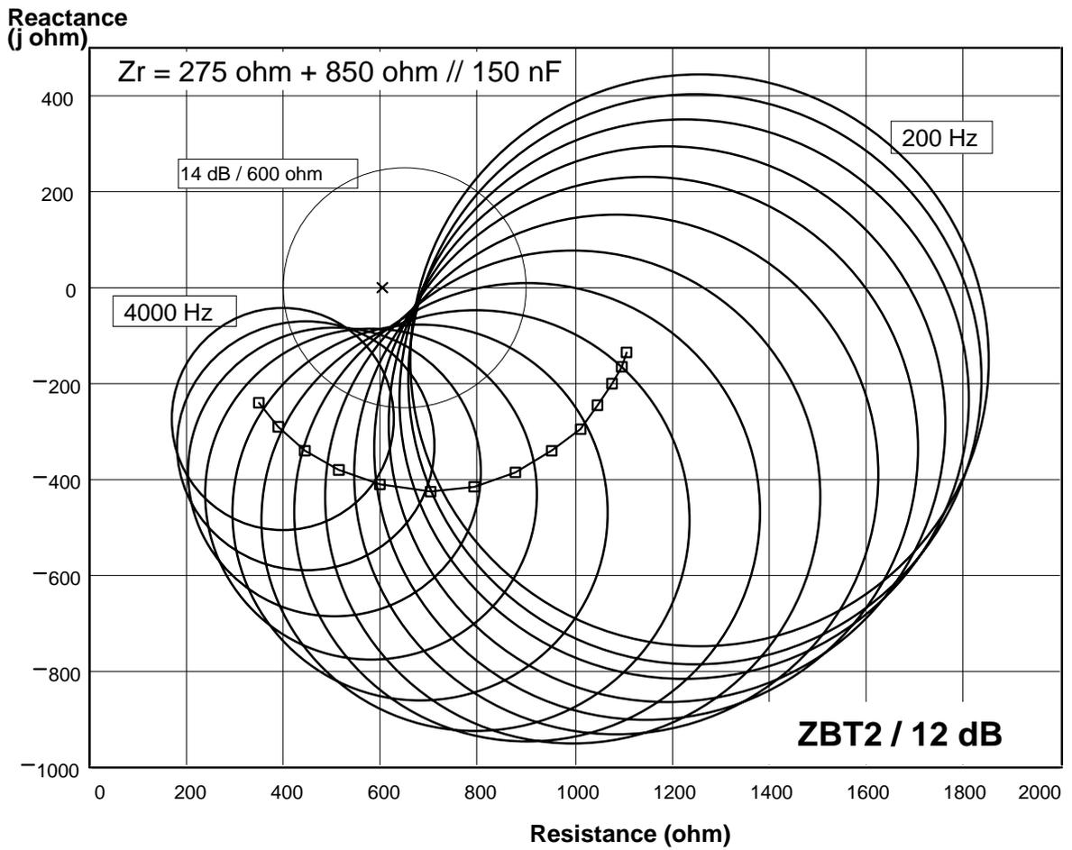
Values of the reference impedance and return loss limits for ZBT2 12dB:
