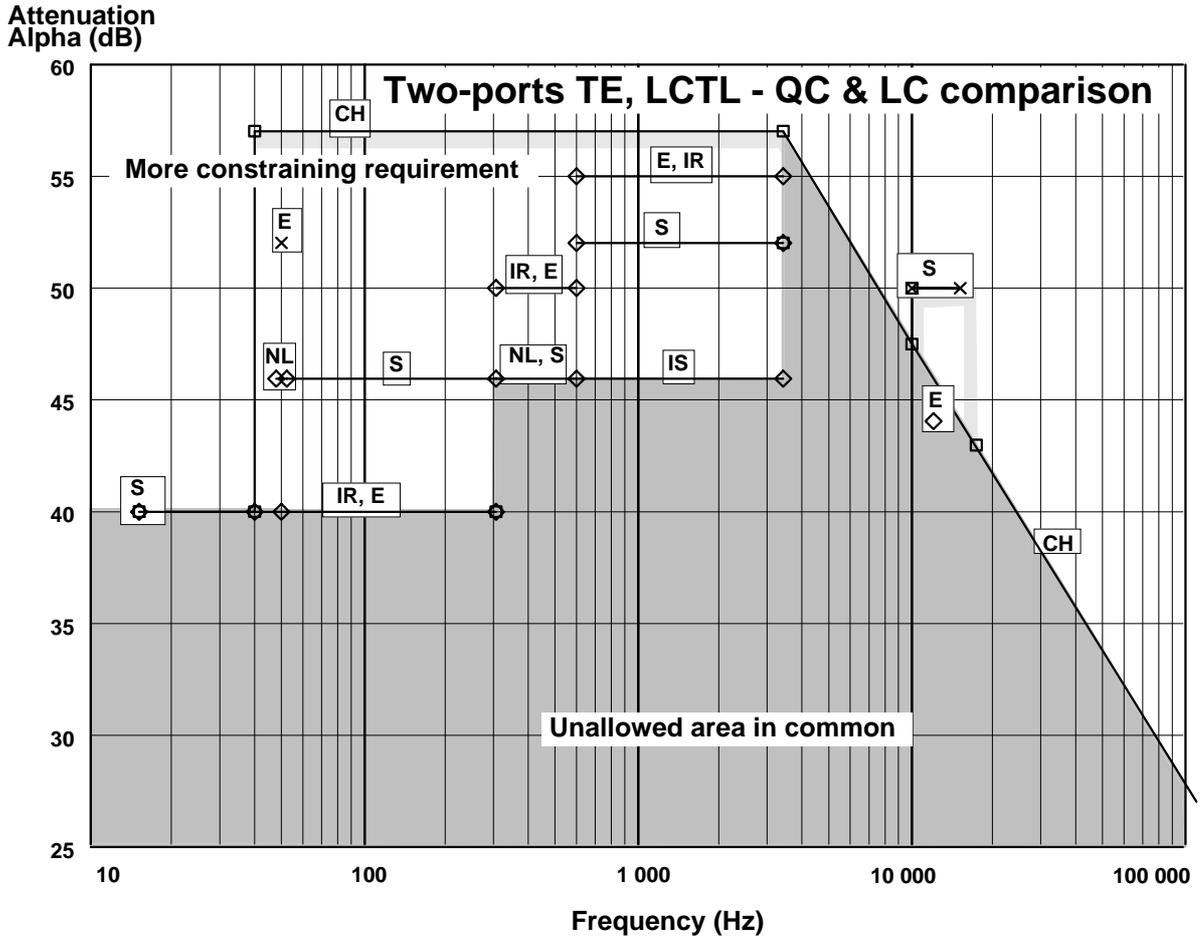
Figure C.5: Comparison of the attenuation value for all countries for the degree of unbalance about earth, case of LCL in quiescent and loop condition (QC and LC) for two ports TE
