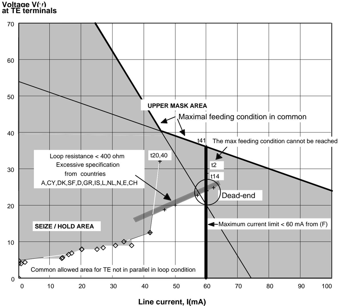
**Figure A.12: Common allowed area available in the intersection of the 19 country masks (case of TE never in parallel in loop condition)**
