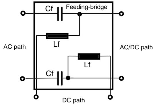
Figure D.9: Feeding bridge circuit
