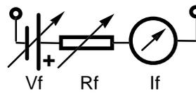
Figure D.10: DC feeding supply and adjustable feeding resistance
