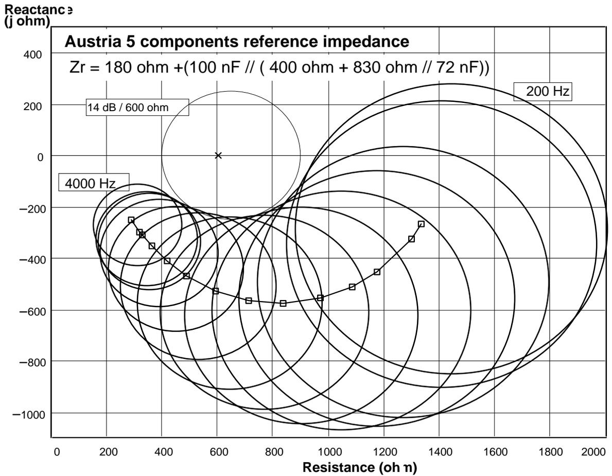
Values of the 5 components reference impedance and return loss limits for Austria "A":
