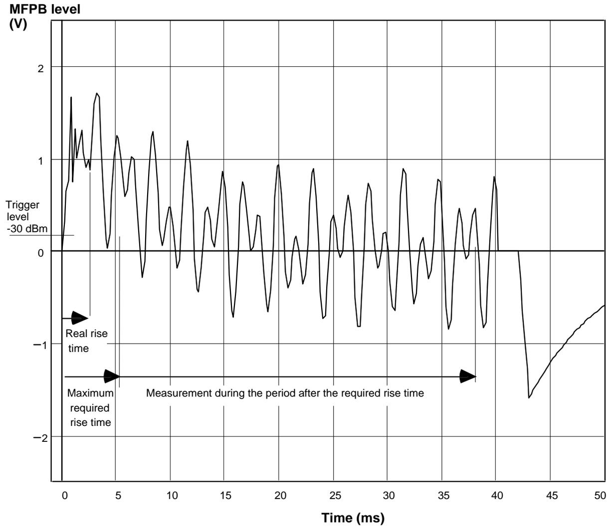
Figure D.17: MFPB transient timing, pragmatic measurement method
