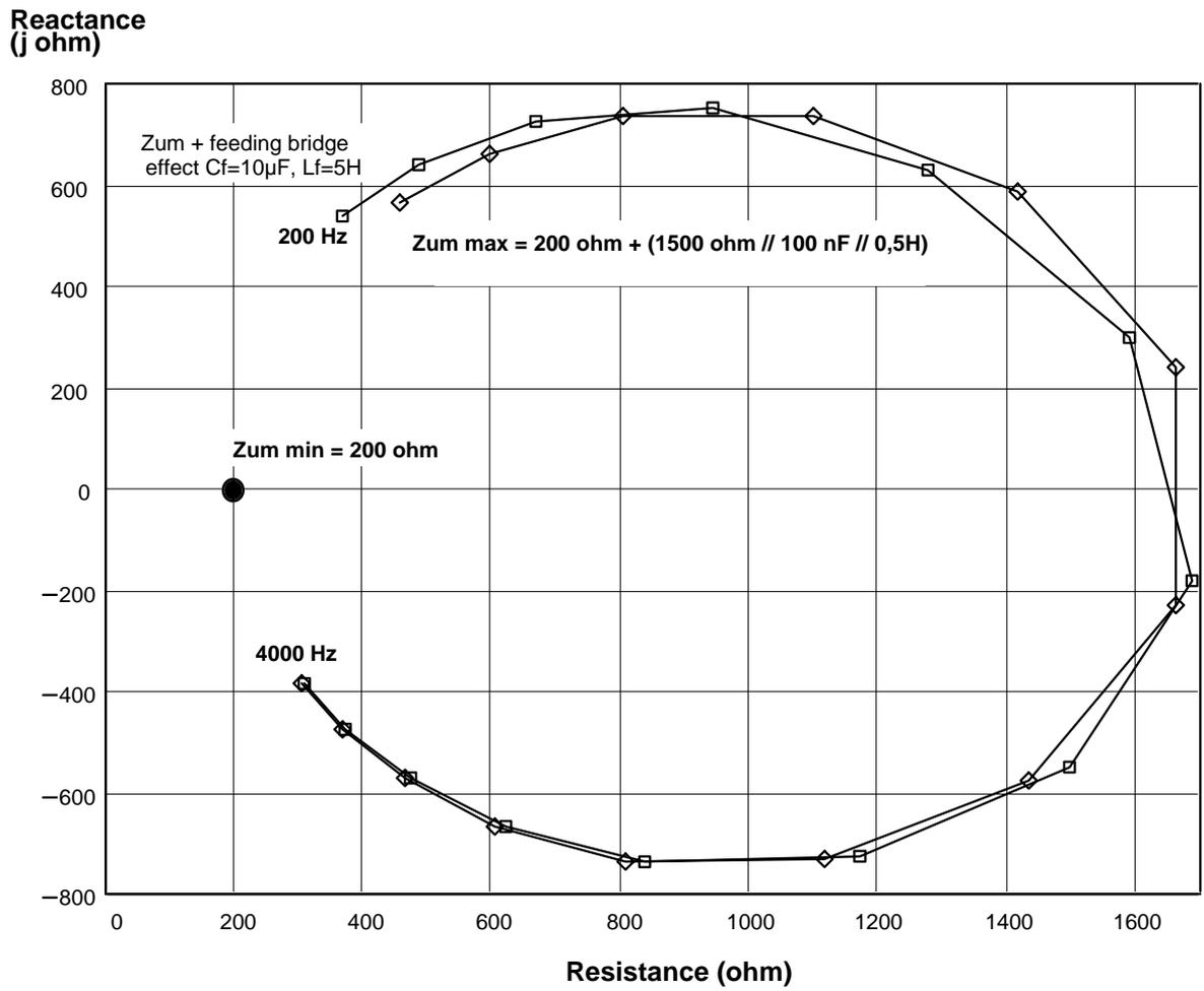
Figure D.5: Realistic external impedances (Zum min and Zum max) for the systematic effects study
