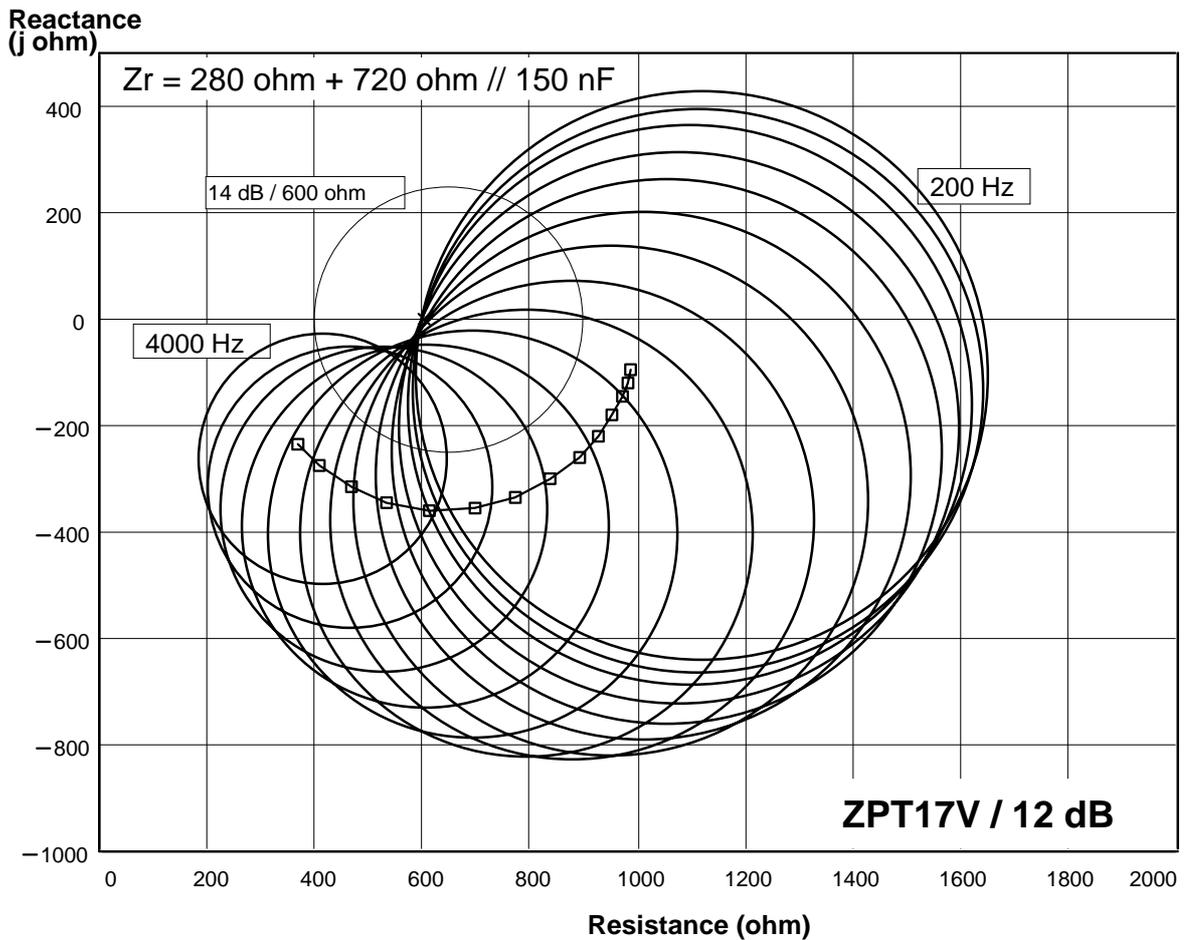
Values of the reference impedance and return loss limits for ZPT17V 12dB:
