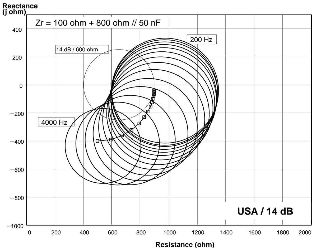
Values of the reference impedance and return loss limits for USA:
