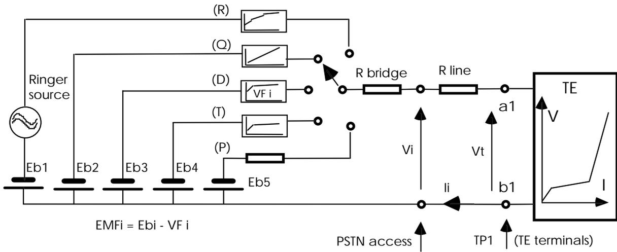
Figure A.3: PSTN interfaces and feeding conditions in the various call progress phases
