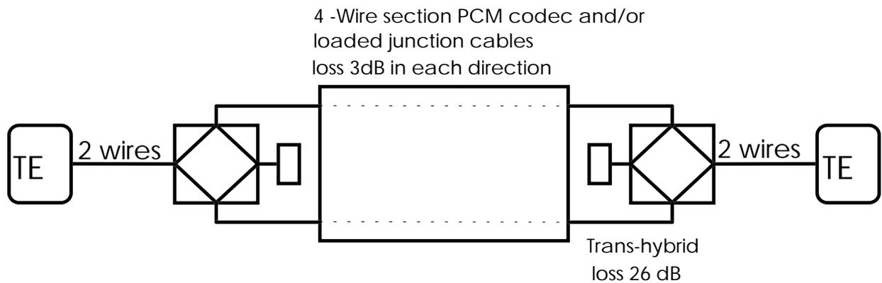
**Figure B.1: Basic telecommunication interconnection for echo consideration**
