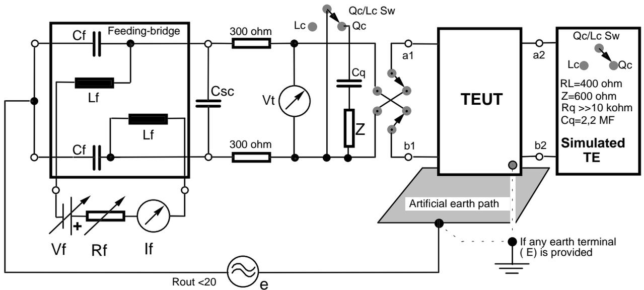
Figure D.15: Degree of unbalance about earth test arrangement for two-ports TE (LCL)
