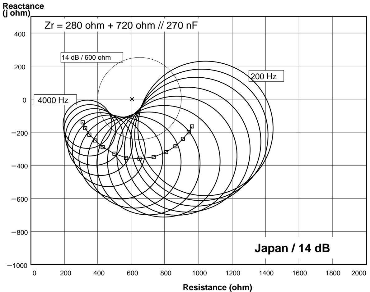
Values of the reference impedance and return loss limits for Japan:
