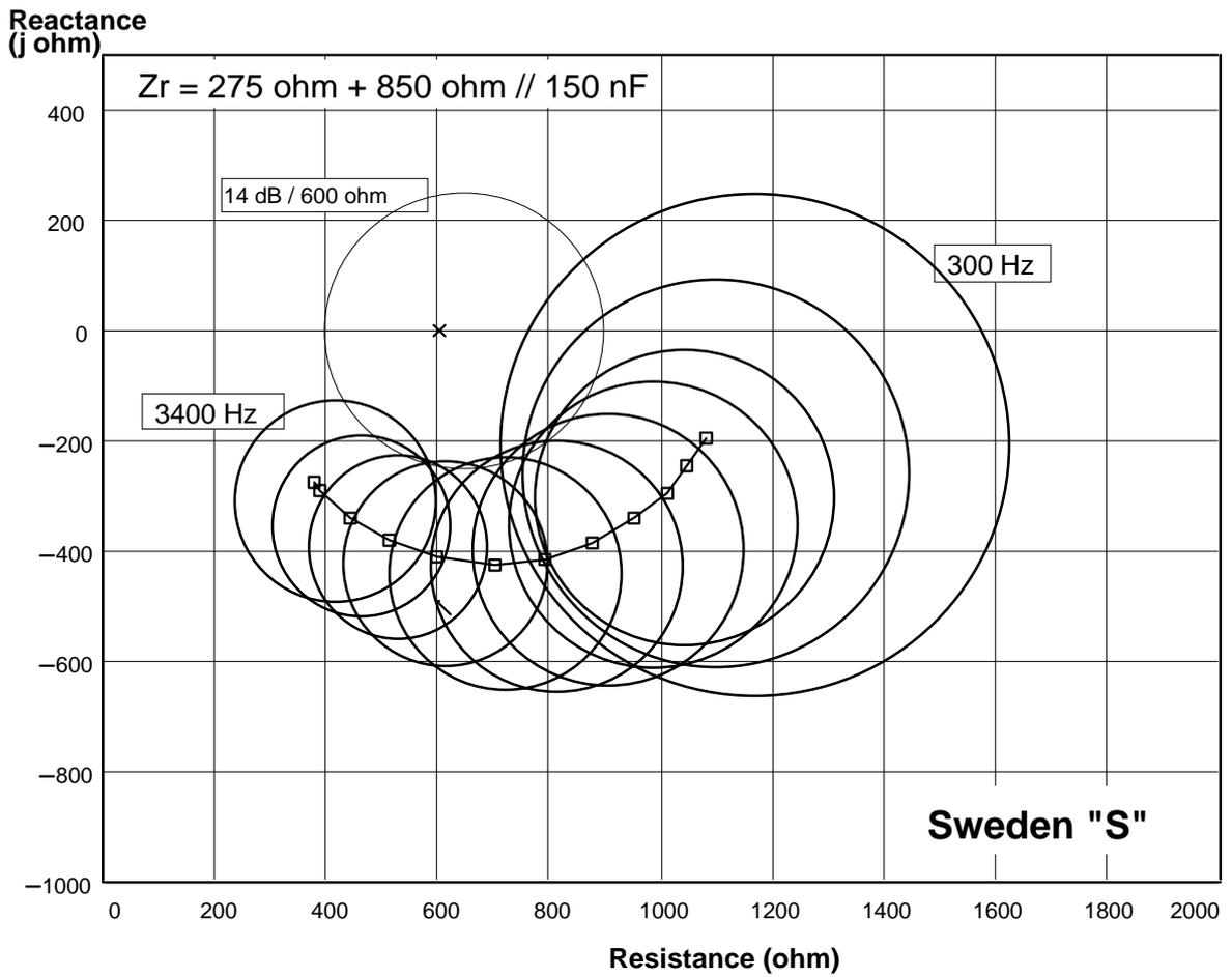
Values of the reference impedance and return loss limits for Sweden "S":
