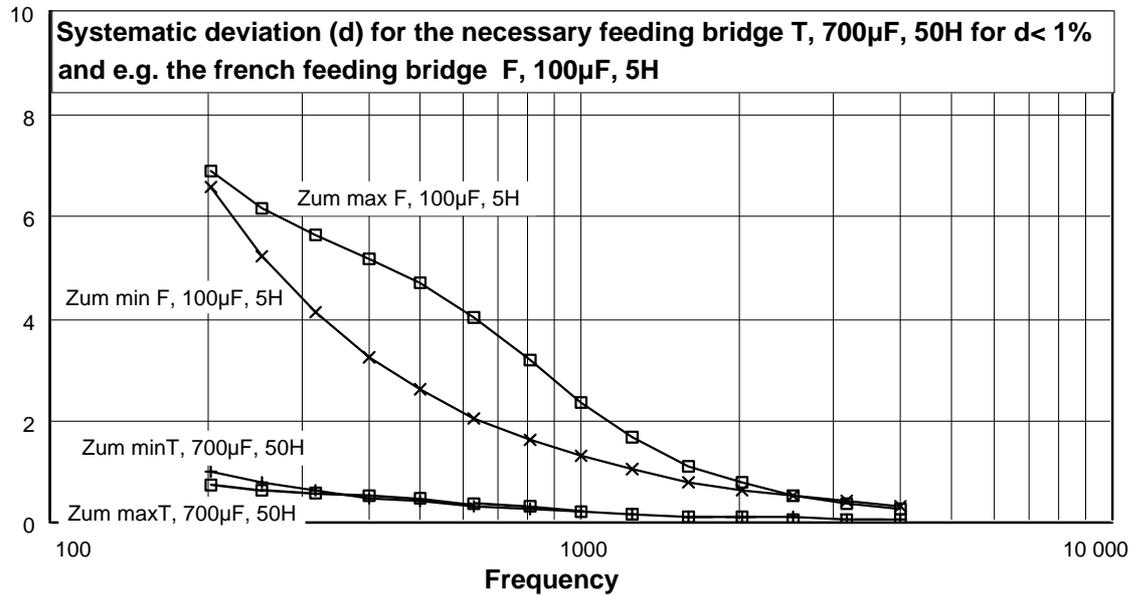
**Figure D.2: Determination of the feeding bridge characteristic to limit the systematic deviation at 1 % and the related systematic deviation**
