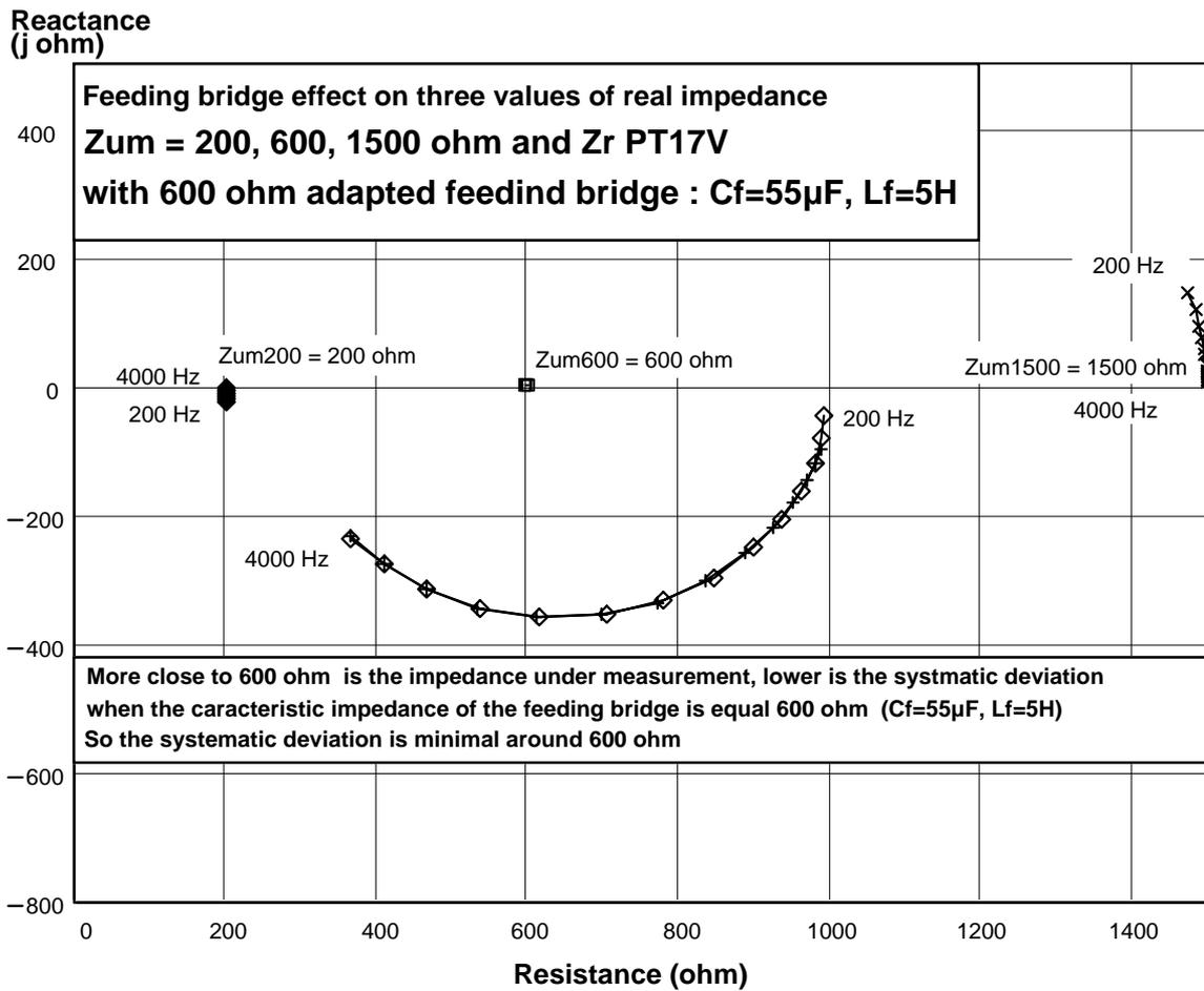
Figure D.7: Systematic deviation reduction around 600 ohm by the use of adapted feeding bridge
