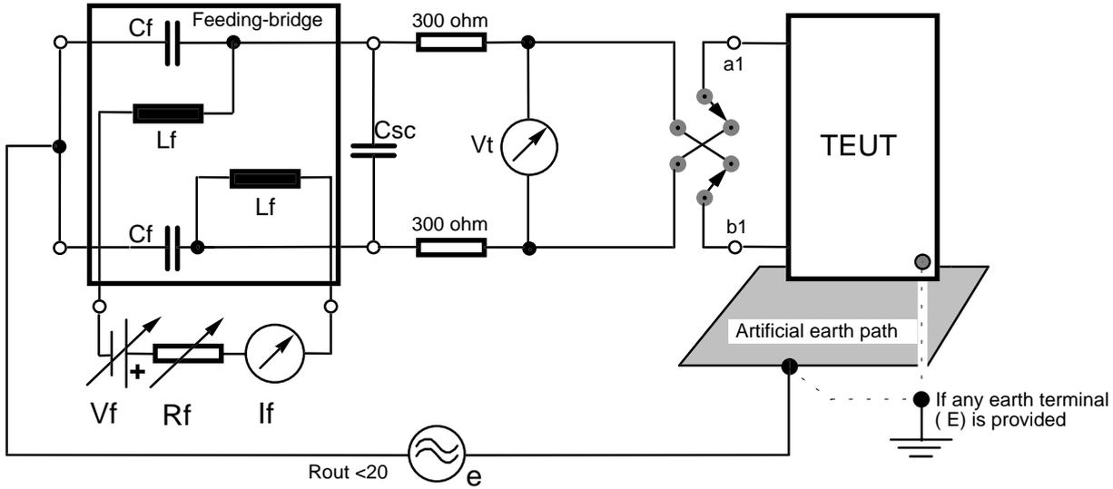
Figure D.14: Degree of unbalance about earth test arrangement for one-port TE (LCL)
