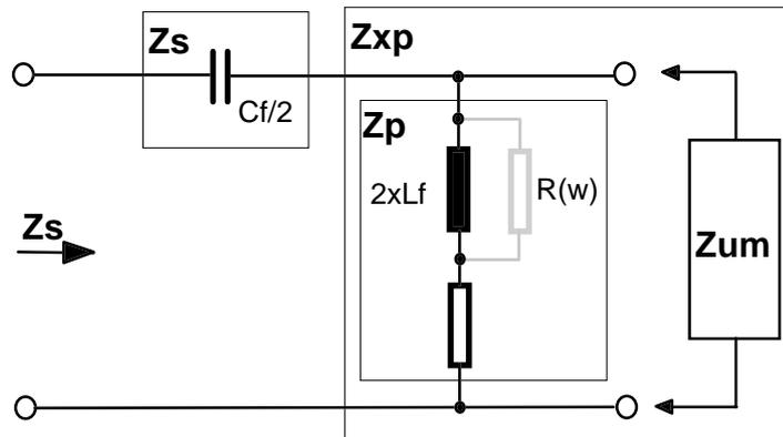
Figure D.11: Feeding bridge equivalent circuit
