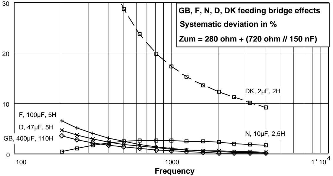
Figure D.1: GB, F, N, D, DK feeding bridge effect on the impedance ( $Z_{rPT17V}$ ) measurement and related systematic deviation
