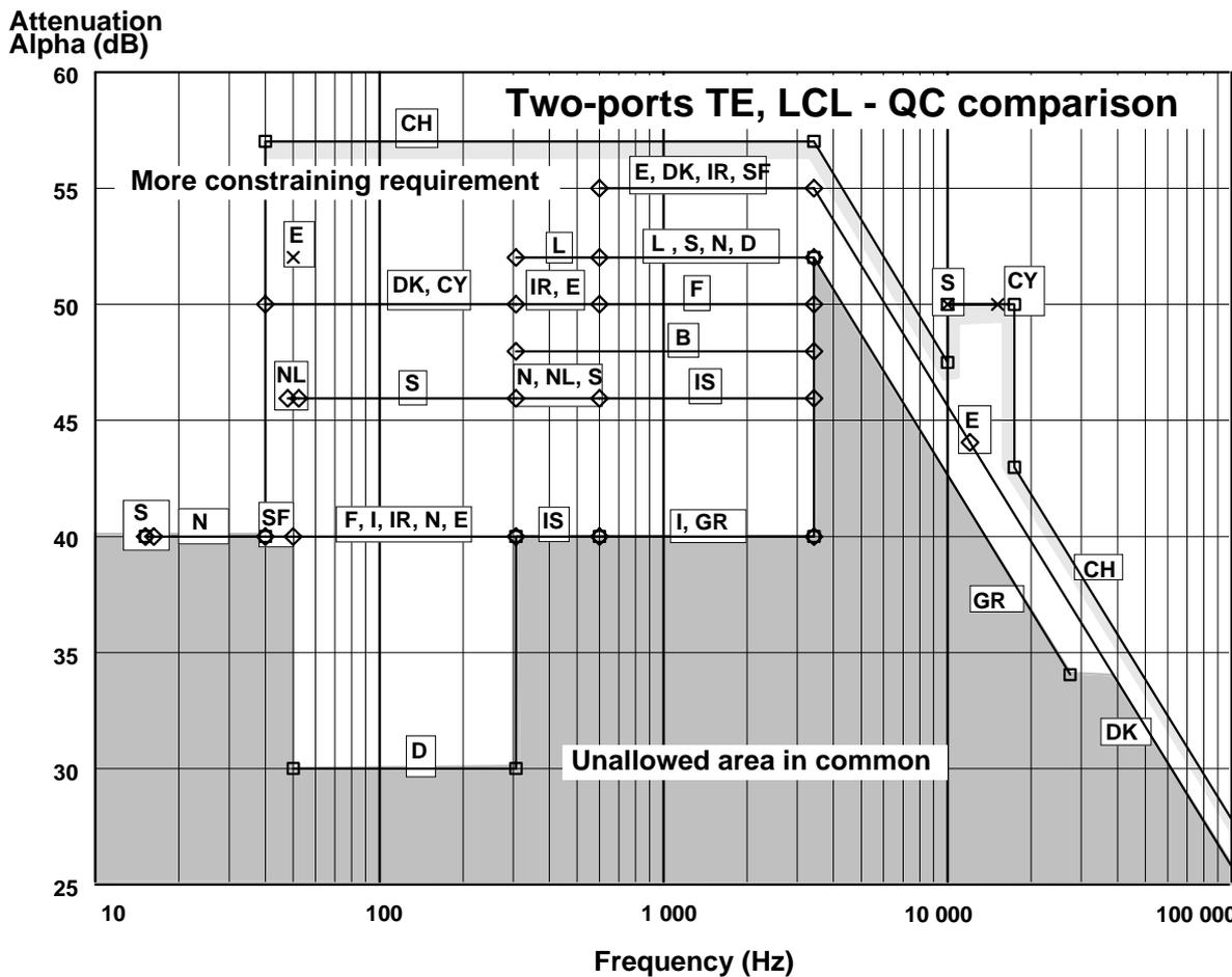
Figure C.2: Comparison of the attenuation value for all countries for the degree of unbalance about earth, case of LCL in loop condition (LC) for one port TE
