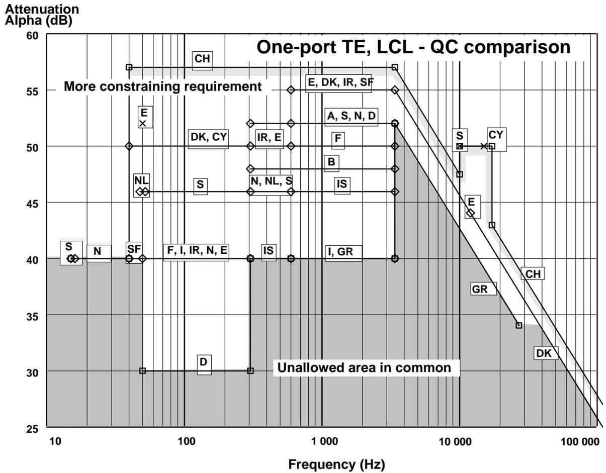
Figure C.1: Comparison of the attenuation value for all countries for the degree of unbalance about earth, case of LCL in quiescent condition (QC) for one port TE
