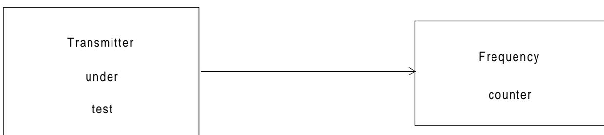
Figure 13: Frequency error measurement configuration
