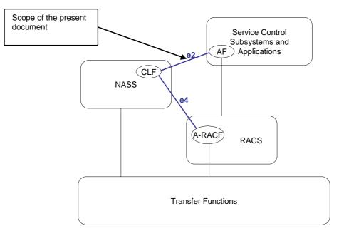
Figure A.1: NASS external interfaces
