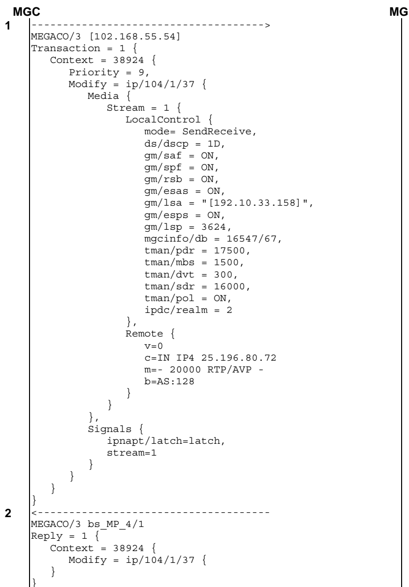
Figure 9: H.248 Message Sequence Example - Session Establishment Update - Remote Addr and Port Known, Through Connect and Latch
