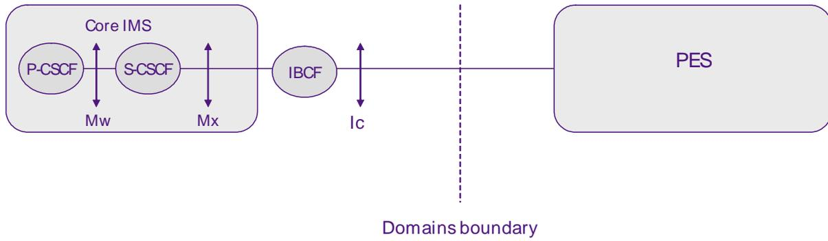
**Figure B.6: Interconnection between an IMS and a PES**
