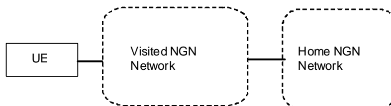
Figure 6.1: Functional network roles in TISPAN NGN
