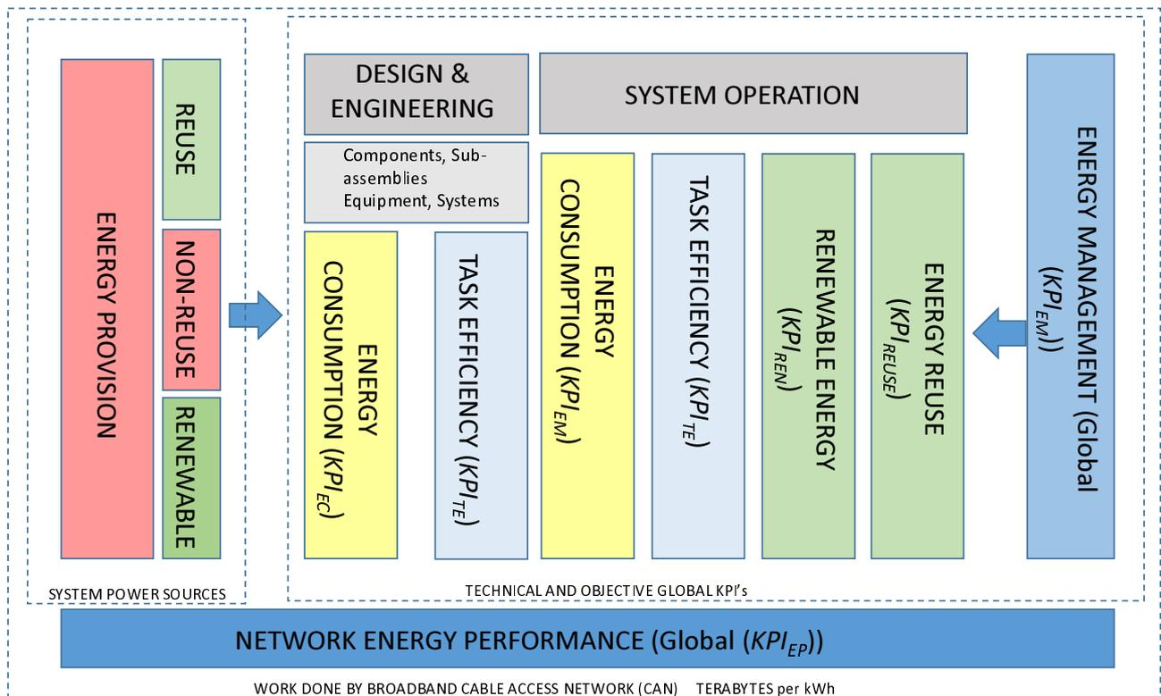
**Figure 6: Inter-relationship between technical, objective and global KPIs**
