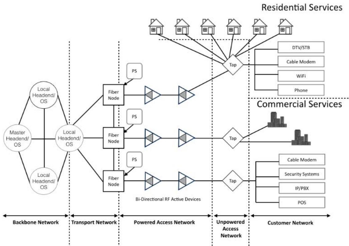
**Figure 3: Schematic of HFC 'fixed' cable network infrastructures**
