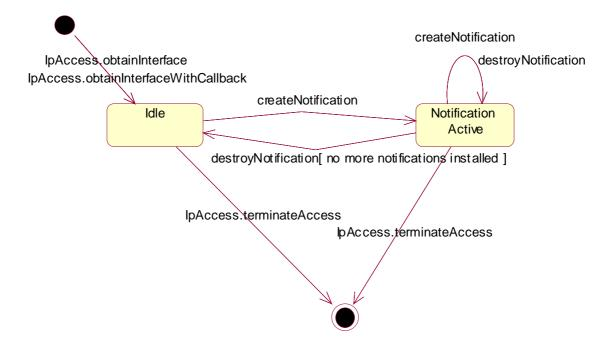
Figure 16: State Transition Diagram for IpEventNotification
