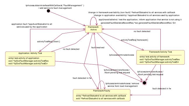
Figure 32: State Transition Diagram for IpFwFaultManager
