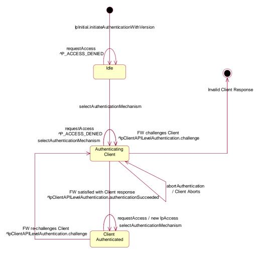
Figure 4: STD for IpAPILevelAuthentication: Framework authenticates Client using initiateAuthenticationWithVersion() and challenge() method combination
