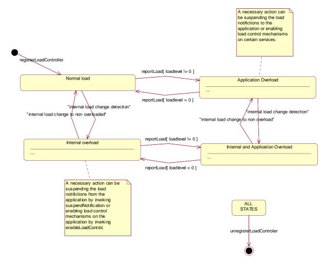
Figure 13: State Transition Diagram for LoadManagerInternal
