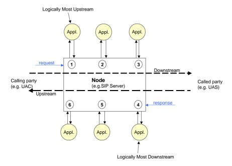
Figure 1: Cascaded Chain Model
