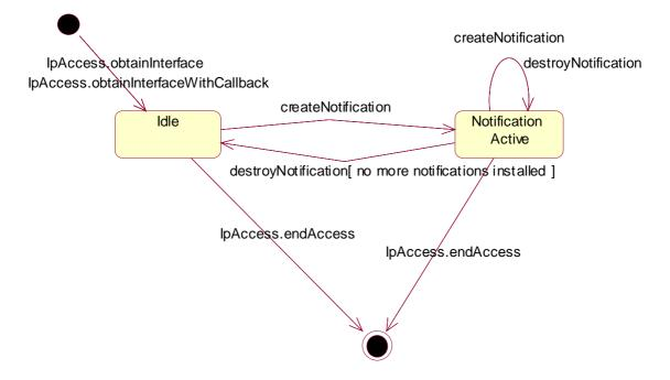
Figure 18: State Transition Diagram for IpEventNotification
