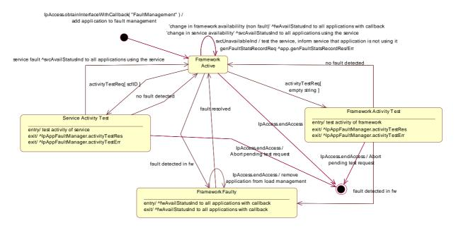
Figure 17: State Transition Diagram for IpFaultManager
