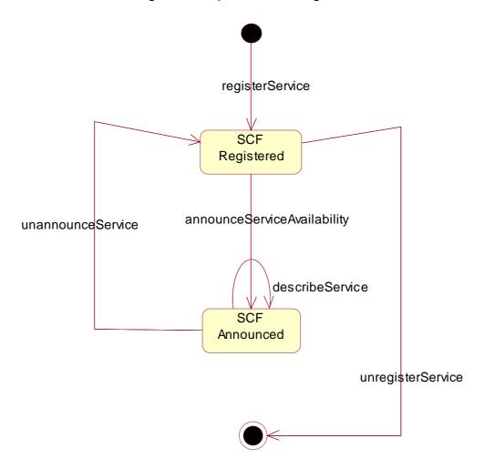
Figure 32: State Transition Diagram for IpFwServiceRegistration
