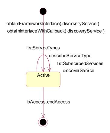
Figure 13: State Transition Diagram for IpServiceDiscovery
