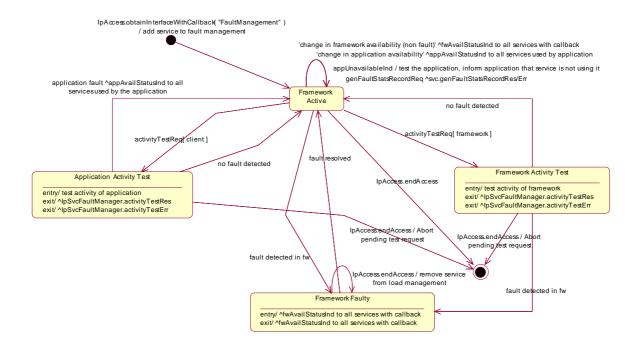
Figure 34: State Transition Diagram for IpFwFaultManager
