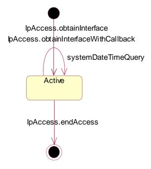
Figure 16: State Transition Diagram for IpOAM
