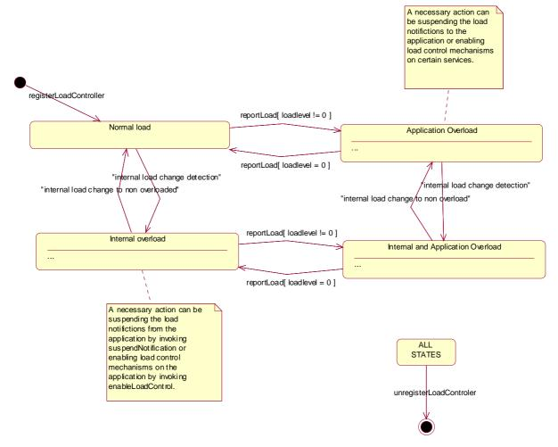
Figure 15: State Transition Diagram for LoadManagerInternal
