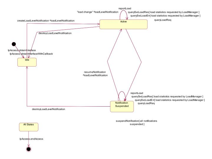
Figure 14: State Transition Diagram for IpLoadManager
