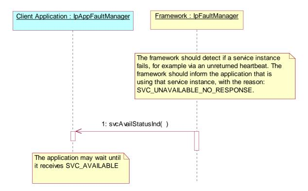
1: The framework informs the client application that is using the service instance that the service is unavailable. The client application may wait to receive a new call to the svcAvailStatusInd with the reason SVC\_AVAILABLE when the Service has become available again. The different Unavailability reasons used by the Framework (TpSvcAvailStatusReason) guides the client application developers to make the decision.
