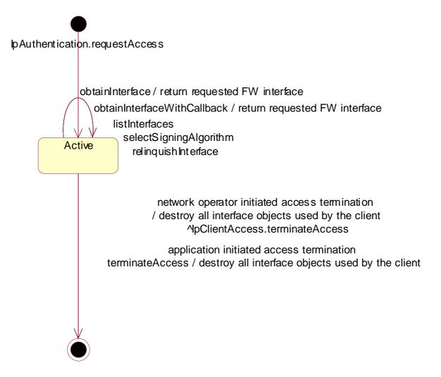
Figure 7: State Transition Diagram for IpAccess
