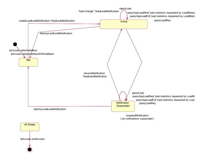
Figure 33: State Transition Diagram for IpFwLoadManager
