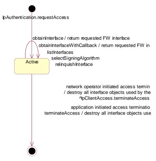
Figure 7: State Transition Diagram for IpAccess
