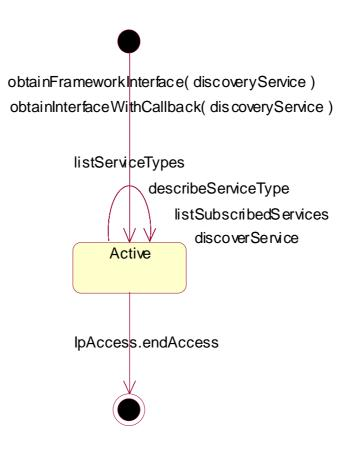
Figure 13: State Transition Diagram for IpServiceDiscovery
