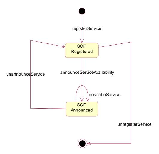
Figure 32: State Transition Diagram for IpFwServiceRegistration
