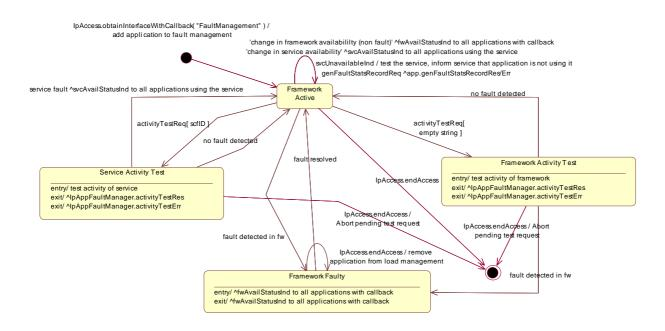
Figure 17: State Transition Diagram for IpFaultManager
