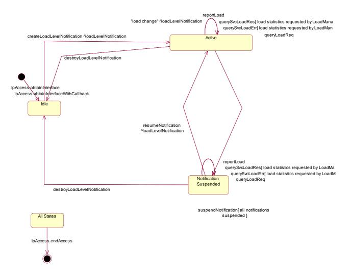
Figure 14: State Transition Diagram for lpLoadManager
