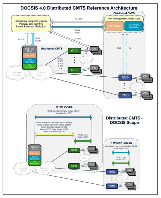
Figure 3: Distributed CMTS reference architecture
