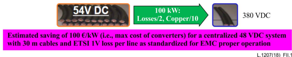
Figure C.1: Estimation of copper saving comparing -48 V and up to 400 VDC
