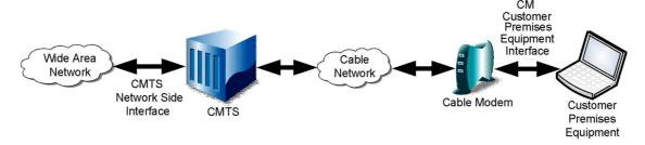
Figure 2: Transparent IP Traffic Through the Data-Over-Cable System
