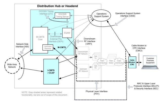
Figure 3: Data-over-Cable Reference Architecture
