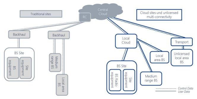
Figure 1: Network under test definition
