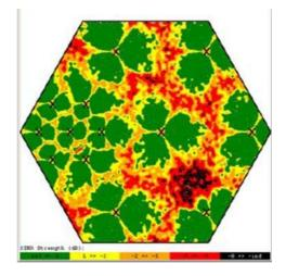
Figure 5: Typical SINR distribution of a mobile network
