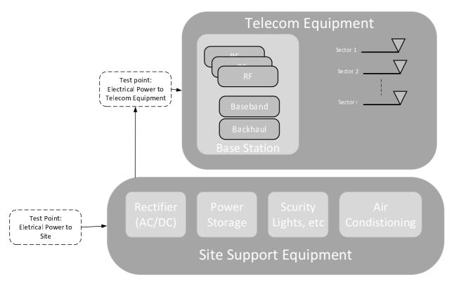
Figure 2: Layout of a typical site to determine the SEE metric
