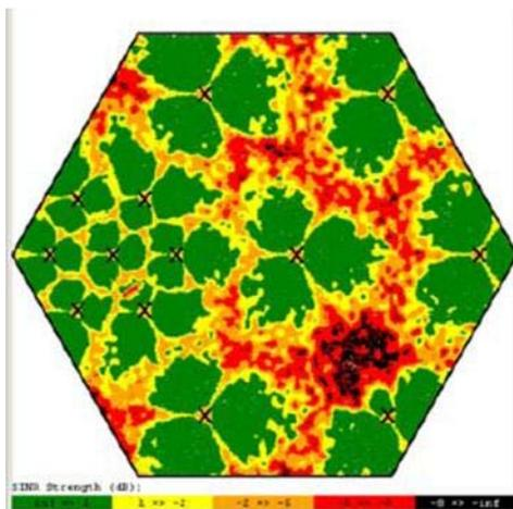
**Figure 2: Typical SINR distribution of a mobile network**
