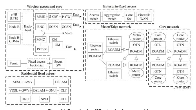
Figure I.1: Example of an ICT network reference model
