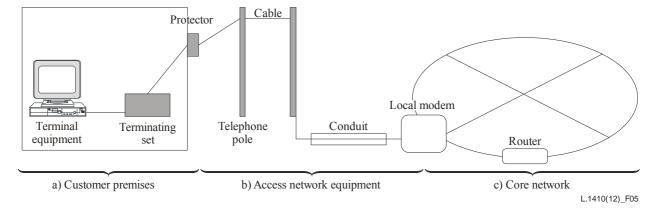
Figure 5: Fixed telecommunication network - simplified physical view
