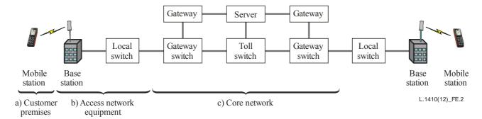
Figure I.2: Example of functions of wireless mobile telecommunication network
