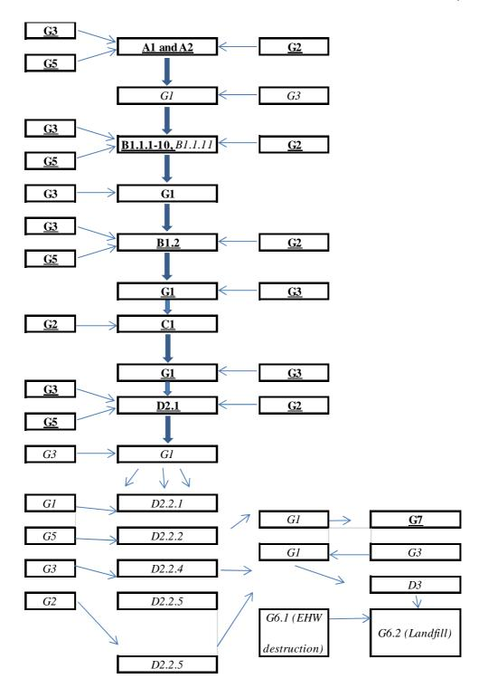
Figure L.2: The system boundary of the product system for LCA of the Mobile Phone showing connections with generic processes
