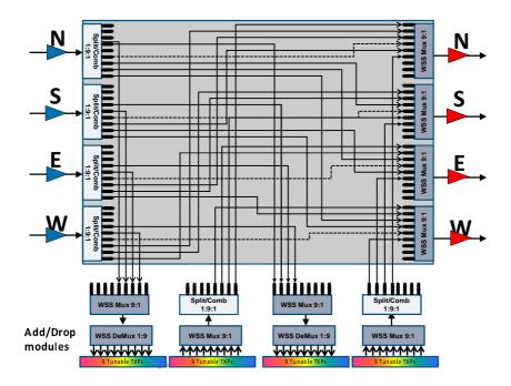
Figure A.4: ROADM WSS based schematic (System Configuration)
