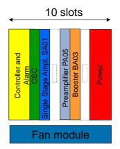
Figure A.3: Optical amplifier schematic (System Configuration from Manufacturer B)
