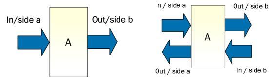
Figure 1: Schematic representation for Category A Transport equipment: unidirectional (on the left) or bidirectional (on the rigth)
