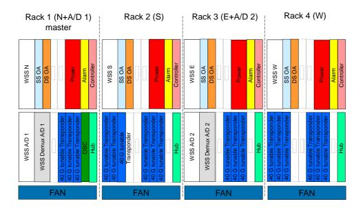
Figure A.5 represents the whole 4 degrees ROADM system on four 20 slots/two rows (shelves) racks.
