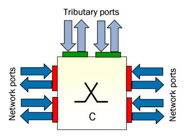
Figure 3: Schematic representation for Category C Transport equipment
