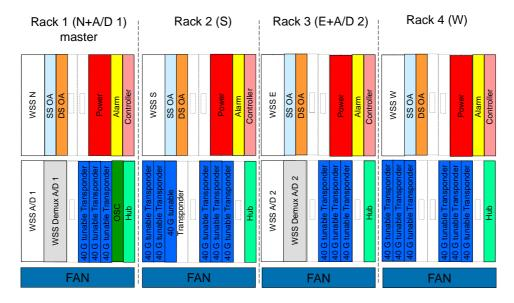
Figure A.5: ROADM WSS based schematic for whole 4 degrees system (System Configuration)
