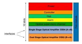
Figure A.2: Optical amplifier schematic (System Configuration from Manufacturer A)
