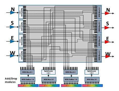
Figure A.4: ROADM WSS based schematic (System Configuration)
