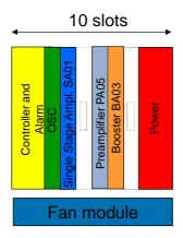
Figure A.3: Optical amplifier schematic (System Configuration from Manufacturer B)
