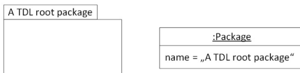
Figure 4: Concrete syntax (left) and model instance representation of a TDL root Package (right)
