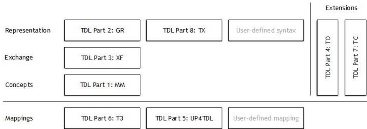
**Figure 4.1: The TDL standards and their positioning**
