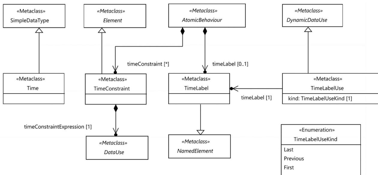
**Figure 7.1: Time, time label and time constraint**
