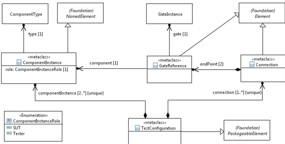
Figure 8.2: Test configuration
