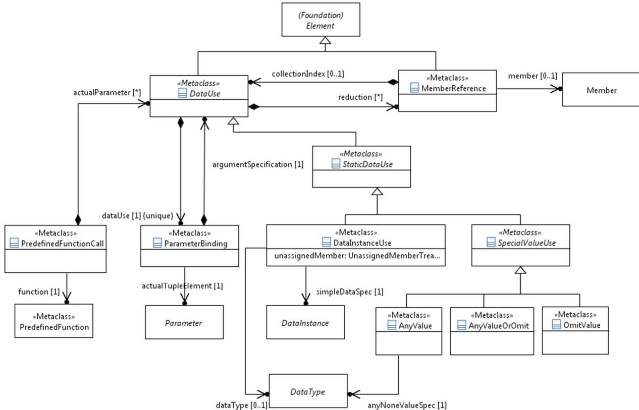
Figure 6.7: Data use concepts and static data use
