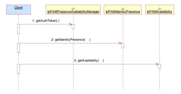
1: For any unique entity requesting the operation, the authenticated client of the OSA PAM service, requests for an authentication token using the getAuthToken() method in the PresenceAvailability Manager interface.
