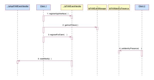
1: The client uses the registerAppInterface() method to register its notification interface. The getAuthToken() can be null since the client is doing this registration on its own behalf. The client gets a unique client ID back.
