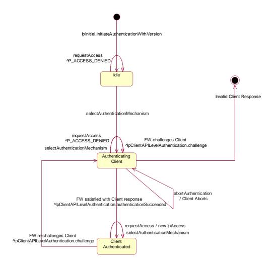
Figure 6: STD for IpAPILevelAuthentication: Framework authenticates Client using initiateAuthenticationWithVersion() and challenge() method combination
