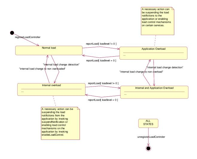
Figure 15: State Transition Diagram for LoadManagerInternal
