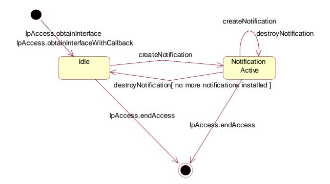
Figure 13: State Transition Diagram for IpEventNotification
