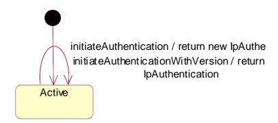
Figure 2: State Transition Diagram for IpInitial
