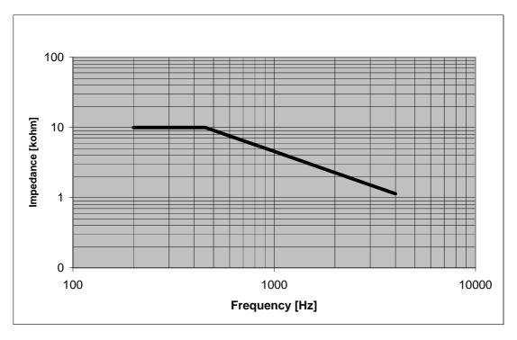
Figure 4: Minimum impedance in the voice band
