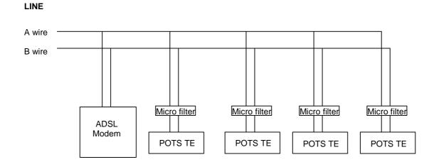
Figure 2: Scenario 2: installation using distributed filters
