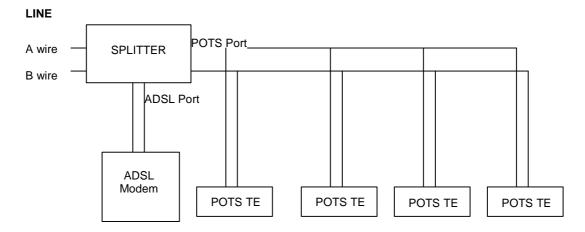
Figure 1: Scenario 1: installation using a central splitter
