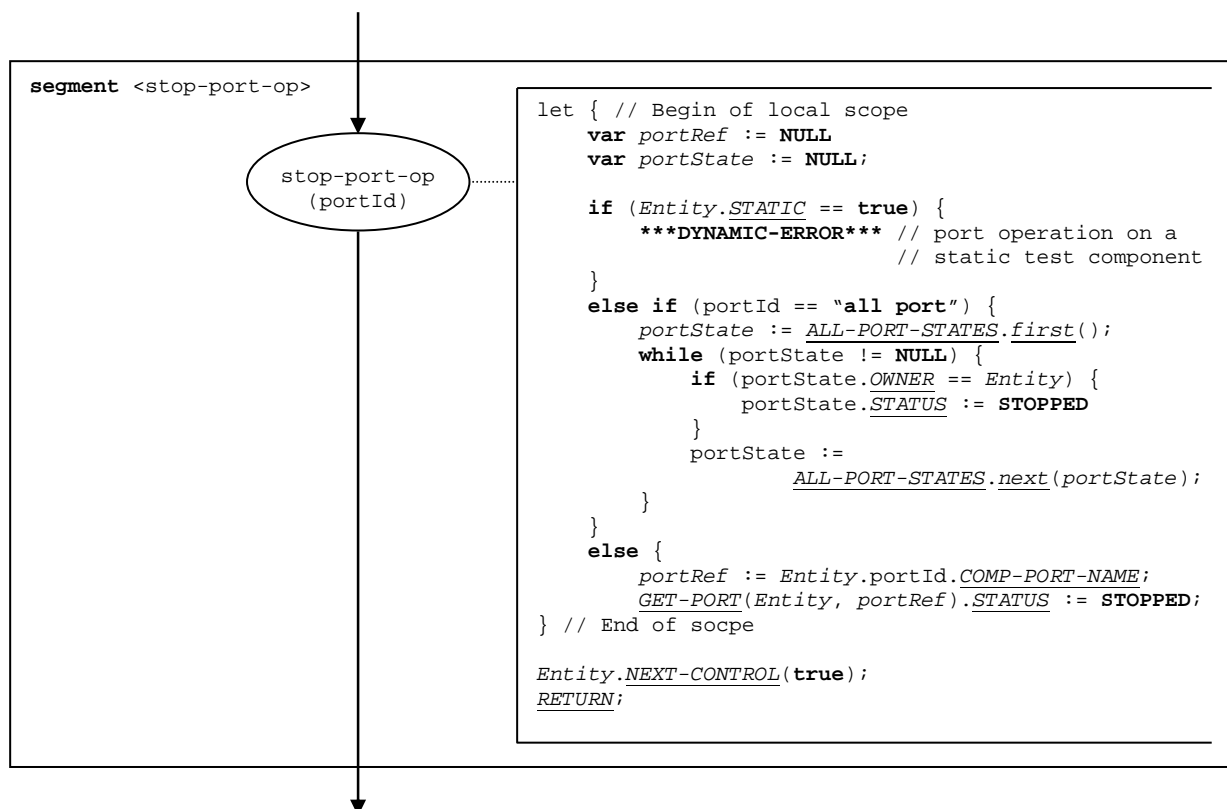
Figure 129 of ETSI ES 201 873-4 [2]: Flow graph segment <stop-port-op>
