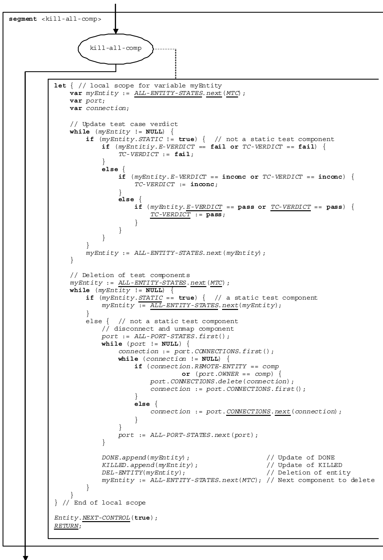
Figure 90d of ES 201 873-4 [2]: Flow graph segment &lt;stop-all-comp&gt;
