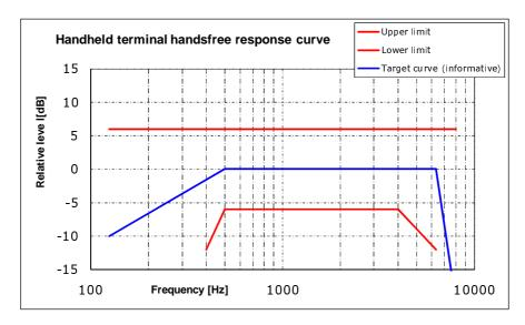
Figure 15: Receive frequency response mask for Hand-held HFT
