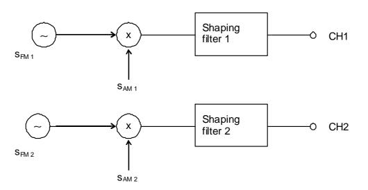
Figure 17a: Measurement signals
