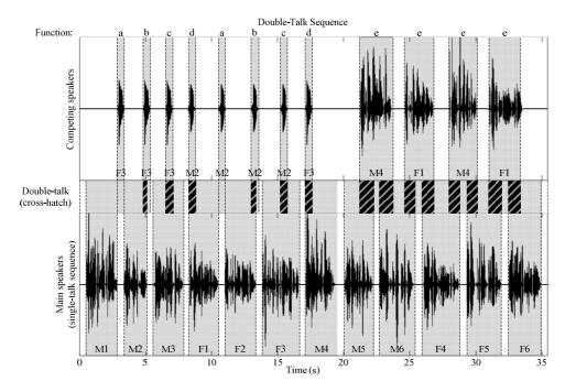
Figure 17: Double Talk Test Sequence with overlapping speech sequences in send and receive direction
