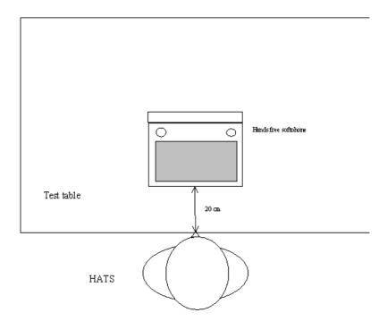
Figure 6: Configuration of softphone relative to the HATS top sight
