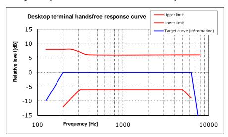
Figure 14: Receive frequency mask for Desktop HFT
