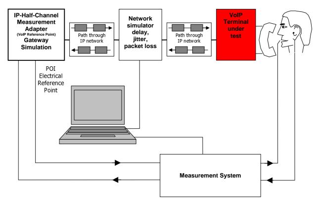
Figure 1: Half channel terminal measurement
