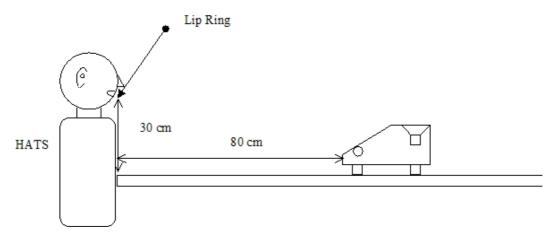
Figure 9: Configuration of group audio terminal relative to the HATS side view
