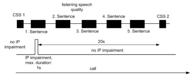
Figure 21: Test Sequence to measure quality of Jitter buffer adjustment (with 1 of 12 sentences)
