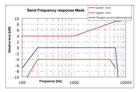
Figure 13: Send sensitivity/frequency mask for HFT
