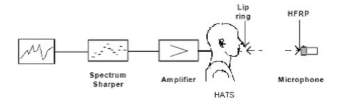
Figure 11: Calibration at HFRP (with d<sub>HFS</sub> = 50 cm)
