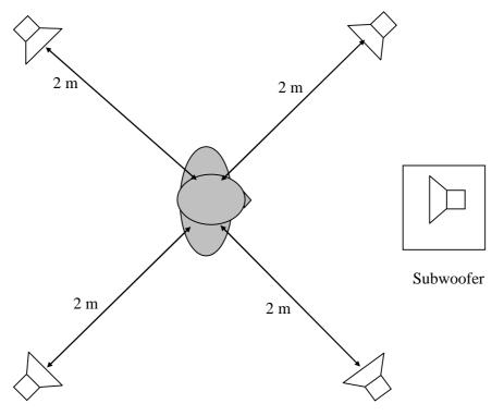
Figure 12: Loudspeaker arrangement for background noise simulation
