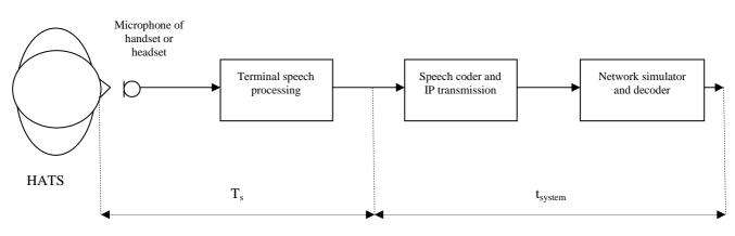
Figure 8: Different blocks contributing to the delay in send direction
