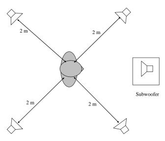
Figure 2: Loudspeaker arrangement for background noise simulation
