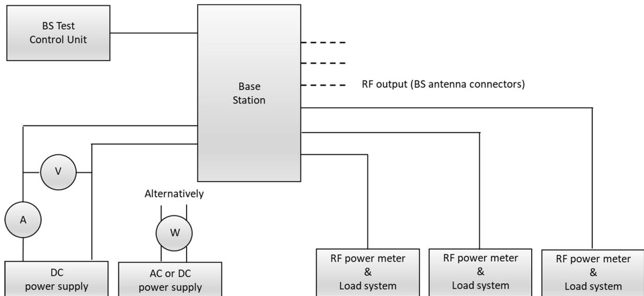
NOTE: BS as defined in Figure 1 (integrated BS) or Figure 2 (distributed BS). AC supply to be used for BS with built in AC power supply, otherwise default DC supply voltage as specified in clause 5.2.
