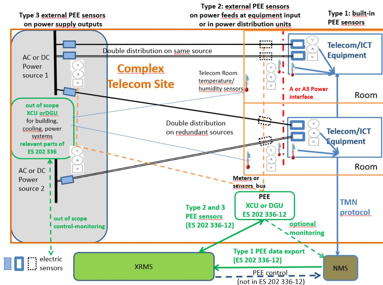
**Figure 3: Example of cohabitation of ICT equipment internal and external power/energy/environment measurement acquisition in a site considering 3 cases of implementations (power frame measurement, input junction box measurements, built-in measurements)**
