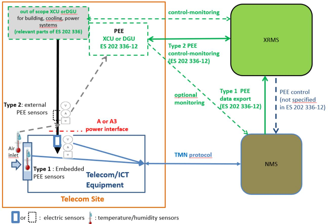
**Figure 2: Example of possible implementation in a simple Telecom site (e.g. a radio mobile site with ICT/Telecom connected to an OSS/NMS)**
