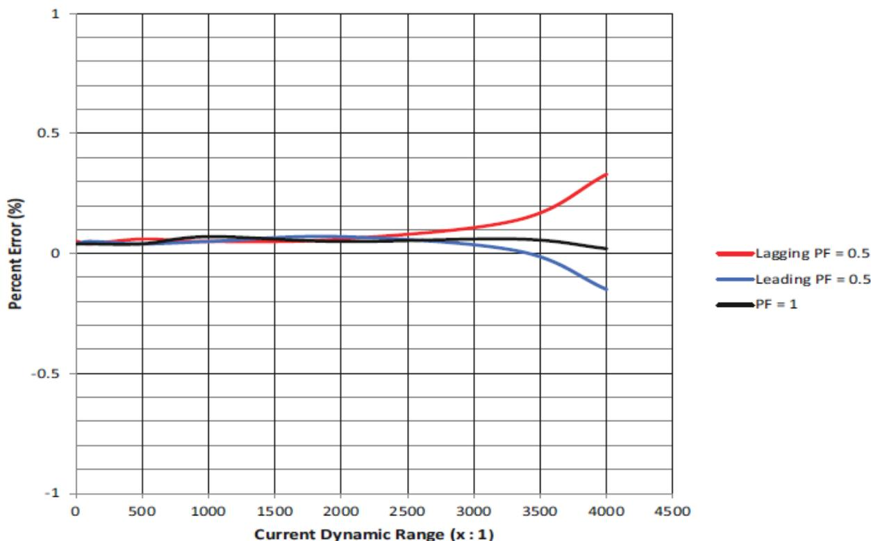
**Figure F.2: Example of electric AC energy metering accuracy**
