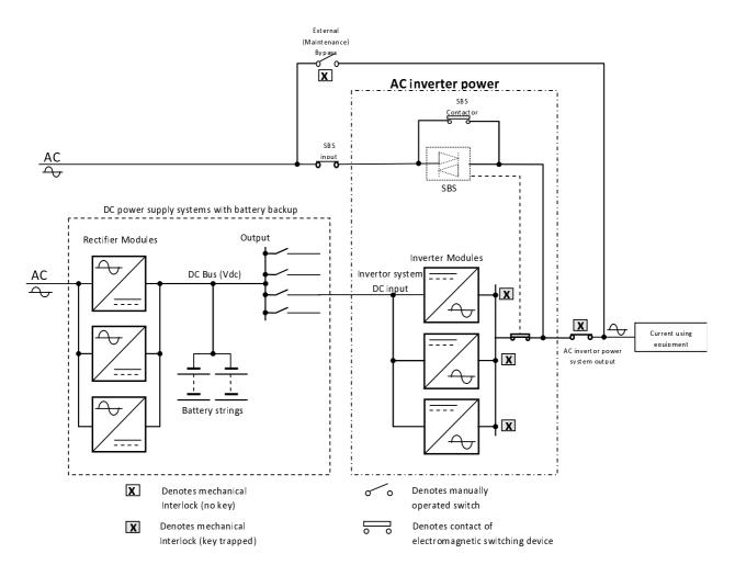
NOTE: Part of figure 1, with DC power supply system with battery backup is shown for better understanding and is not subject of the present document.
